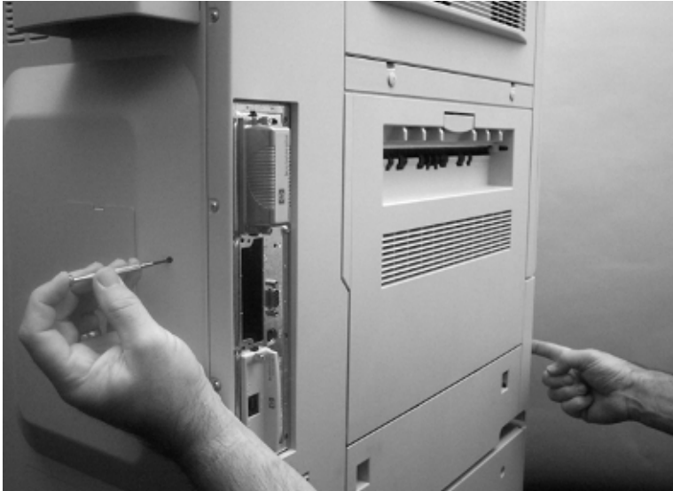
Figure 122. Prepare to print a laser/scanner adjustment page
