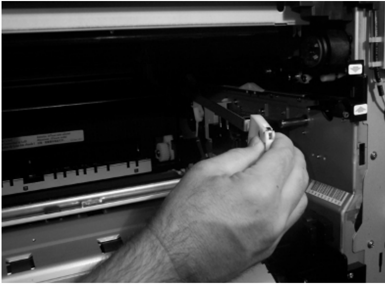
Figure 206. Remove the right back ITB lifting link
