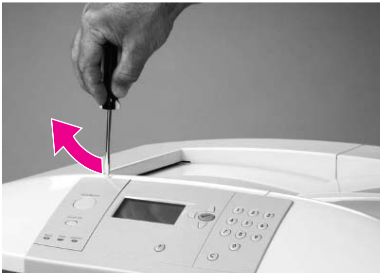
Figure 82. Remove the control panel overlay
