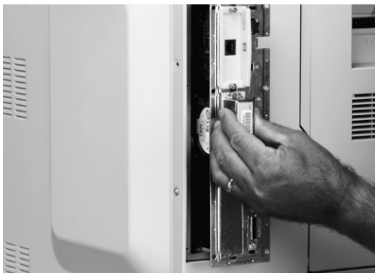
Figure 230. Remove the formatter PCB
