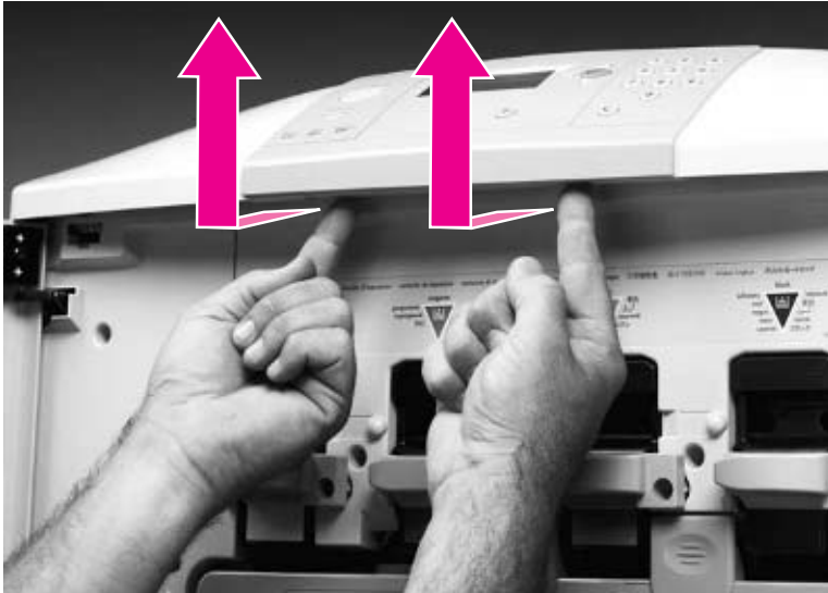
Figure 83. Release the control panel
