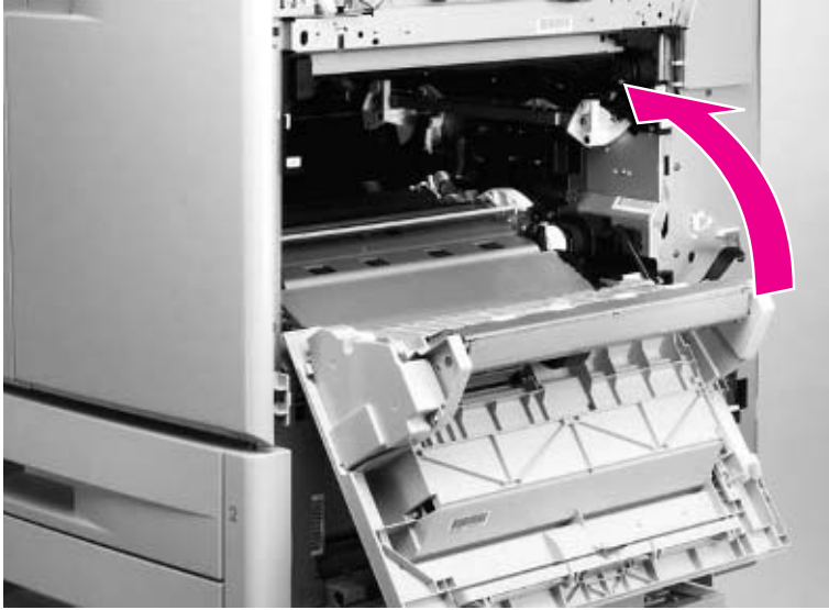
Figure 185. Gain access to the ITB door mounting screws
