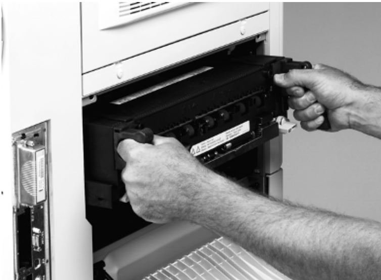
Figure 158. Remove the fuser
