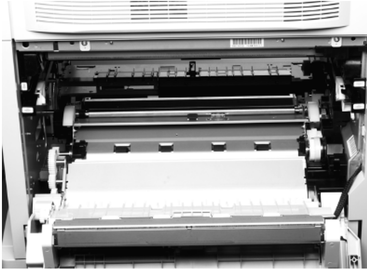
Figure 178. Remove the T2 assembly
