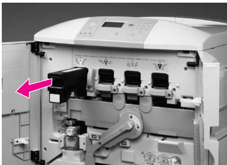
Figure 72. Remove the toner cartridge
