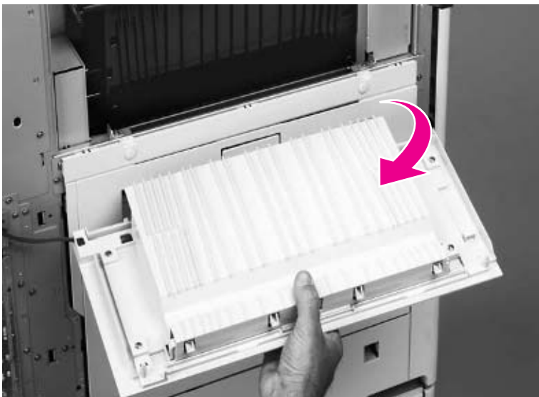
Figure 149. Remove the paper path access door
