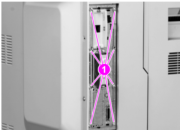
Figure 229. Remove the formatter PCB mounting screws
