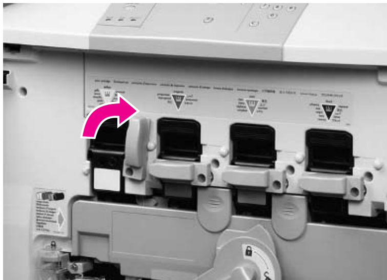
Figure 71. Rotate the toner cartridge lever
