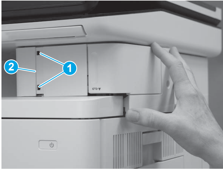
Figure 1-345 Install two tabs
