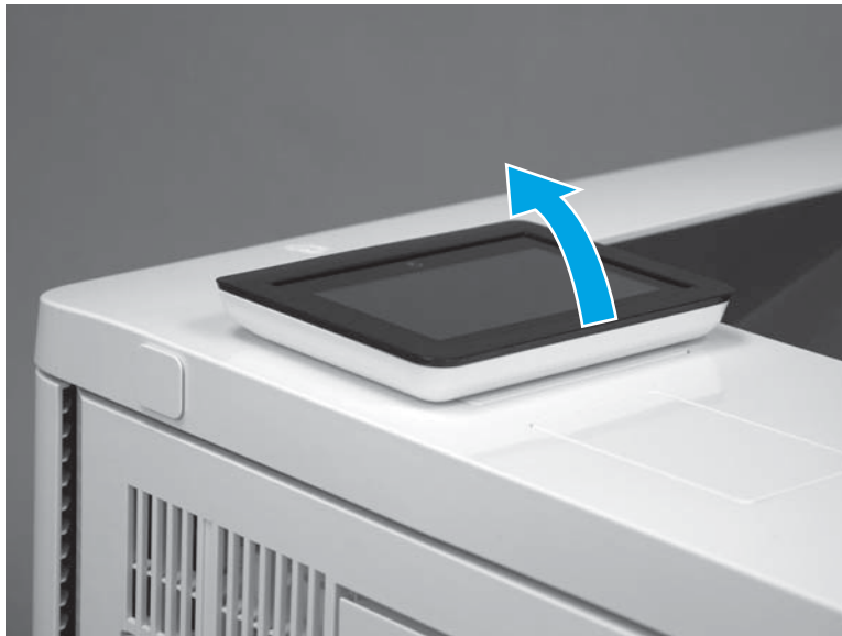
Figure 1-2640 Tilt the control panel up
