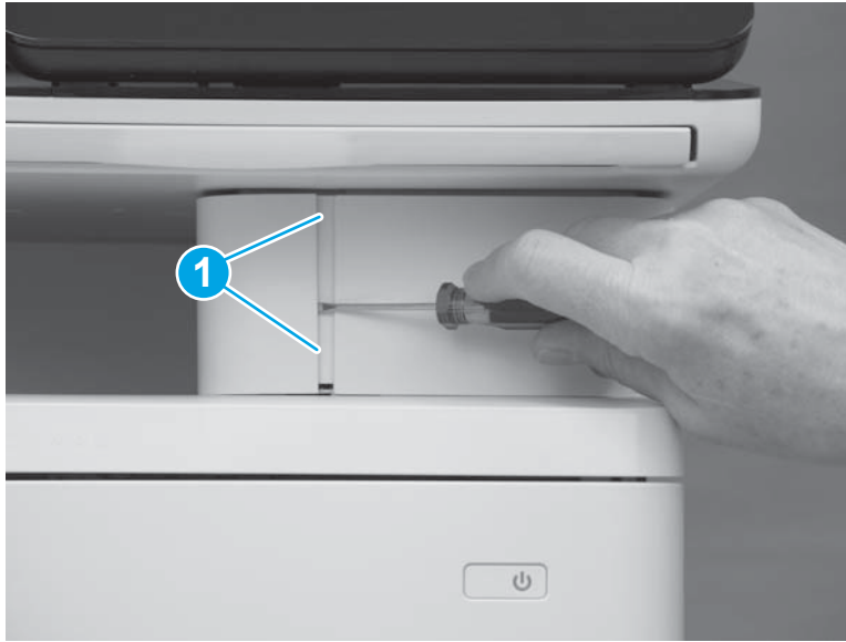
Figure 1-3406 Release two tabs
