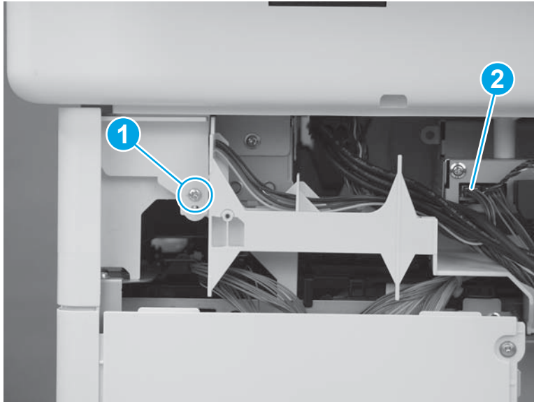
Figure 1-3211 Remove one screw and connector
