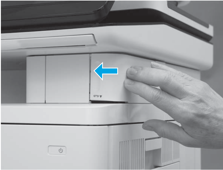
Figure 1-4227 Install the cover assembly
