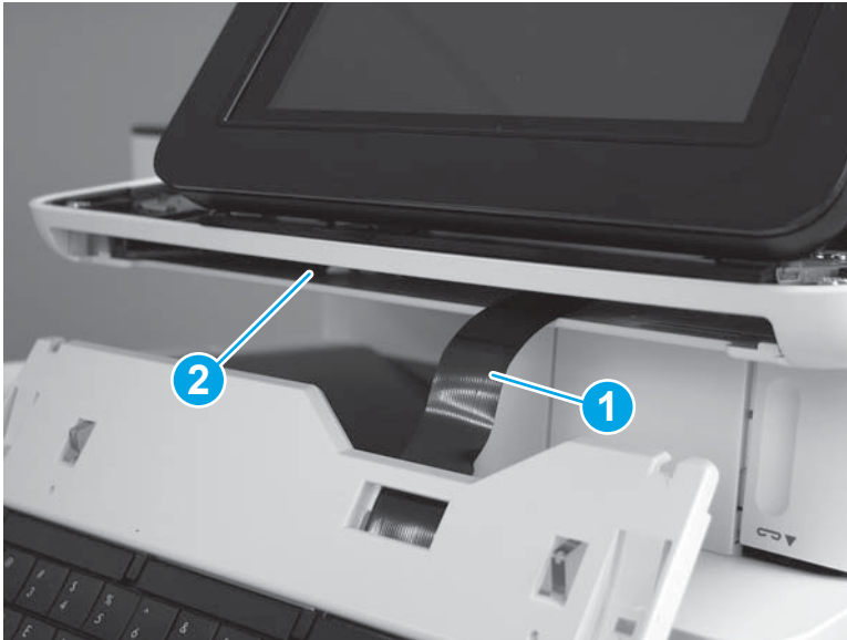
Figure 1-4953 Install the flat cable through the slot
