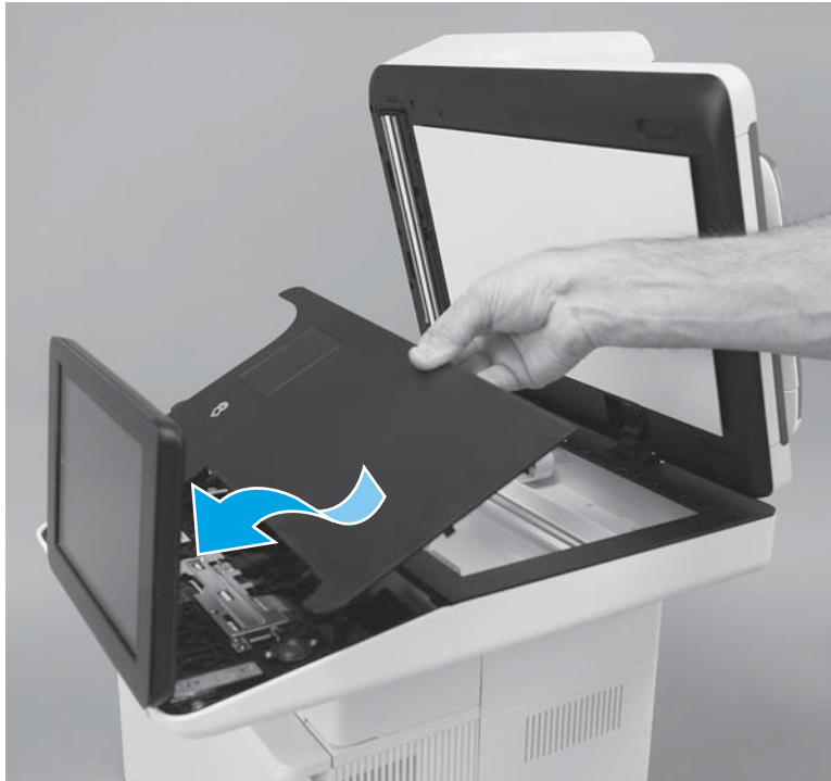
Figure 1-1060 Position the control-panel cover on the printer
