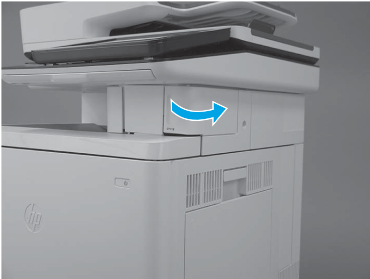
Figure 1-1204 Open the stapler door
