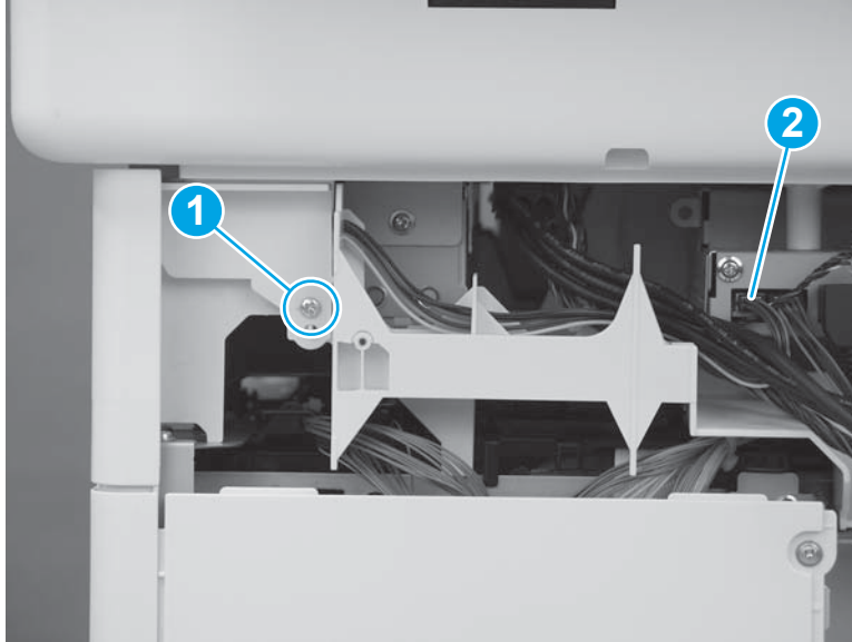
Figure 1-4730 Install one screw and connector
