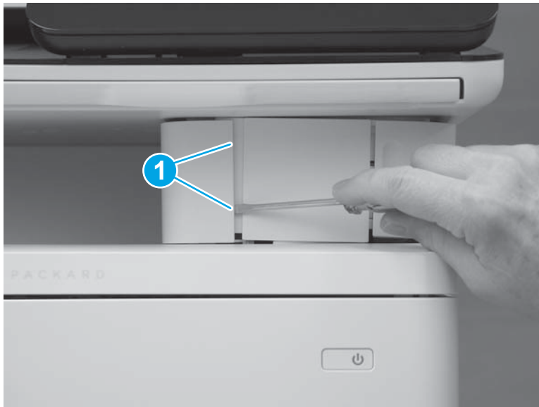
Figure 1-4573 Release two tabs
