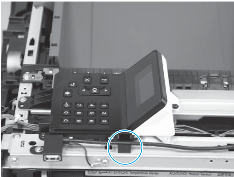
Figure 1-953 Place one cable in the guide
