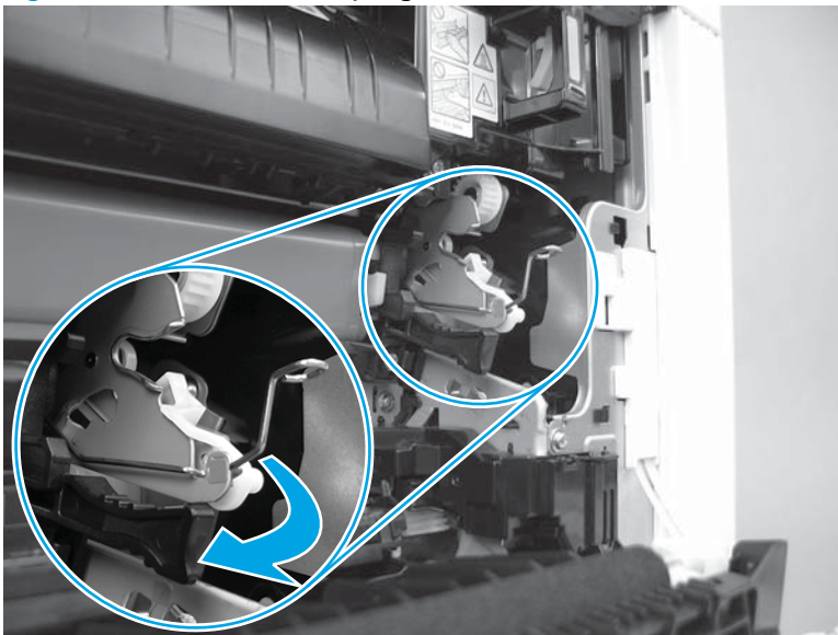
Figure 1-4510 Remove the spring from the holder
