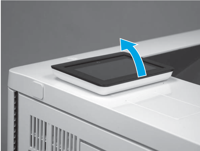
Figure 1-1813 Tilt the control panel up
