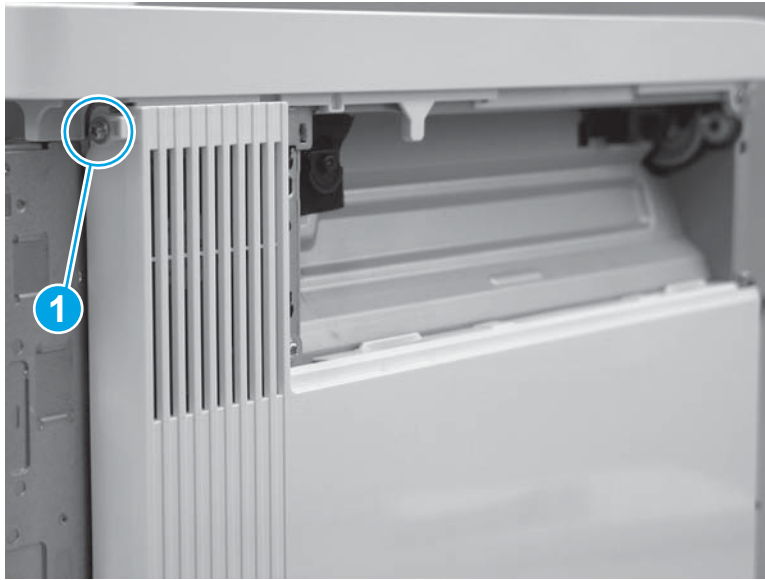
Figure 1-691 Install one screw
