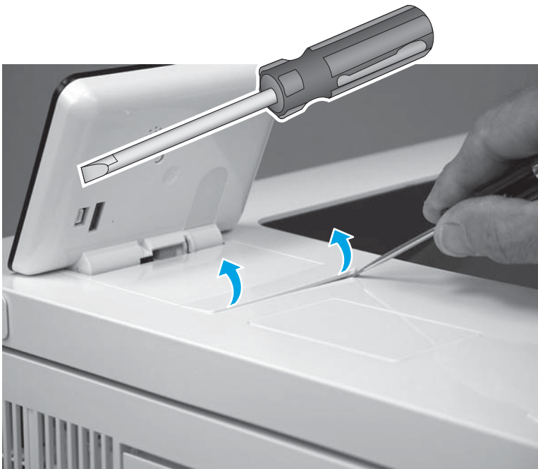
Figure 1-1814 Release the control-panel screws cover tabs
