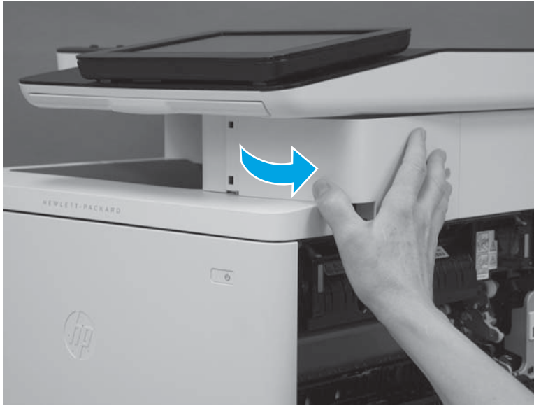
Figure 1-1282 Rotate the cover
