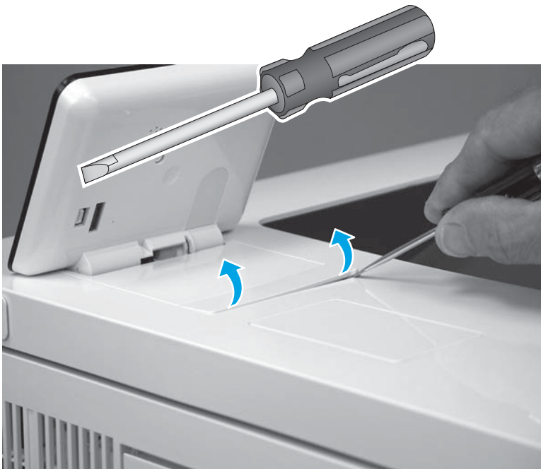
Figure 1-3811 Release the control-panel screws cover tabs
