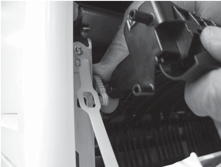
Figure 1-996 Disengage the blue arm and pin
