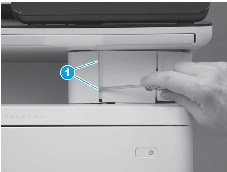
Figure 1-1844 Release two tabs
