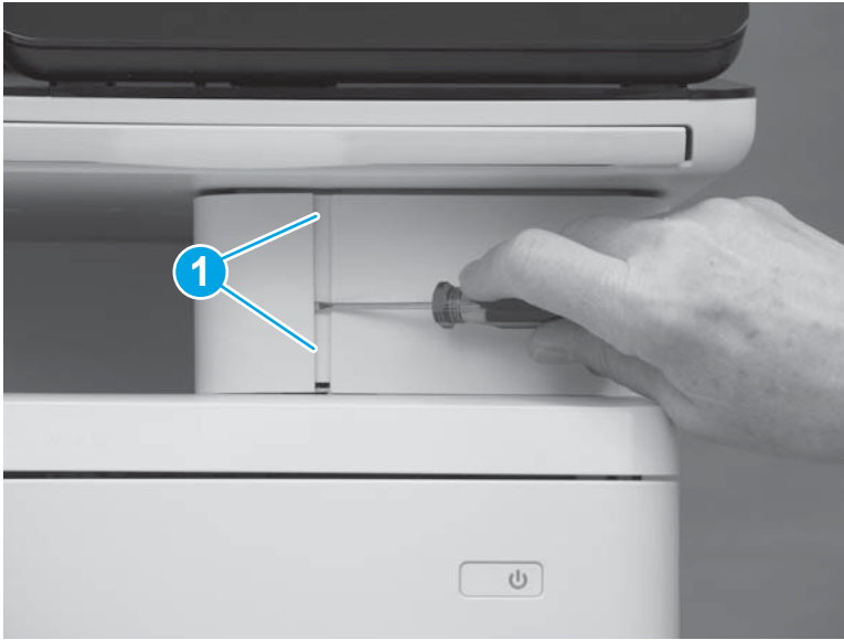
Figure 1-4071 Release two tabs
