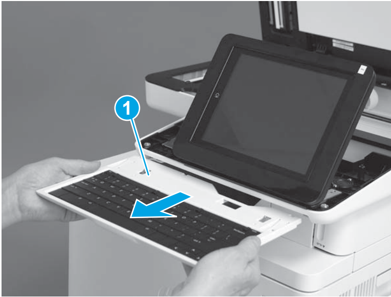
Figure 1-153 Remove the keyboard
