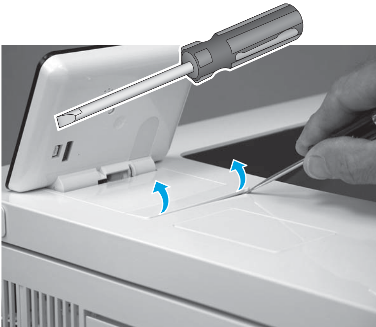
Figure 1-4042 Release the control-panel screws cover tabs
