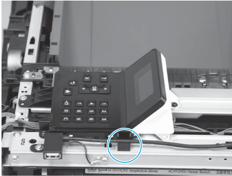
Figure 1-1377 Place one cable in the guide
