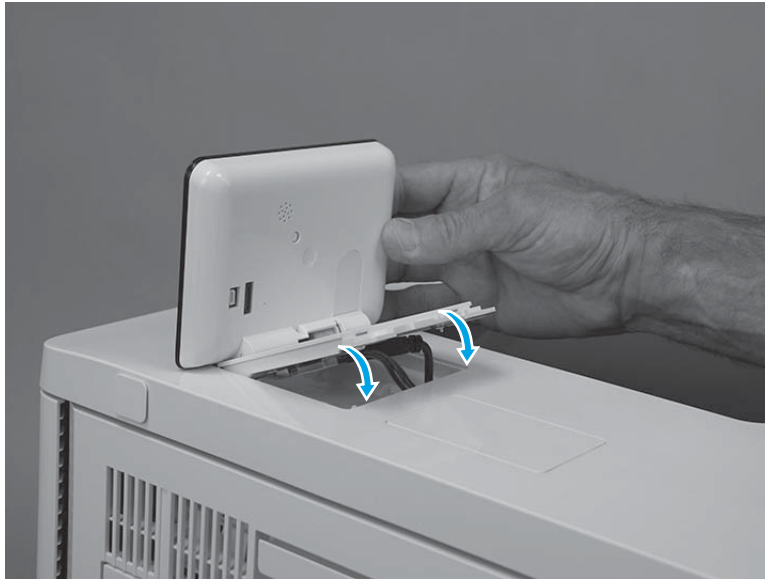
Figure 1-1180 Rotate the control-panel base down
