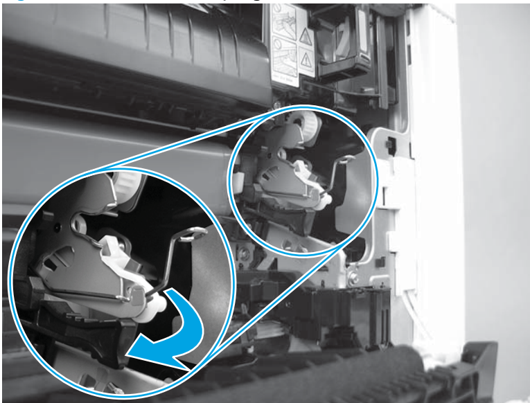
Figure 1-4784 Remove the spring from the holder
