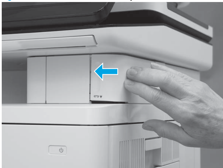
Figure 1-1914 Install the cover assembly
