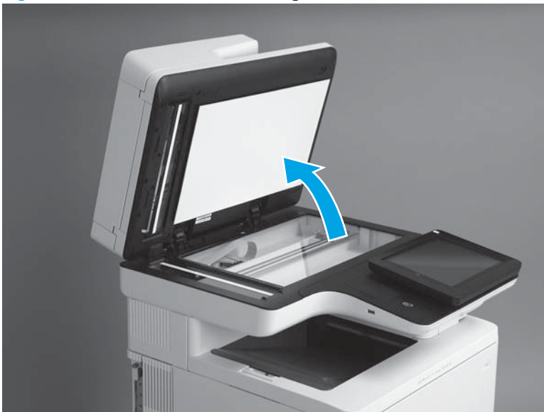
Figure 1-171 Check the white backing
