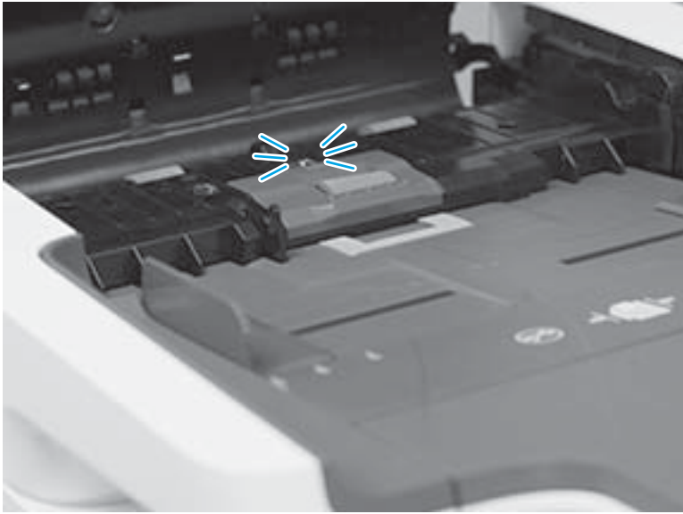
Figure 1-196 Snap the cover closed
