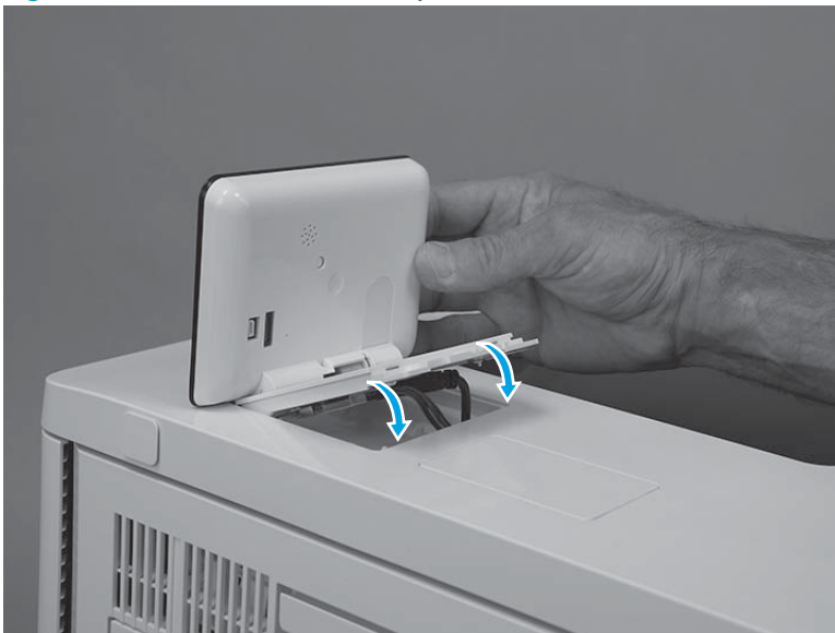
Figure 1-2472 Rotate the control-panel base down
