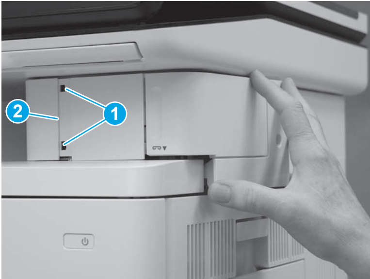
Figure 1-918 Install two tabs
