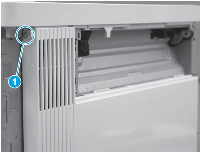
Figure 1-2859 Remove one screw
