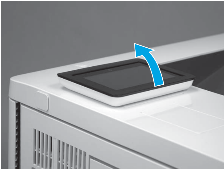
Figure 1-4041 Tilt the control panel up
