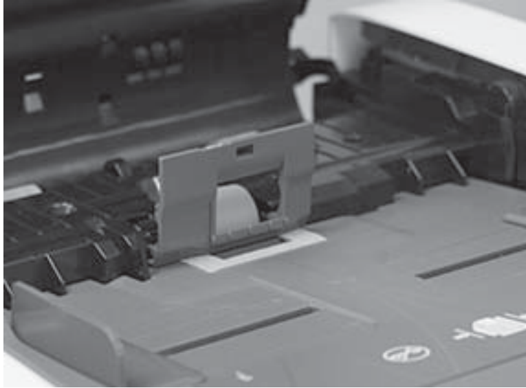
Figure 1-194 Position the separation roller cover
