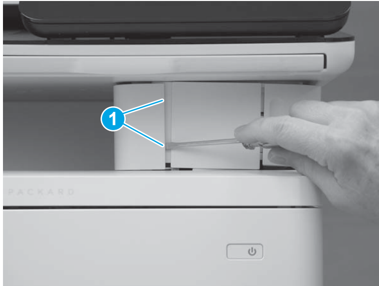
Figure 1-430 Release two tabs
