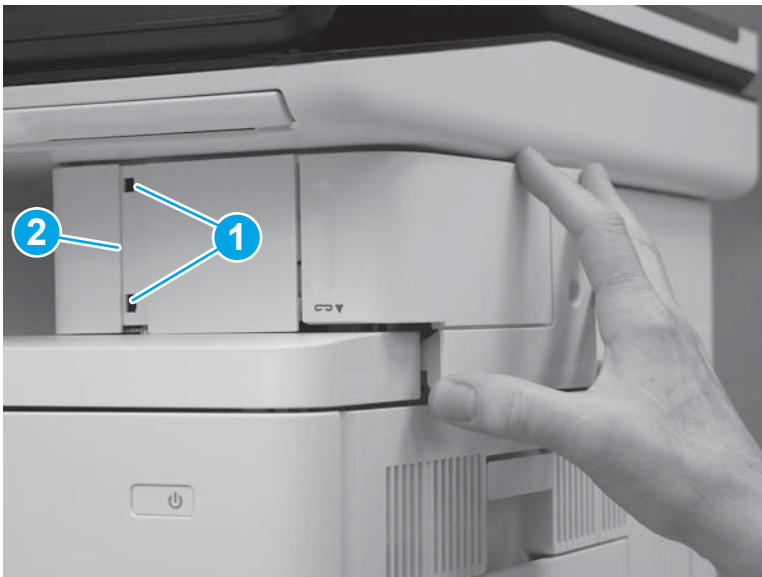
Figure 1-1155 Install two tabs
