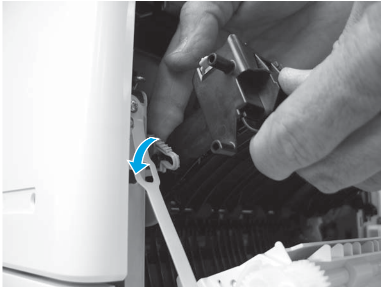
Figure 1-3789 Carefully flex the top portion of the blue arm
