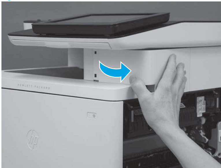
Figure 1-1842 Rotate the cover
