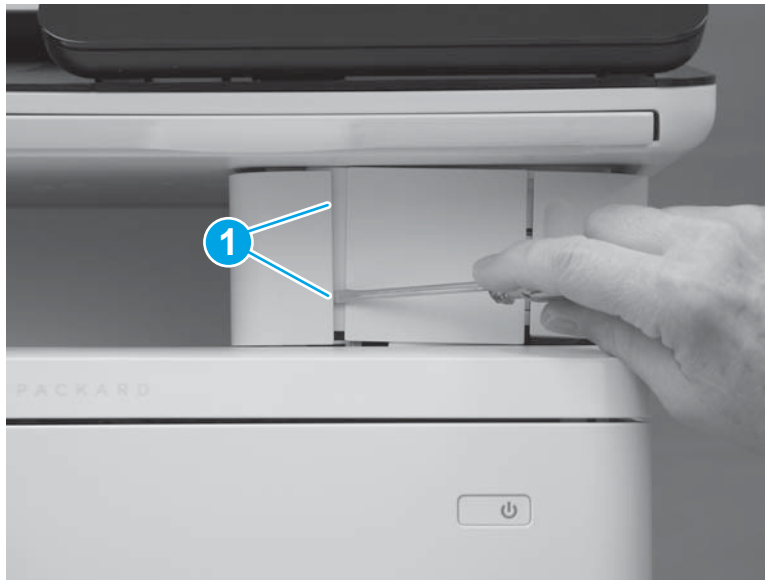
Figure 1-1193 Release two tabs
