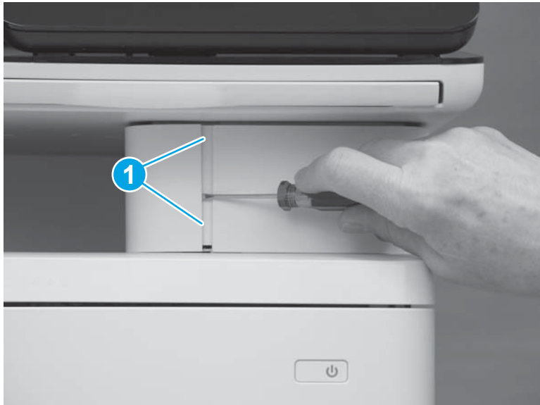
Figure 1-326 Release two tabs
