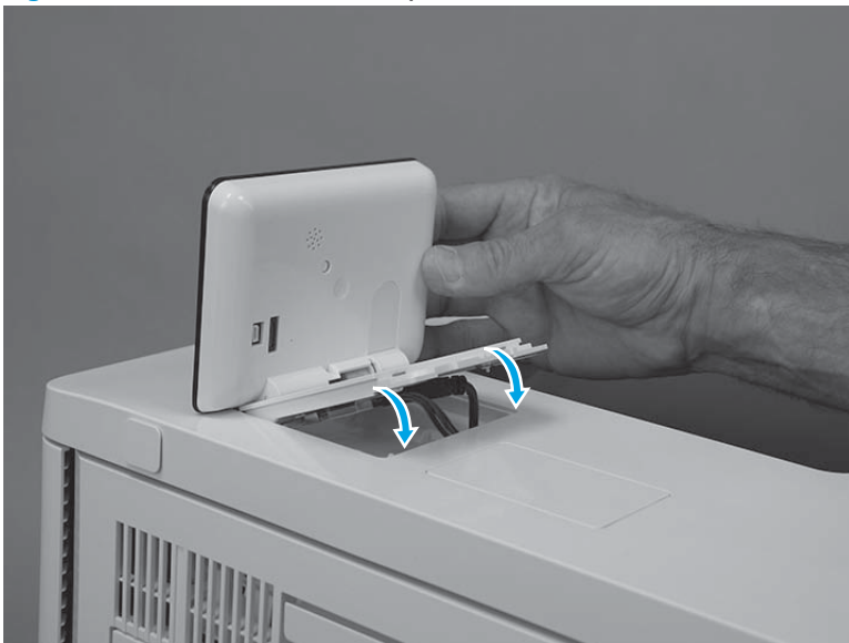
Figure 1-828 Rotate the control-panel base down
