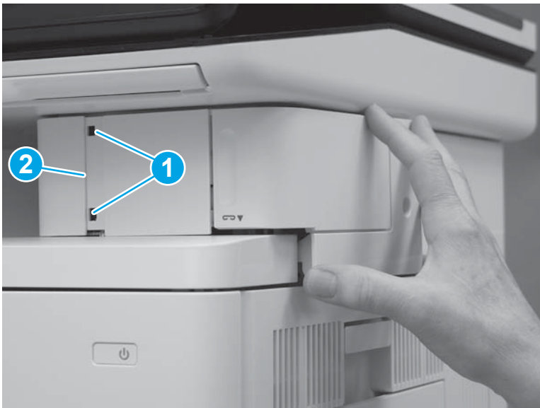
Figure 1-800 Install two tabs
