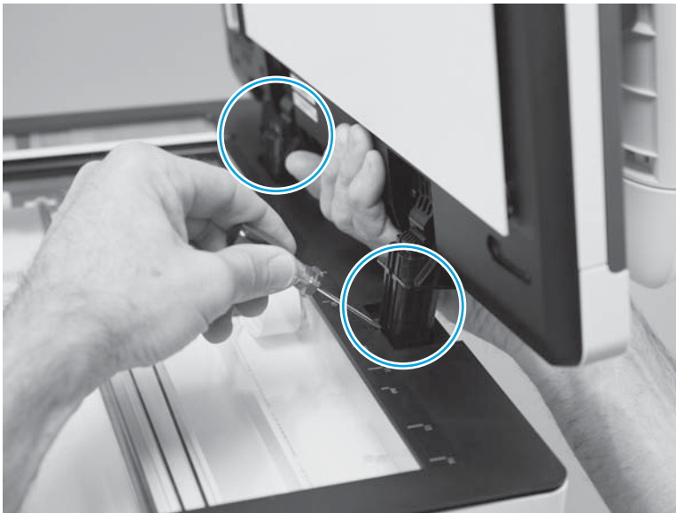
Figure 1-4808 Release two tabs
