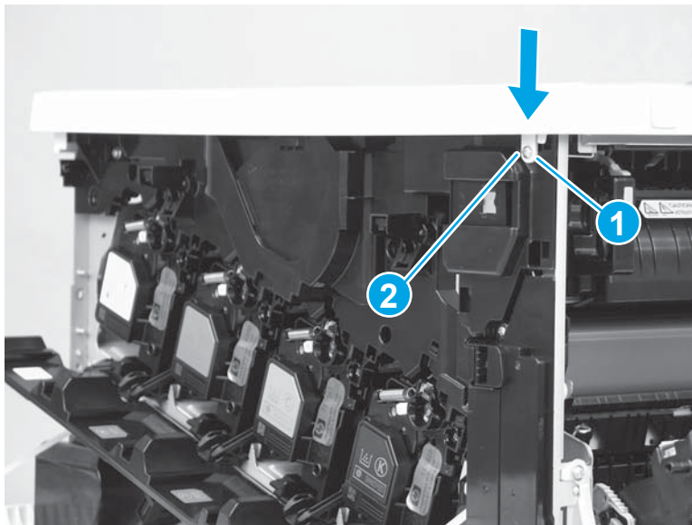
Figure 1-1382 Engage one tab and install one screw
