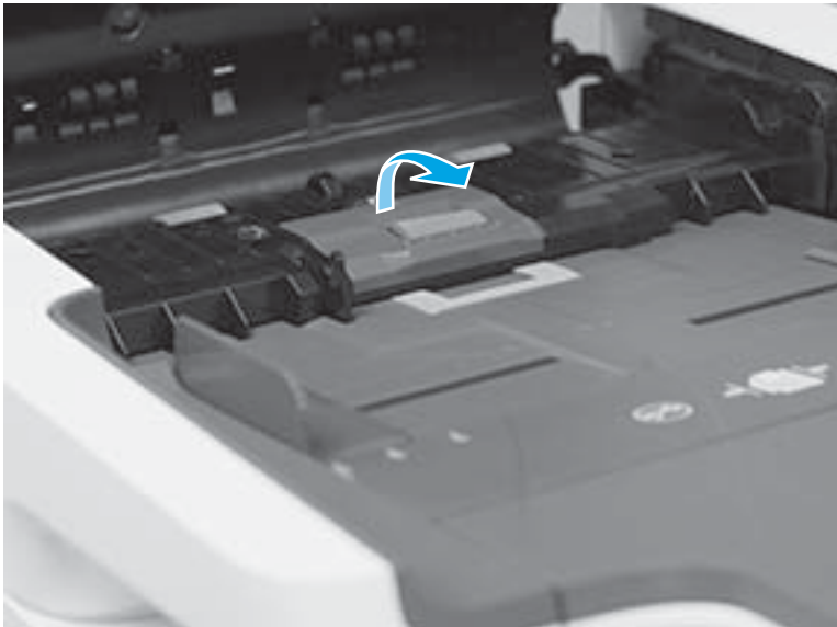
Figure 1-189 Release the separation roller cover
