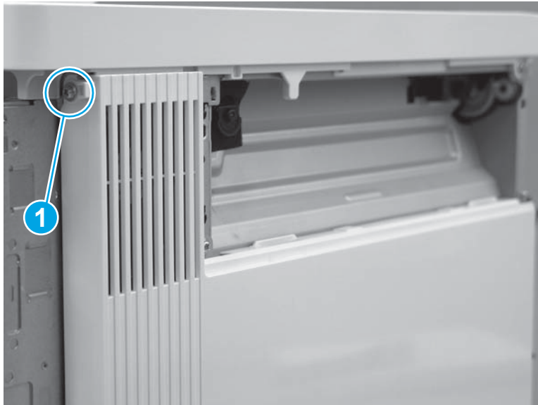
Figure 1-1925 Install one screw
