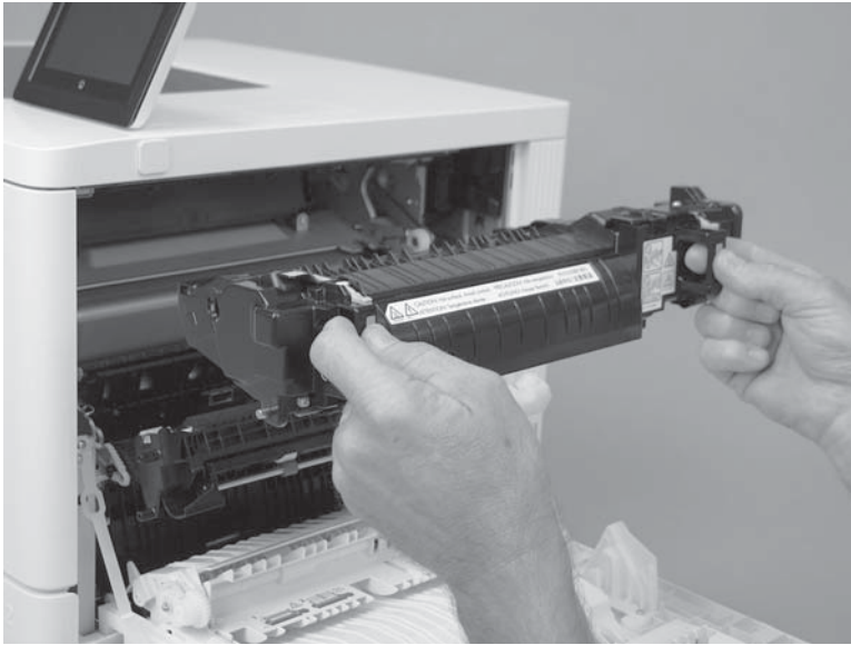
Figure 1-3158 Remove the fuser
