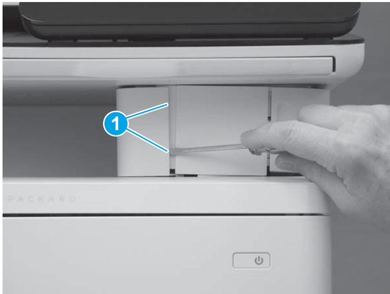
Figure 1-4074 Release two tabs
