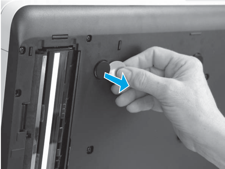
Figure 1-176 Loosen damaged clips
