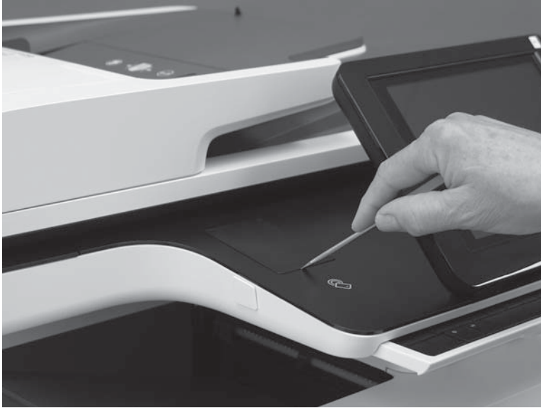
Figure 1-107 Release the HIP cover tabs
