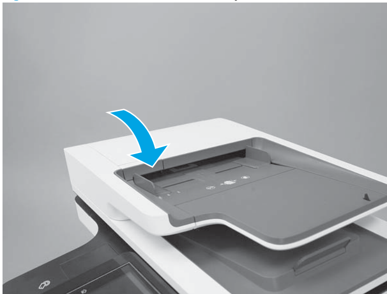
Figure 1-199 Close the document-feeder jam access door
