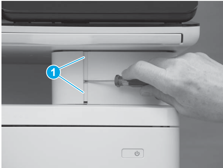
Figure 1-427 Release two tabs
