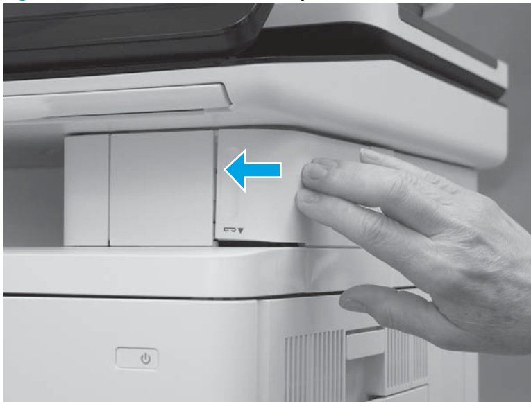
Figure 1-346 Install the cover assembly
