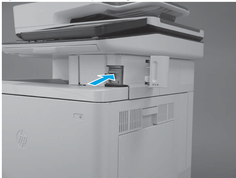
Figure 1-20 Install the staple cartridge
