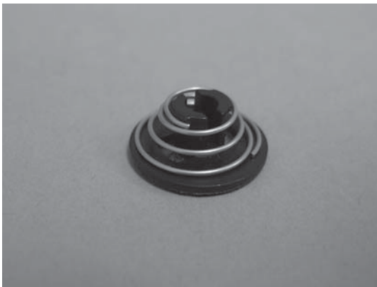
Figure 1-4859 Check the retention clip spring
