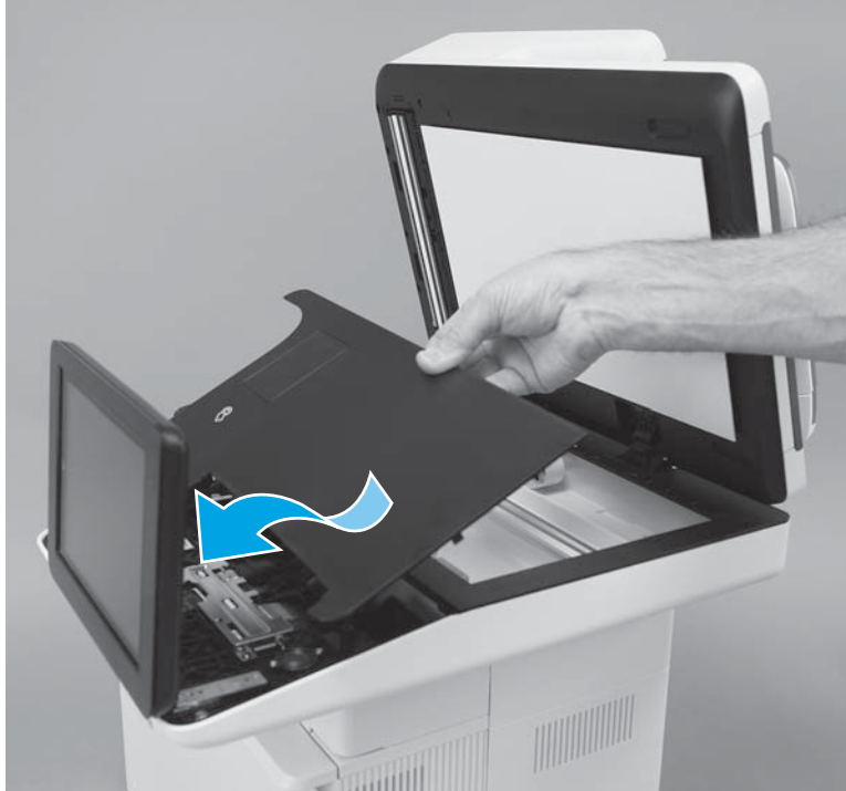
Figure 1-159 Position the control-panel cover on the printer
