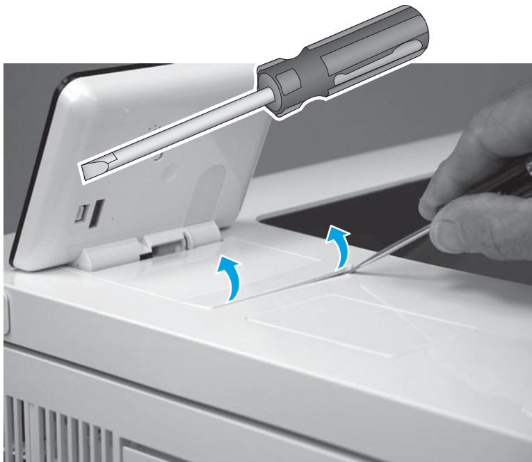
Figure 1-4305 Release the control-panel screws cover tabs
