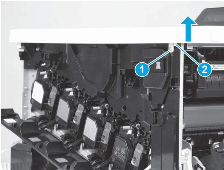
Figure 1-1265 Remove one screw and release one tab
