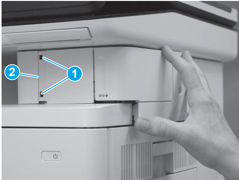
Figure 1-4226 Install two tabs
