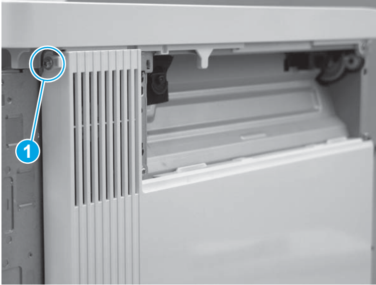
Figure 1-3283 Install one screw
