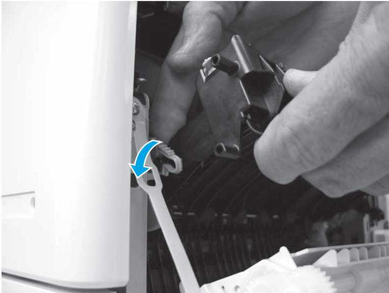
Figure 1-995 Carefully flex the top portion of the blue arm
