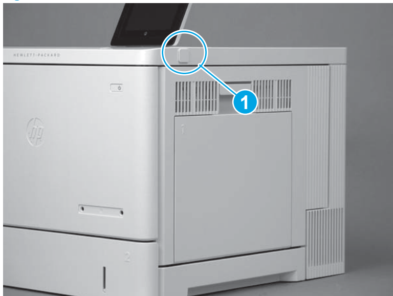
Figure 1-3367 Locate the USB cover
