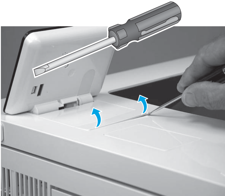
Figure 1-114 Release the control-panel screws cover tabs
