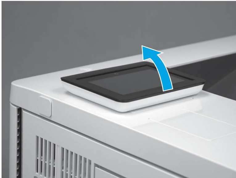
Figure 1-3613 Tilt the control panel up
