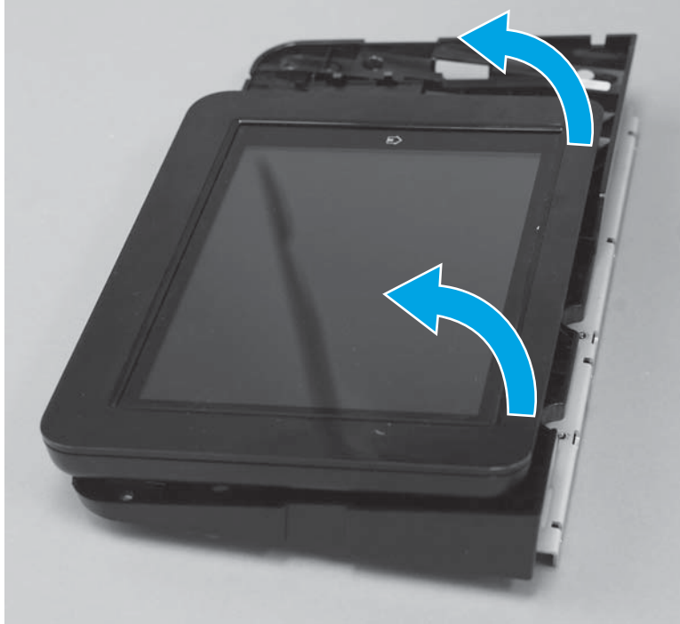
Figure 1-4947 Open the control panel
