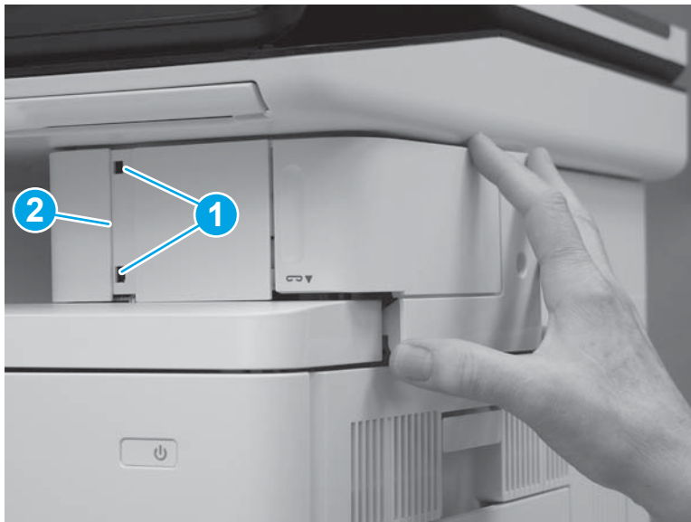
Figure 1-1362 Install two tabs
