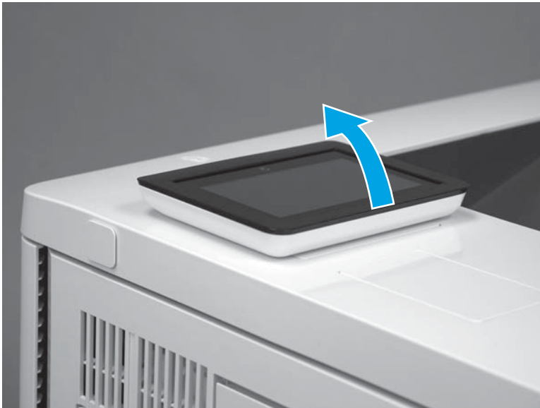
Figure 1-3810 Tilt the control panel up
