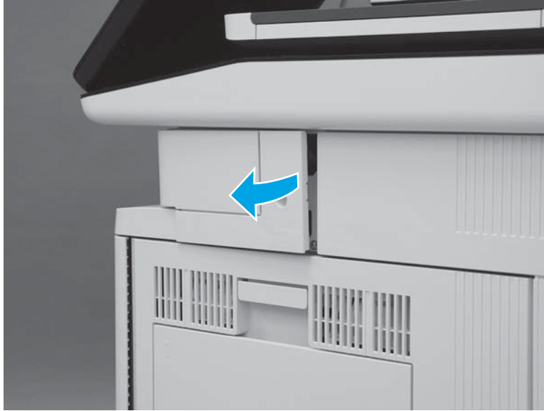
Figure 1-3647 Release the back edge of the cover
