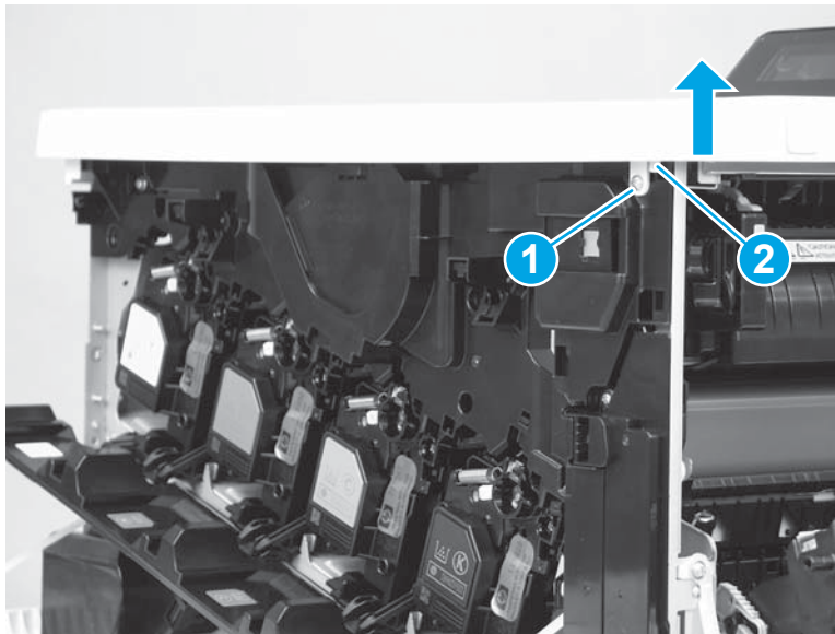
Figure 1-2700 Remove one screw and release one tab
