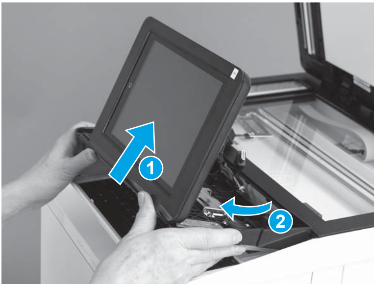
Figure 1-134 Remove the control panel
