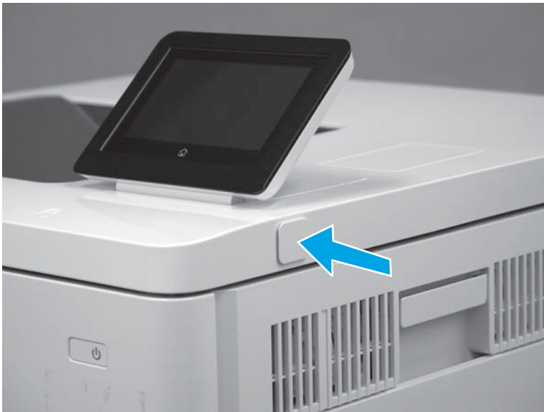
Figure 1-706 Install the cover
