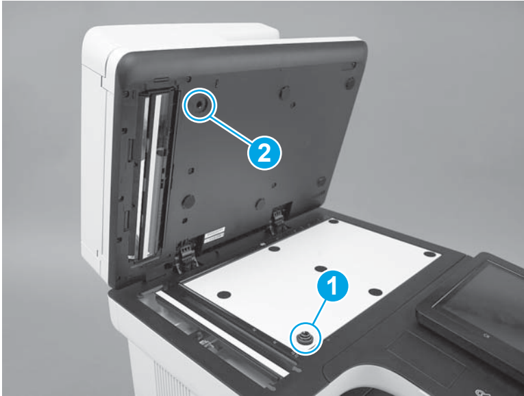
Figure 1-175 Check the retention clips
