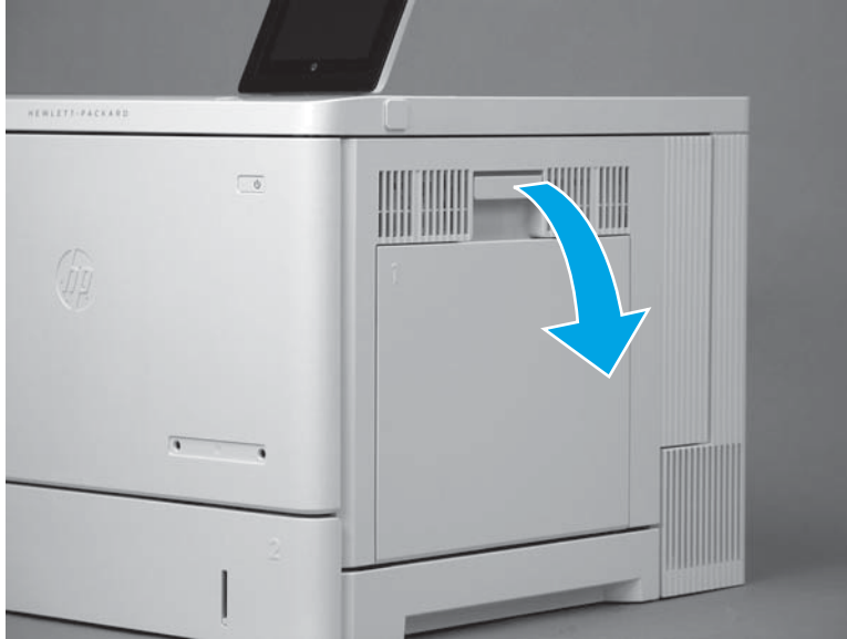
Figure 1-4522 Open the right door
