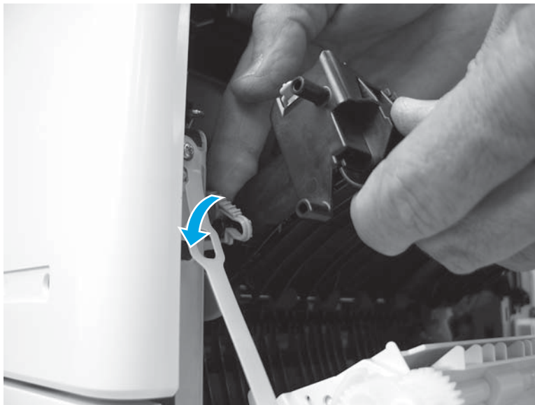
Figure 1-4283 Carefully flex the top portion of the blue arm
