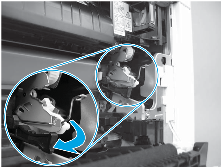
Figure 1-1398 Remove the spring from the holder
