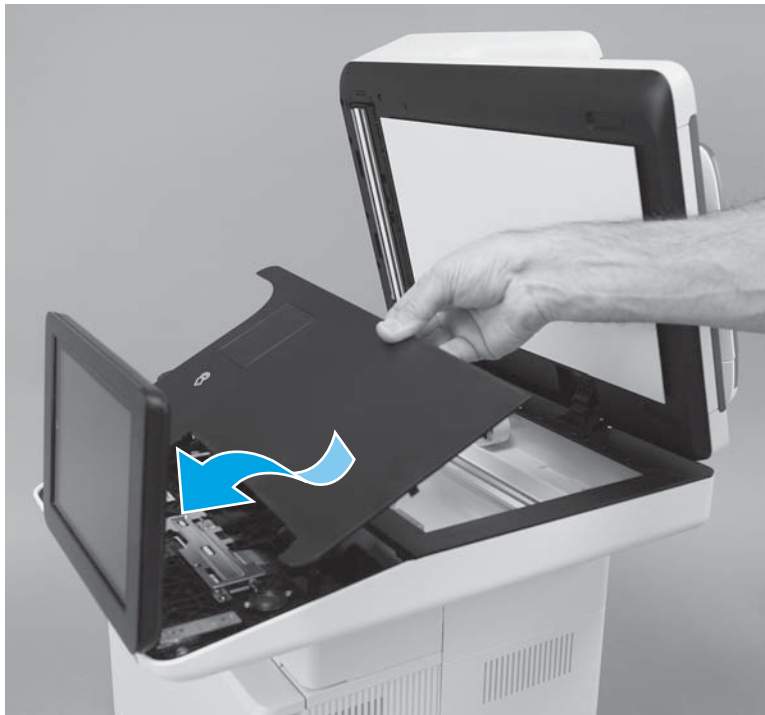
Figure 1-4960 Position the control-panel cover on the printer
