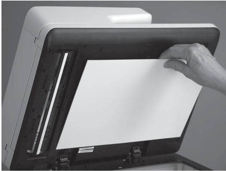
Figure 1-4817 Check the white backing
