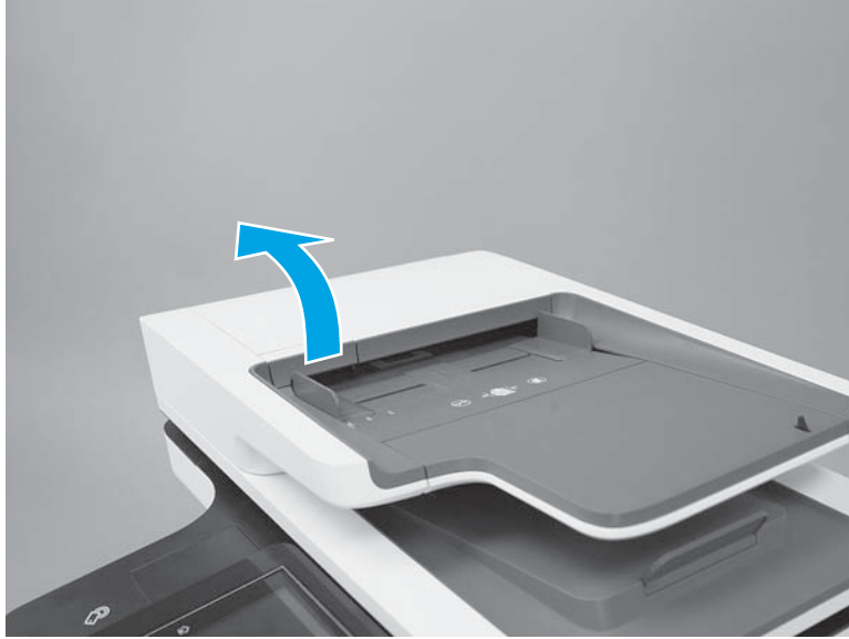
Figure 1-186 Open the document-feeder jam access door
