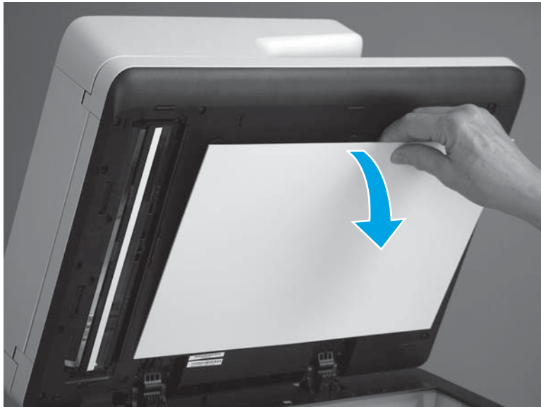
Figure 1-174 Remove the white backing
