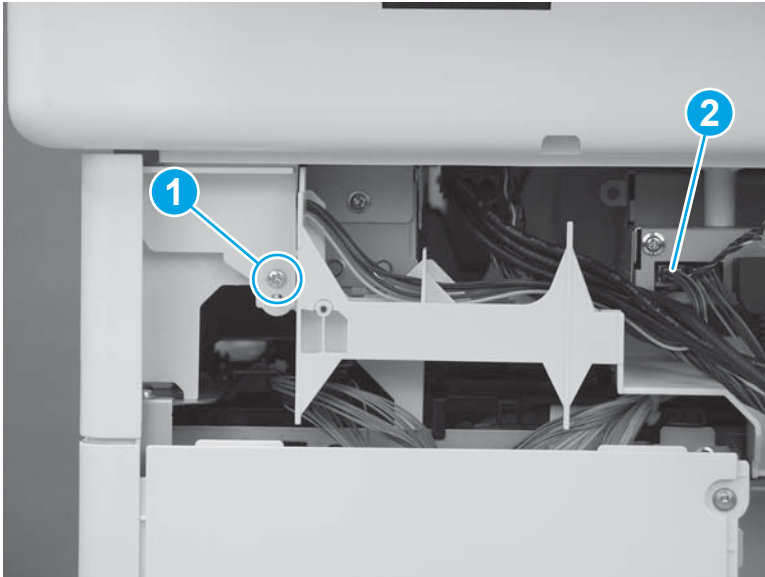
Figure 1-3421 Remove one screw and connector
