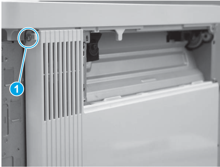
Figure 1-1561 Install one screw
