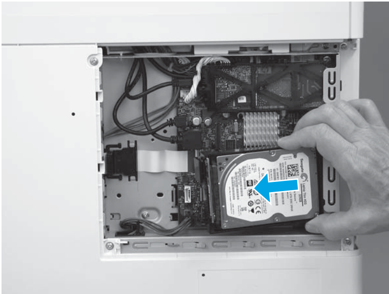
Figure 1-2131 Remove the HDD
