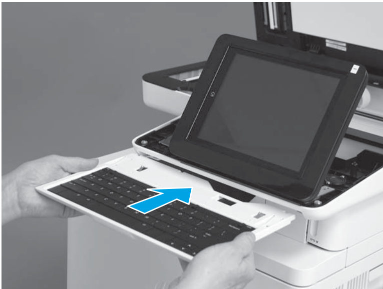
Figure 1-4954 Slide the keyboard into the slot
