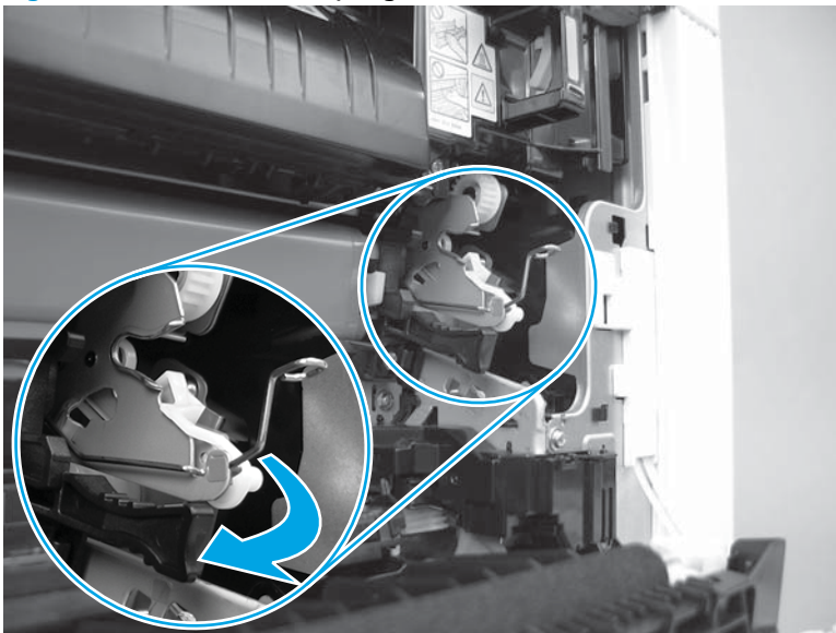
Figure 1-243 Remove the spring from the holder
