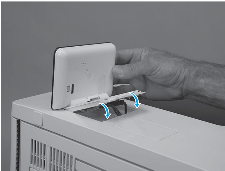
Figure 1-3347 Rotate the control-panel base down
