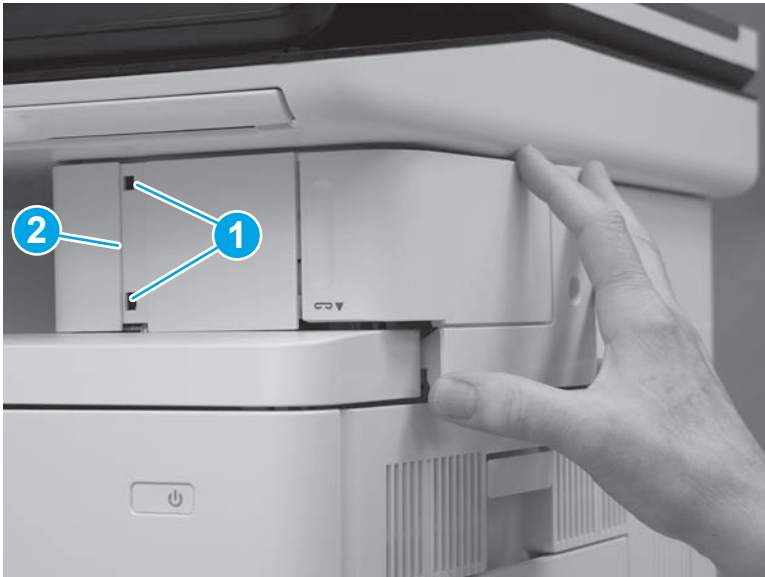
Figure 1-4465 Install two tabs
