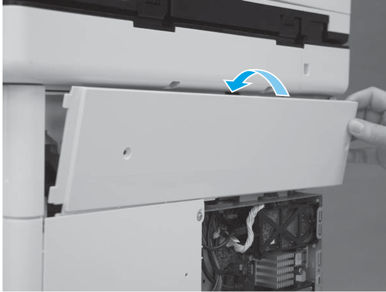
Figure 1-4940 Rotate the top of the cover
