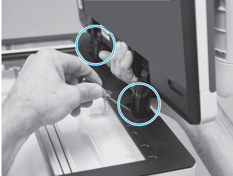
Figure 1-4896 Release two tabs
