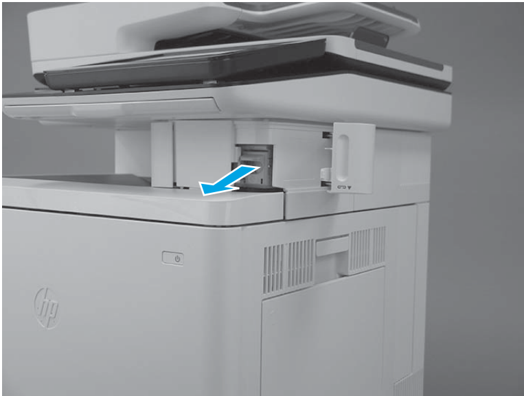
Figure 1-18 Remove the staple cartridge
