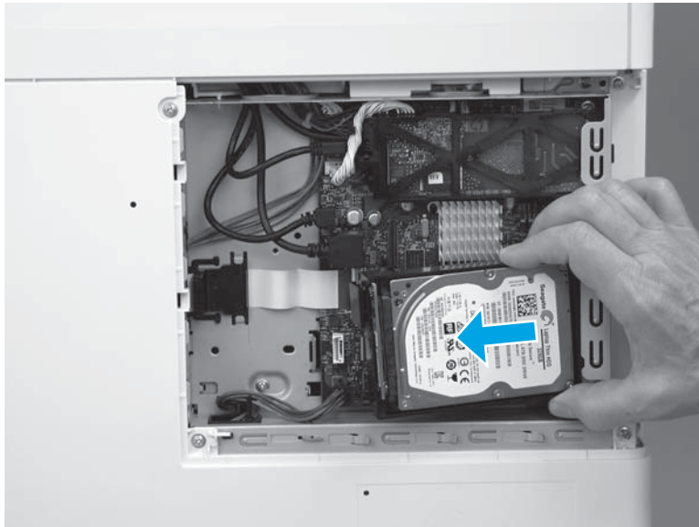
Figure 1-1748 Remove the HDD
