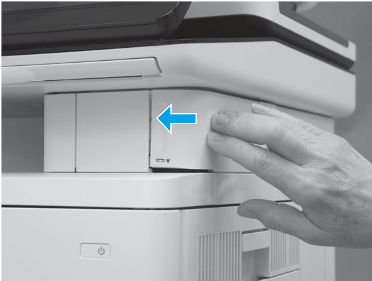
Figure 1-4931 Install the cover assembly
