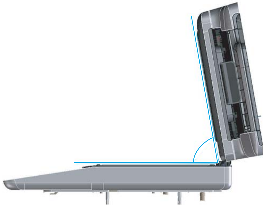
Figure 1-47 Document feeder open (60° to 80°)
