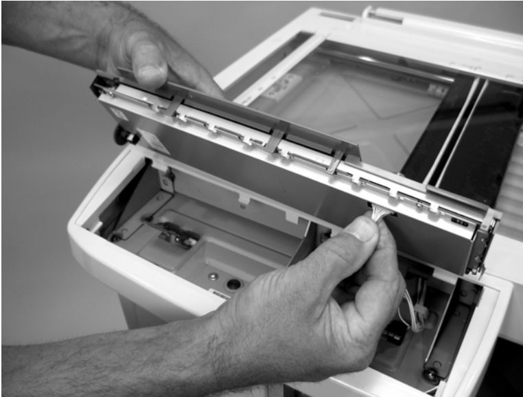
Figure 5-80 Remove the control panel (3 of 3)
