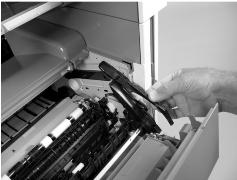
Figure 5-228 Remove the registration assembly (2 of 5)
