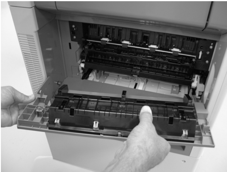
Figure 5-26 Remove the fuser (4 of 6)
