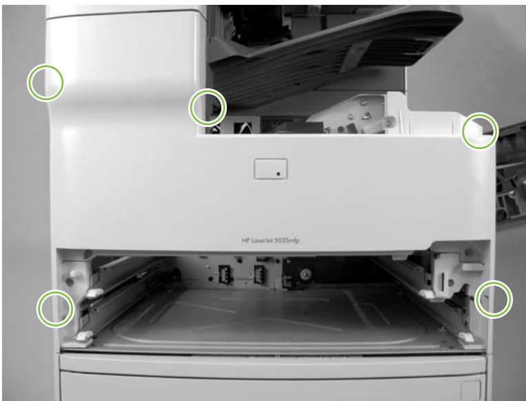
Figure 5-186 Remove the base unit front cover (2 of 7)
