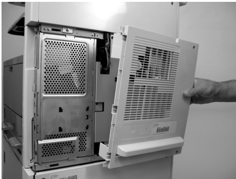
Figure 5-184 Remove the base unit rear cover (2 of 2)
