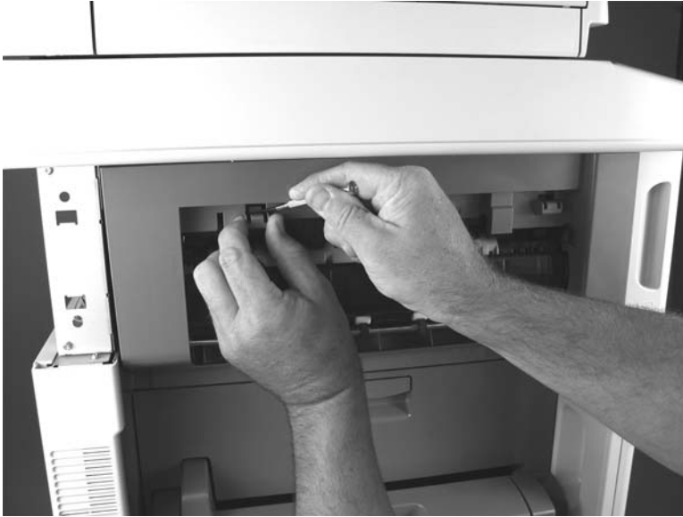
Figure 5-133 Remove the stapler left cover (2 of 3)
