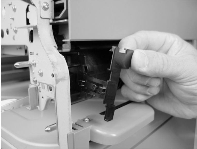
Figure 5-224 Remove the print cartridge door (10 of 12)
