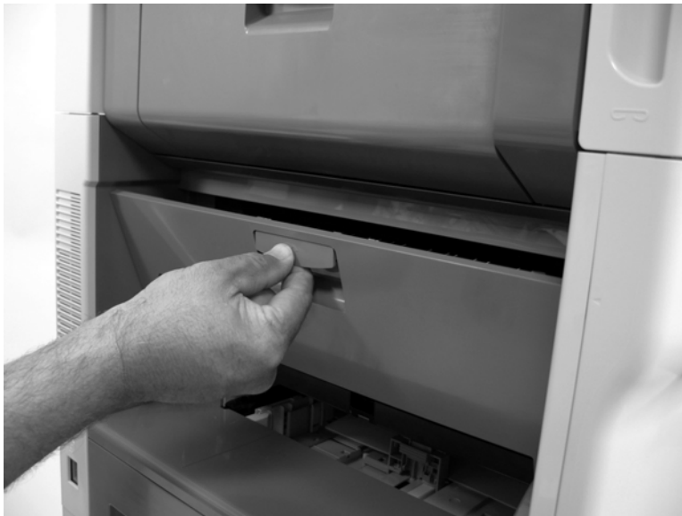
Figure 5-24 Remove the fuser (2 of 6)
