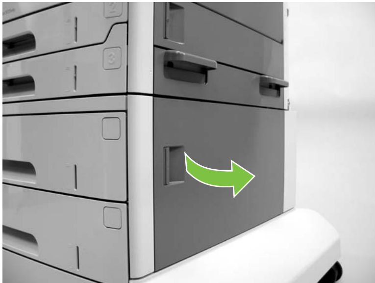
Figure 5-298 Remove the HCI right door (1 of 5)
