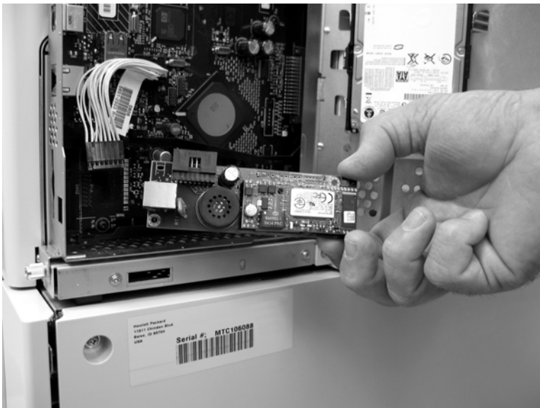
Figure 5-37 Remove the Fax PCA (2 of 2)
