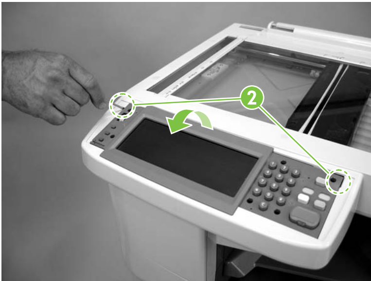
Figure 5-79 Remove the control panel (2 of 3)
