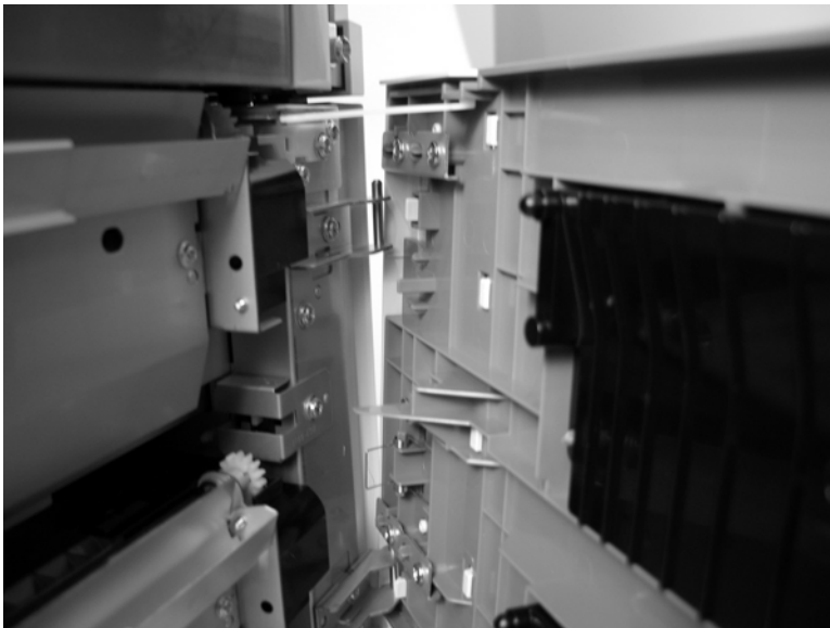
Figure 5-301 Remove the HCl right door (4 of 5)
