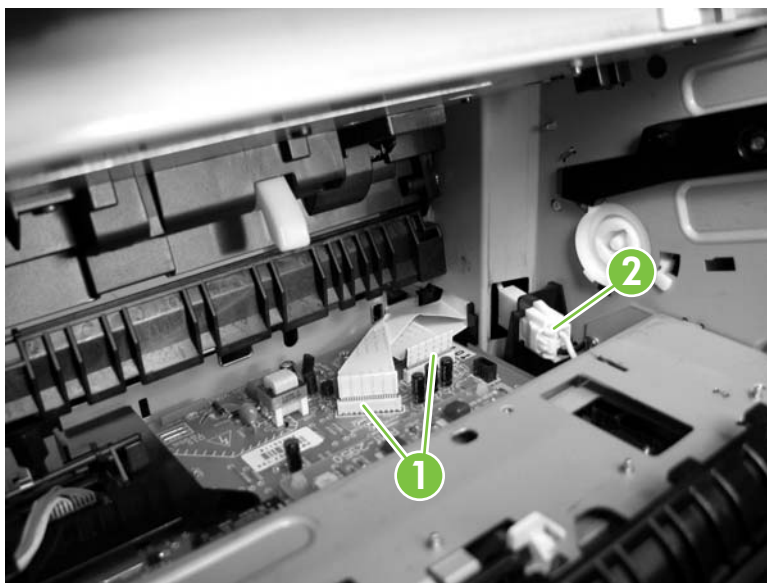
Figure 5-259 Remove the high-voltage power supply assembly (1 of 9)
