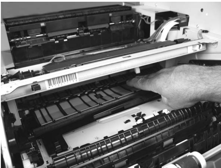
Figure 5-244 Reinstall the paper feed assembly (6 of 8)
