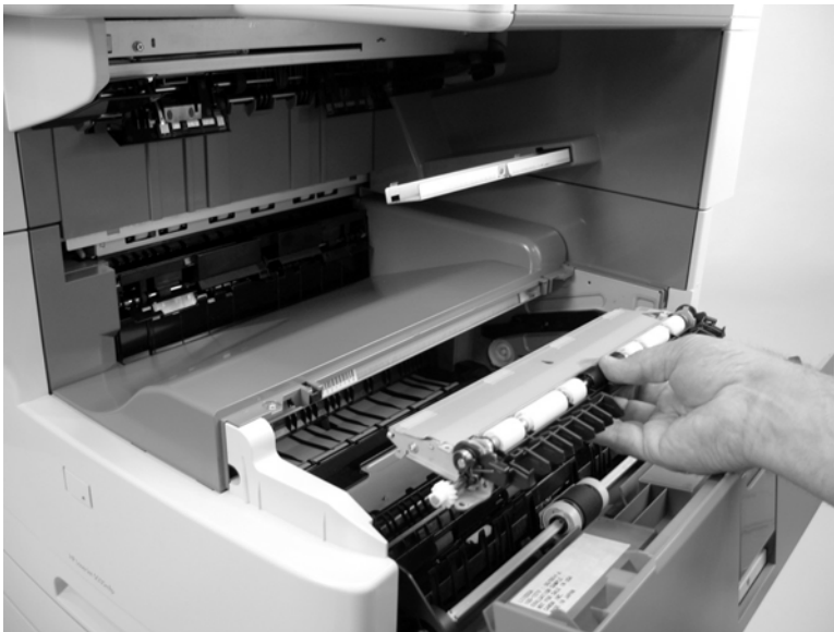
Figure 5-230 Remove the registration assembly (4 of 5)
