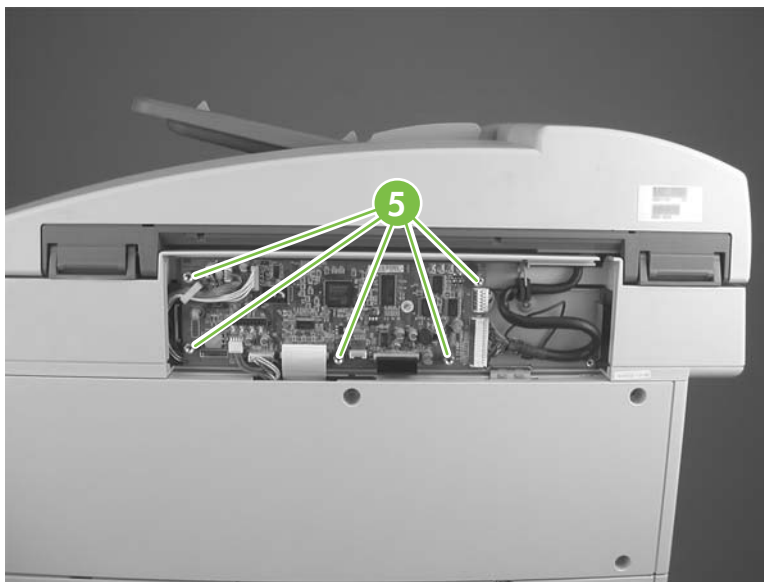
Figure 5-84 Remove the SCB (4 of 4)
