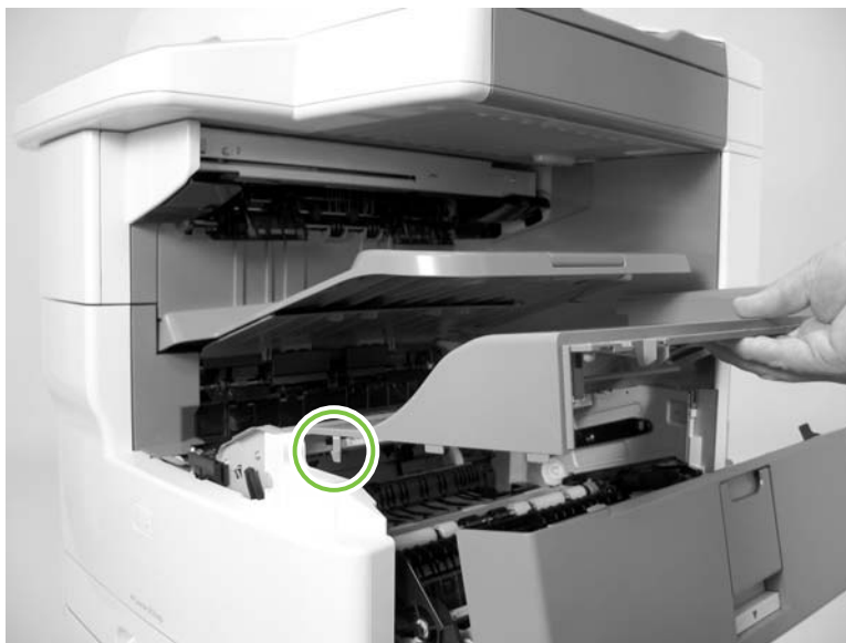
Figure 5-177 Remove the base unit face-down cover (2 of 2)
