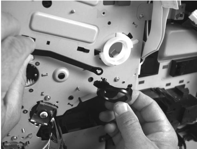
Figure 5-289 Reinstall the print cartridge cam linkage (1 of 2)
