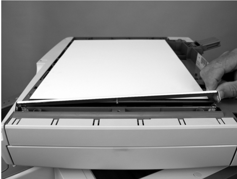
Figure 5-56 Remove the ADF float assembly (3 of 5)
