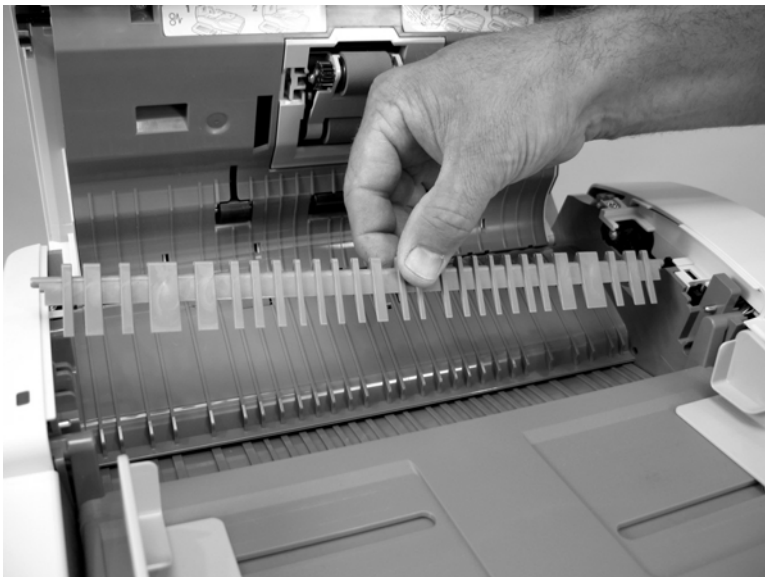
Figure 5-49 Remove the ADF diverter (2 of 2)
