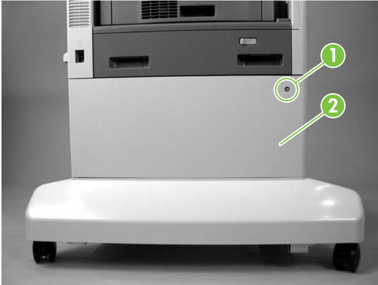
Figure 5-315 Remove the HCI left side tray rail(s) (1 of 3)
