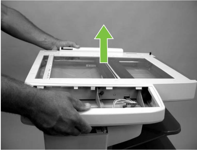
Figure 5-88 Remove the scanner (4 of 4)
