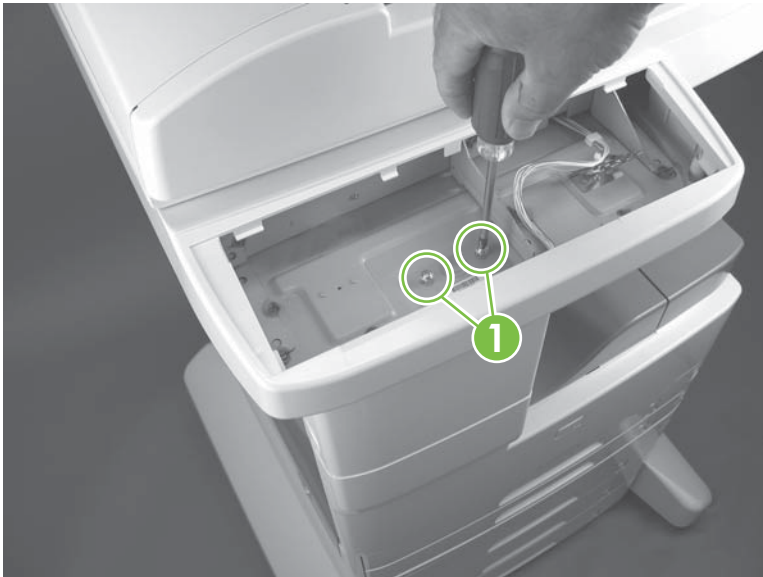
Figure 5-140 Remove the stapler front door and stapler unit cover (1 of 7)
