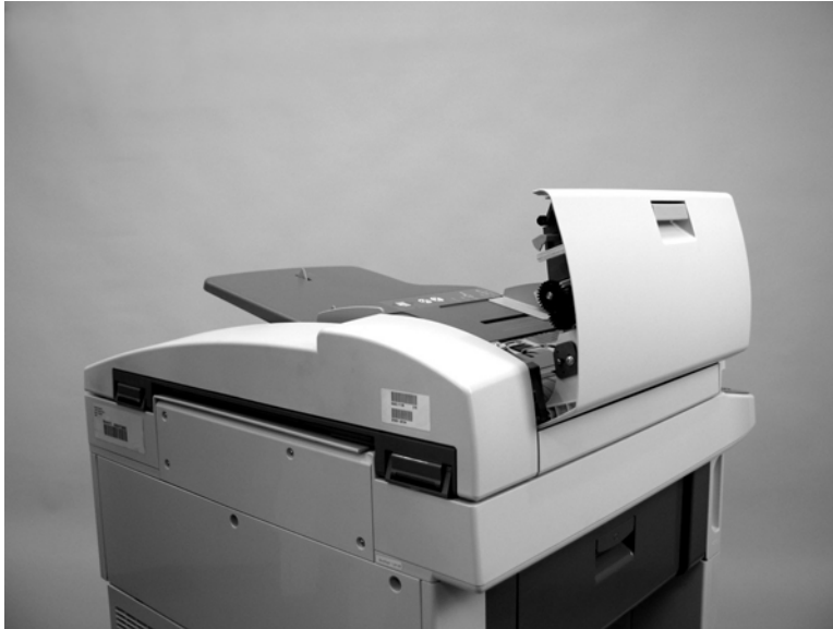
Figure 5-50 Remove the ADF jam cover (1 of 3)
