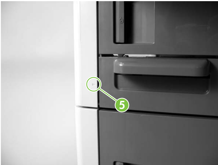
Figure 5-190 Remove the base unit front cover (6 of 7)
