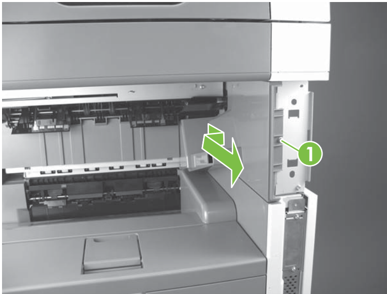
Figure 5-148 Remove the stapler rear inner cover
