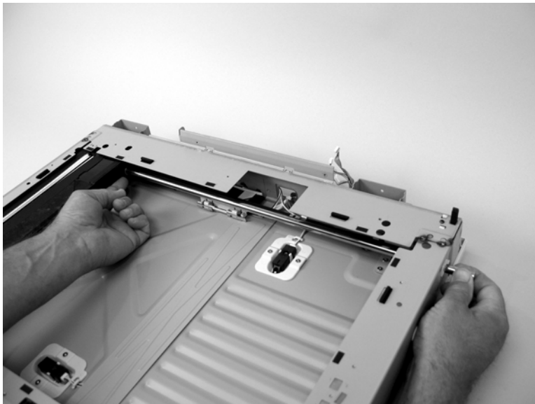
Figure 5-99 Remove the scanner optic assembly (4 of 13)
