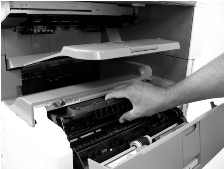
Figure 5-3 Remove the print cartridge (2 of 2)
