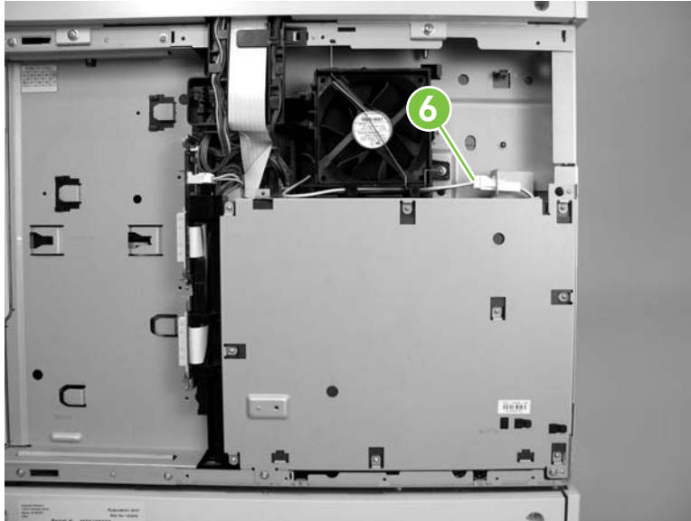
Figure 5-253 Remove the low-voltage power supply assembly (2 of 4)
