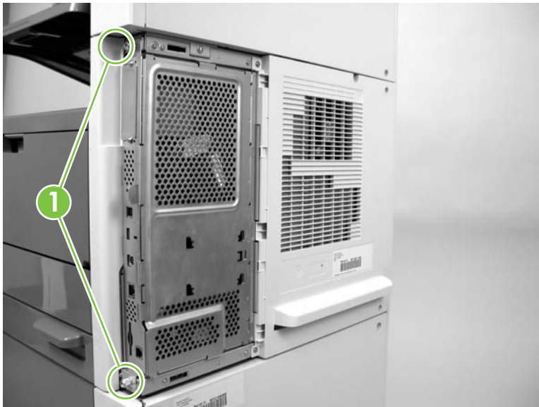
Figure 5-31 Remove the formatter cover and cage (2 of 3)
