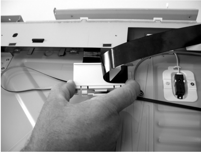
Figure 5-108 Remove the scanner optic assembly (13 of 13)
