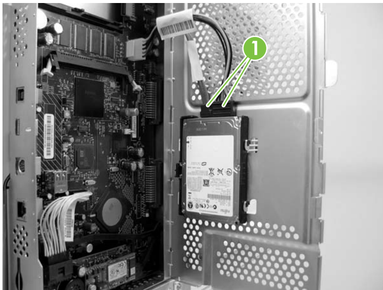
Figure 5-34 Remove the hard drive (1 of 2)
