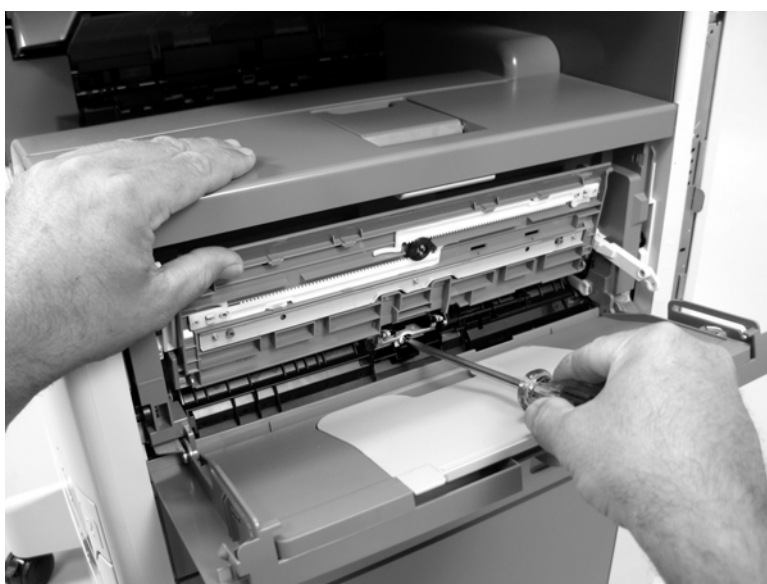
Figure 5-14 Remove the Tray 1 separation pad assembly (2 of 3)
