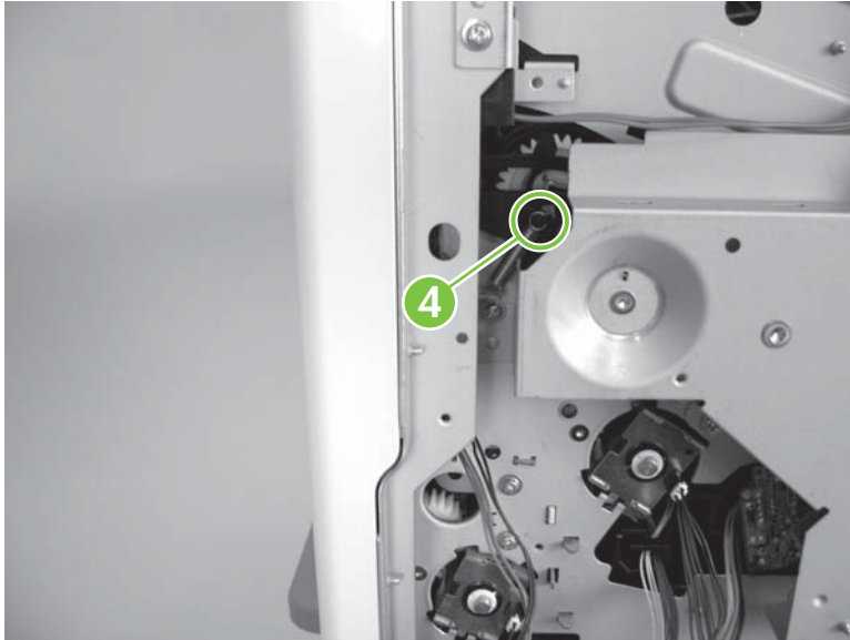
Figure 5-285 Remove the main motor (4 of 7)
