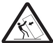
**CAUTION:** Floor-mounted configurations require furniture for stability. You must use either a printer stand or printer base if you are using a 2000-sheet drawer. Certain other configurations also must have a printer stand or printer base. More information is available at our Lexmark Web site at [www.lexmark.com/multifunctionprinters](http://www.lexmark.com/multifunctionprinters).
