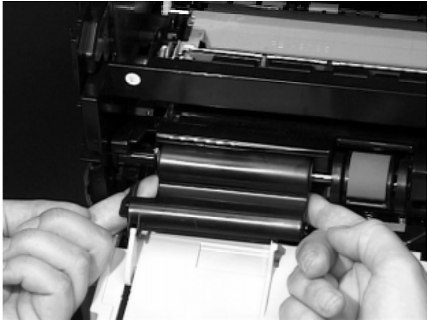
Figure 6-12 Removing the Tray 1 Sensor Arm Cover
