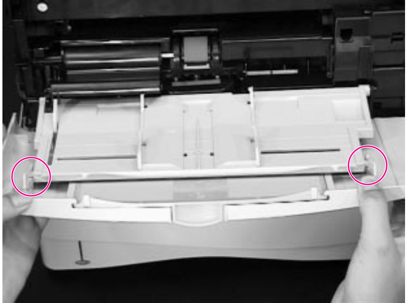
Figure 6-11 Removing Tray 1 from the Front Cover
