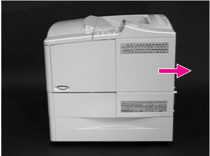
Figure 6-2 Removing the Rear Right Side Cover
