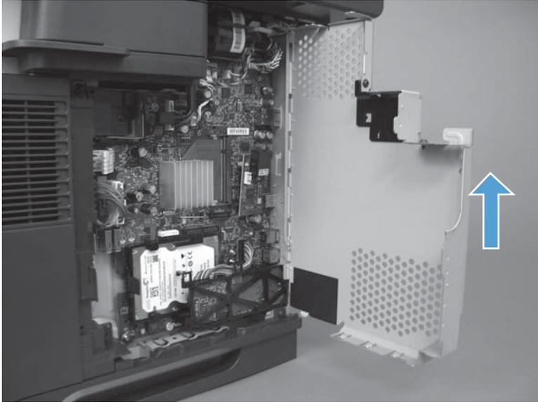
4. Push the locking lever to release the hard drive.
