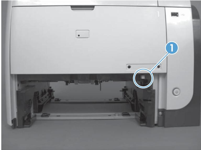
4. Use a small flat blade screwdriver to carefully pry the sheet-metal tab on the assembly away from the hinge pin to release it.
