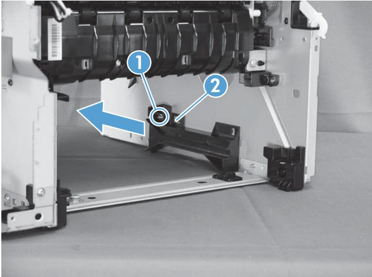
7. Put the product on its side so that the gear cover faces up. Remove three screws (callout 1) and the gear cover.
