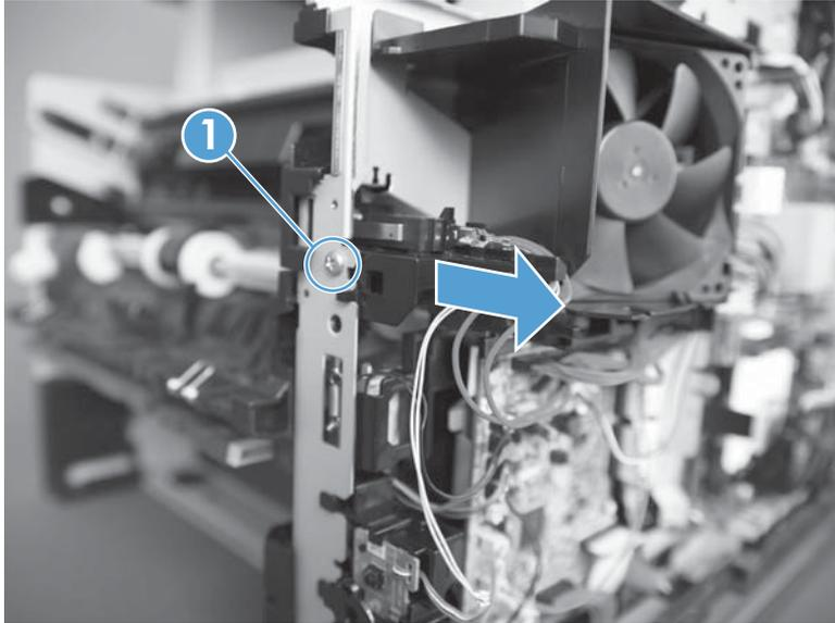
4. Release two tabs (callout 1), and then carefully remove two wire connectors.
