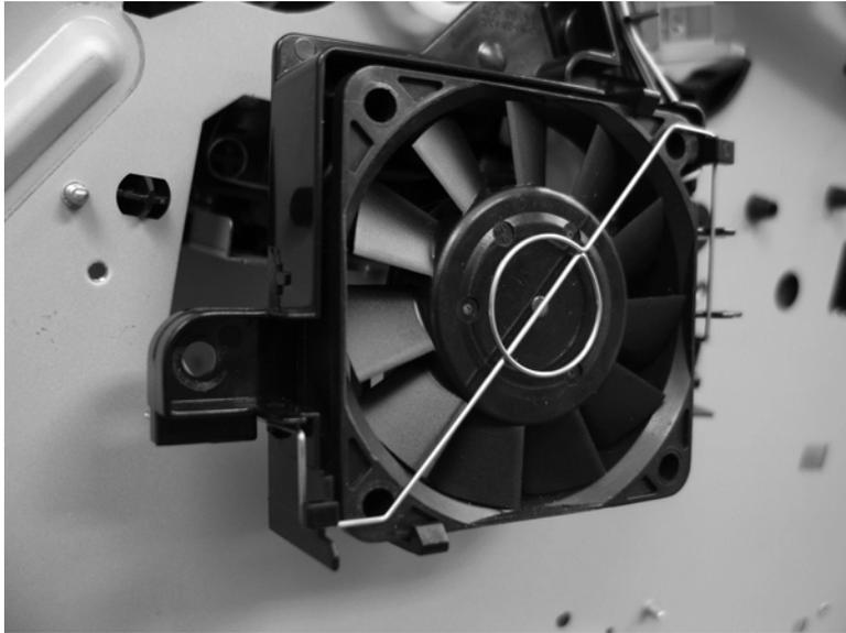
**Figure 1-231** Reinstall the sub fan (2 of 2)
