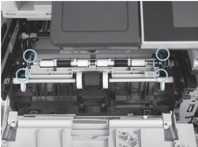
4. Lift the registration roller assembly out of the product, gear-end first.
