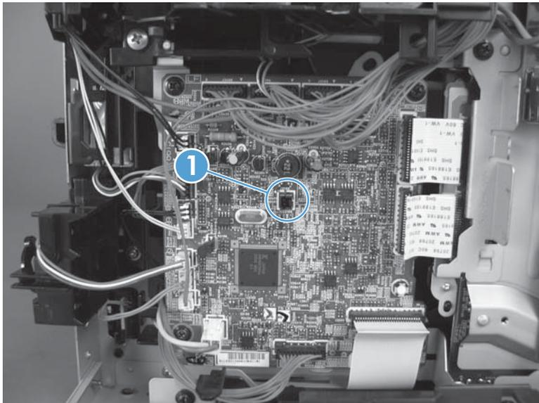
3. Release two tabs, and then carefully remove two wire connectors from the interlock switch assembly.
