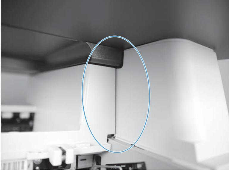
**Figure 1-97** Reinstall the right cover assembly: incorrect alignment
