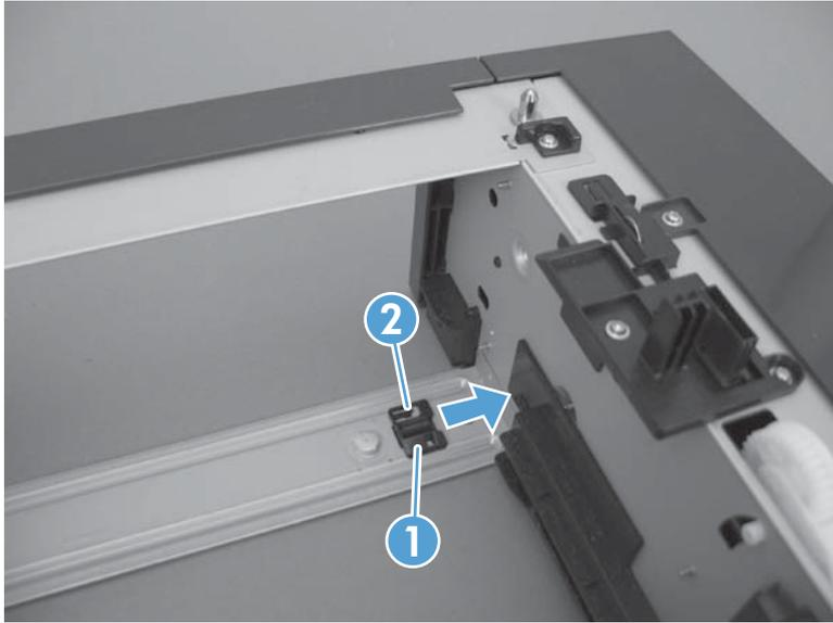
3. Remove the base plate roller assembly.
