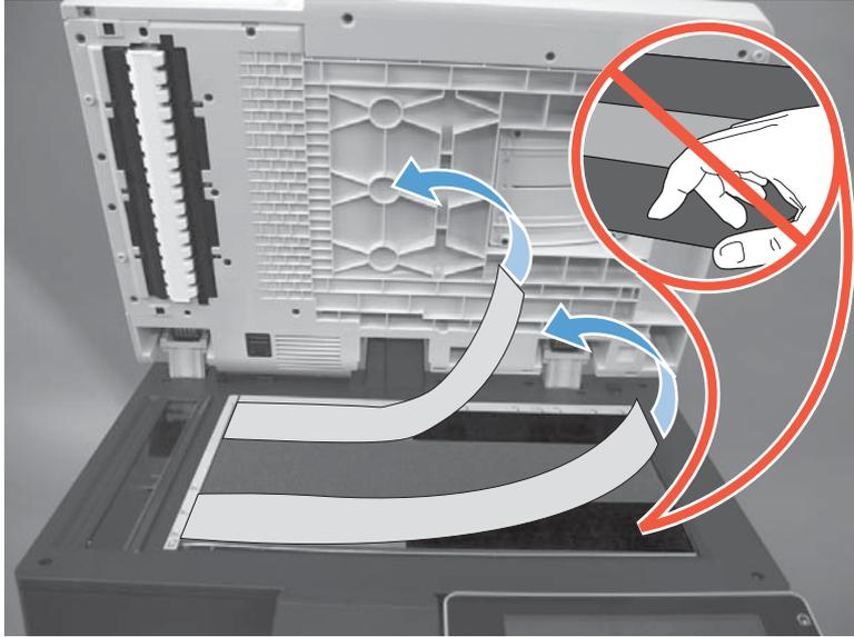
3. Make sure the corner of the foam reflector is aligned with the corner of the scanner glass.
