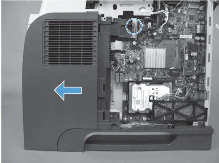
6. If necessary, remove two screws (callout 1), release two tabs (callout 2), and then slide the front-right cover toward the top of the right-side cover to release it.
