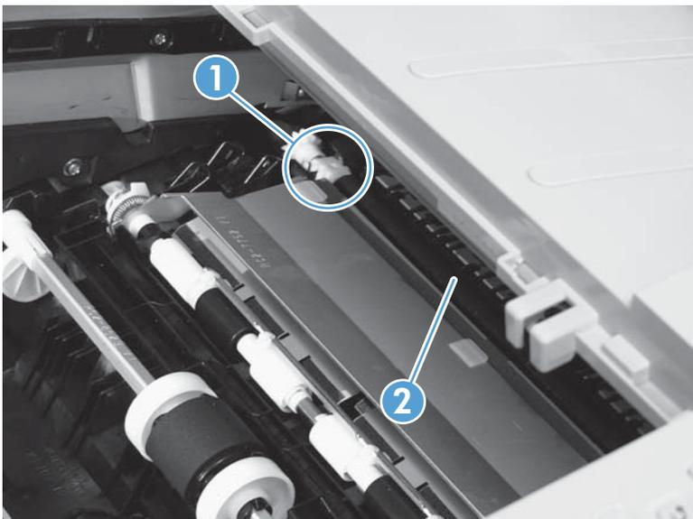
3. If necessary, remove the gear, the bushing, and the spring, and then install them on a replacement roller.
