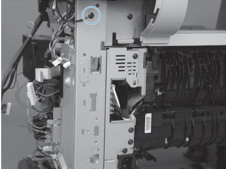
4. Slide the sheet-metal bracket up to release it, and then remove the bracket.
