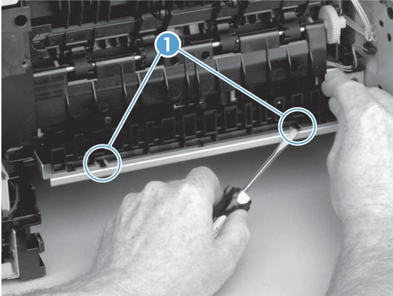
3. Press the green lever (callout 1) to release the duplex media-feed assembly.
