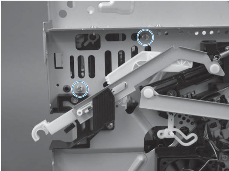
4. Release four wire harness holders from the chassis and then rotate the output bin roller assembly up to expose the pendulum assembly.
