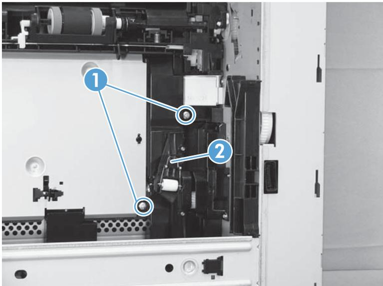
12. Remove two screws (callout 1), and then remove the plate (callout 2).
