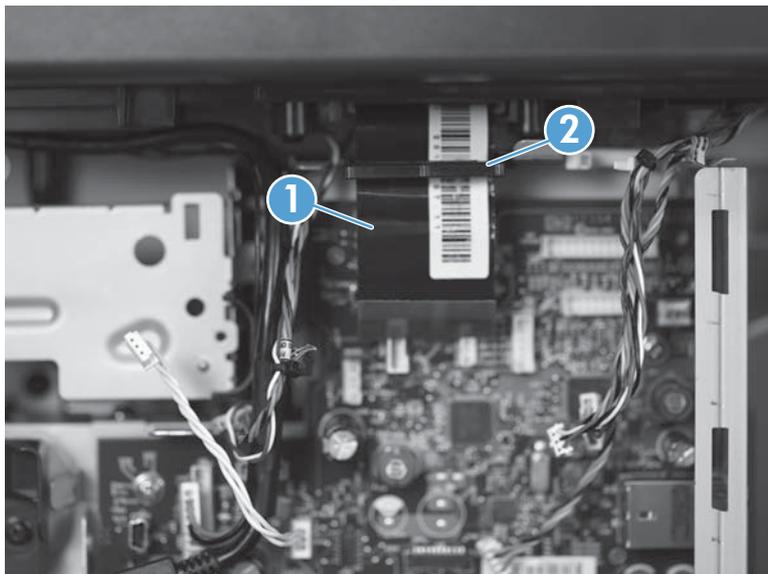
7. Slide the scanner toward the rear of the product (callout 1) until it stops. Lift the scanner (callout 2) to remove.
