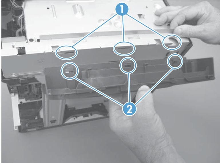
2. Rotate the cover up to engage the tabs with the slots, and then slide the cover toward the front of the product to install it.
