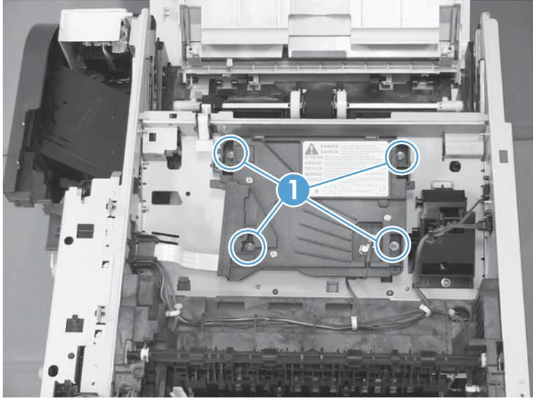
6. Lift the laser scanner up and out of the product.
