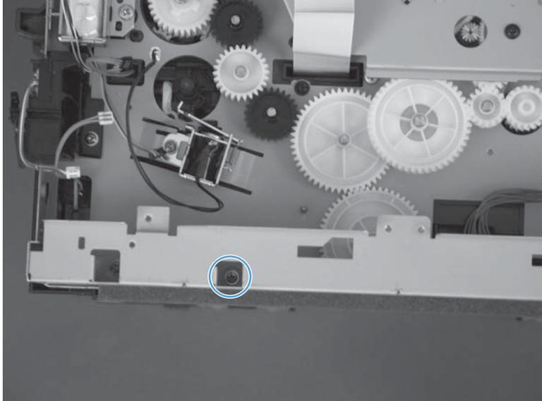
3. Place the product on its rear side. Remove one screw, and then remove the base plate (callout 2).
