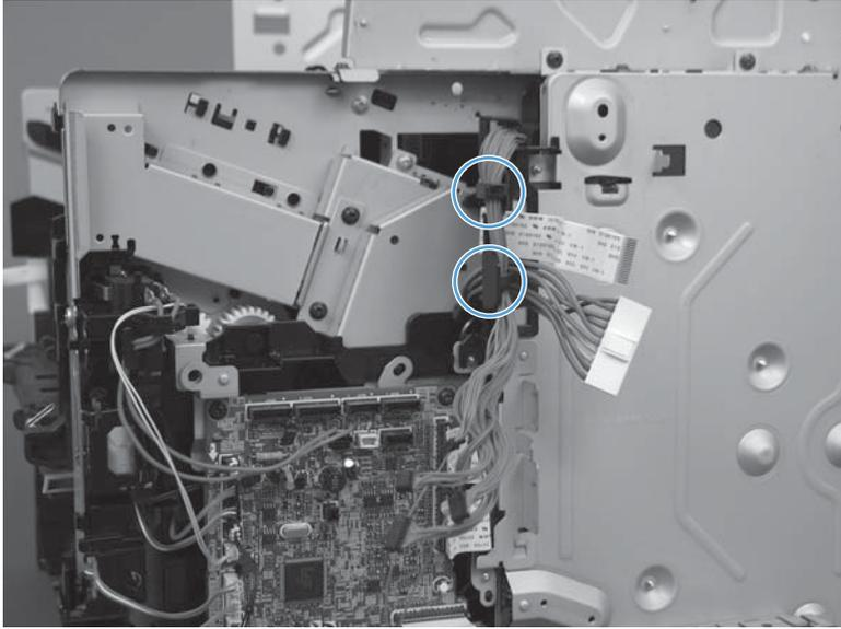
9. Remove six screws (callout 1) and disconnect one connector (callout 2).
