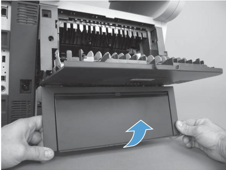
8. Pull down on the rear cover assembly to remove it.
