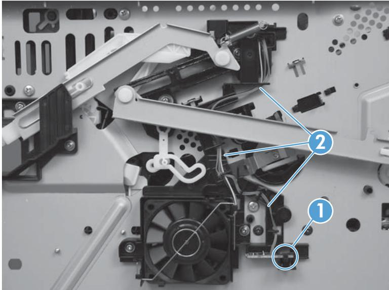
3. Release the wire harness from the retainers (callout 1), and then remove the sensor.
