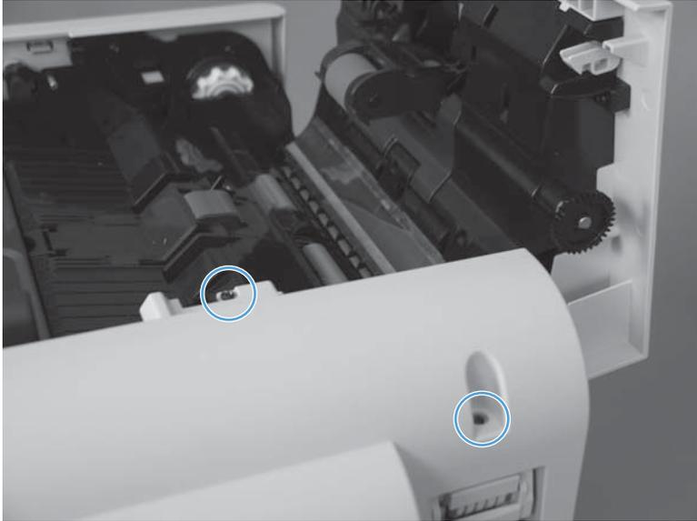
4. Release six tabs and remove the cover.
