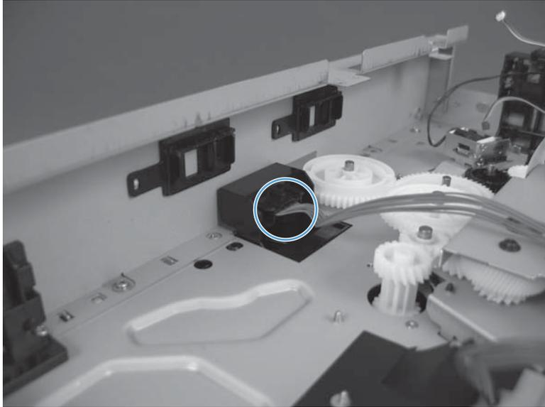
7. Remove one screw (callout 1), release one tab (callout 2) and then slide the guide toward the front of the product to release it.
