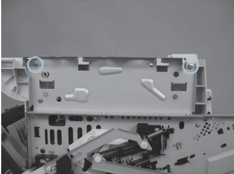
4. Separate each side of the top cover from the chassis.
