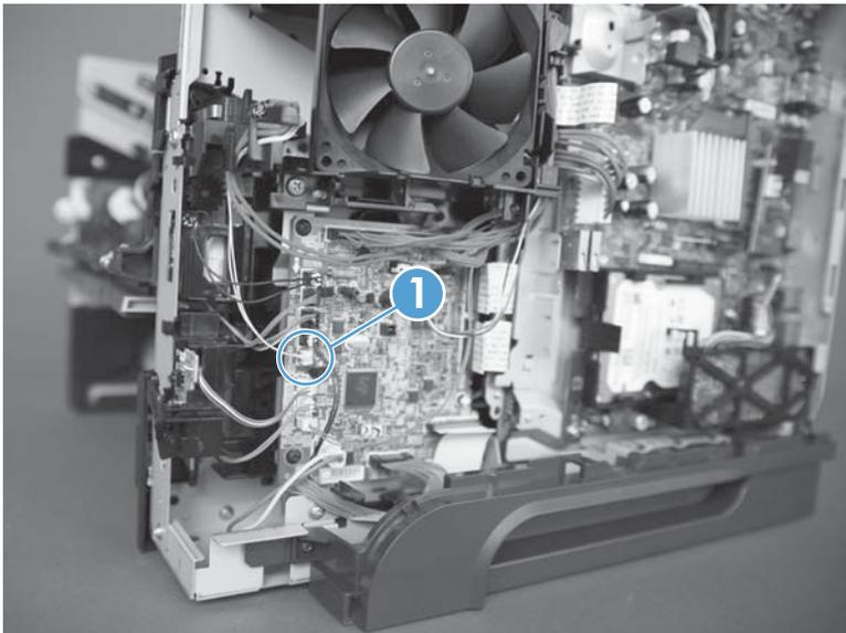
3. Remove one screw (callout 1), and then carefully remove the interlock switch assembly.
