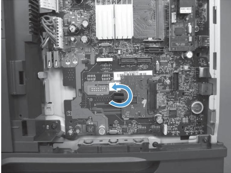
5. Slide the SSM toward the edge of the formatter to remove it.
