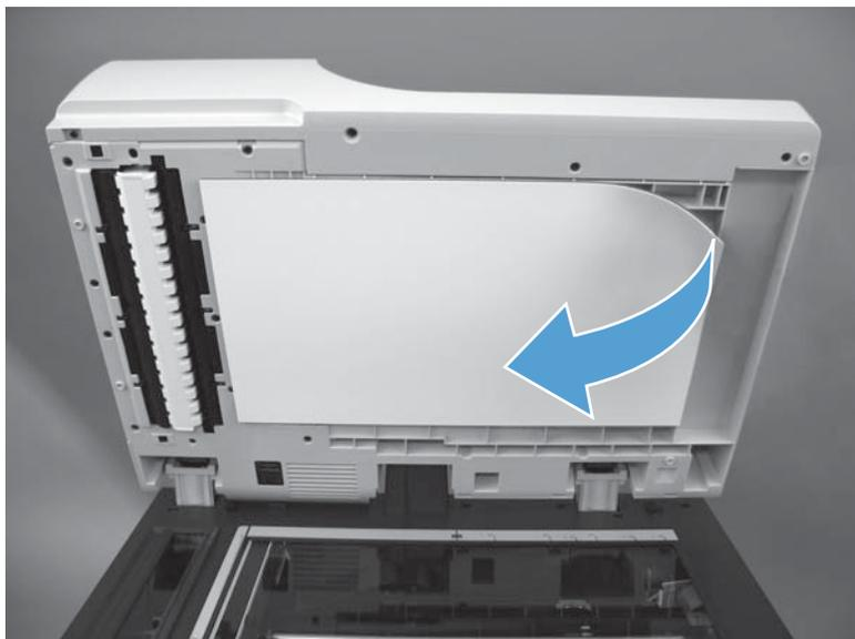
3. Remove any debris from the foam reflector.
