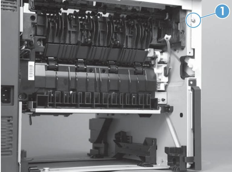
3. Grip the cover and pull it away from the engine. Release the first tab (callout 1), and then release the second tab (callout 2). Release the third tab (callout 3) if necessary to separate the cover from the engine.
