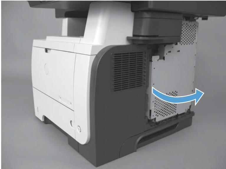
3. Lift and remove the sheet-metal door.
