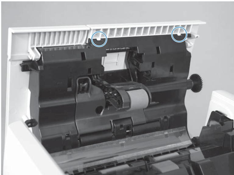
5. Close the ADF jam access cover, and then release the remaining three tabs and remove the cover.
