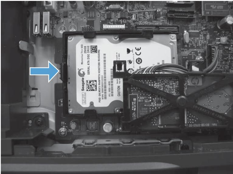
5. Slide the hard disk drive toward the edge of the formatter and remove.
