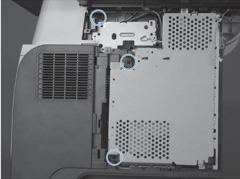
4. Open the formatter cage and remove the sheet metal door.
