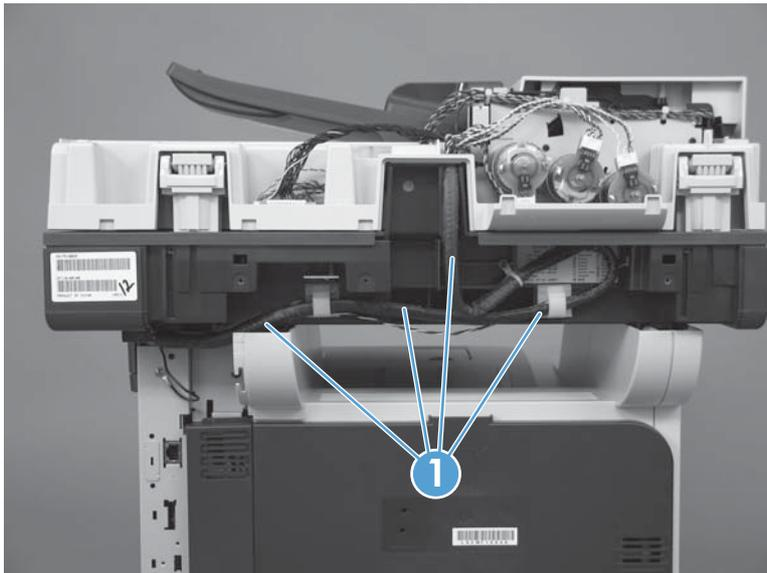
3. Remove two screws (callout 1), release three connectors (callout 2), and cut the tie wrap (callout 3).
