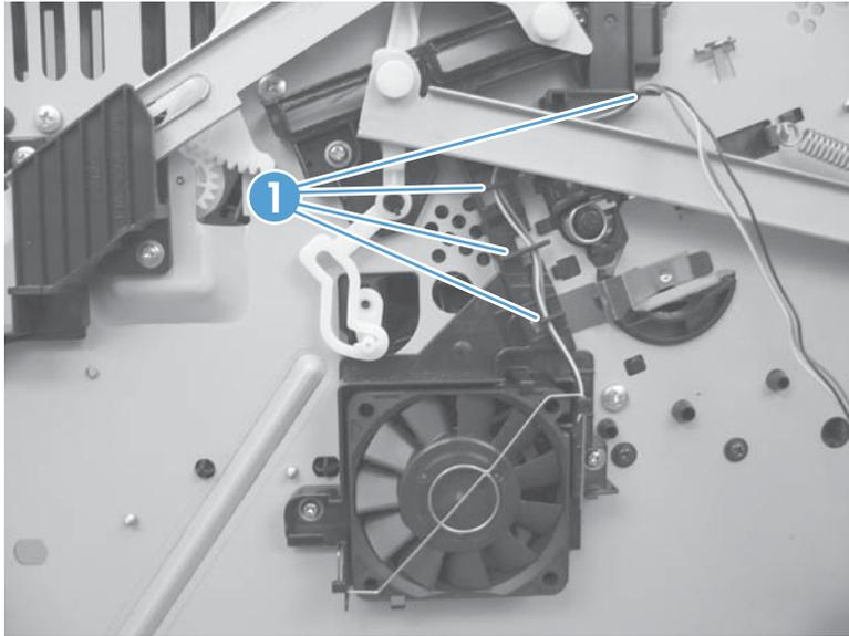
5. **To remove the fan and duct:** Remove two screws (callout 1), and then carefully remove the fan and duct.
