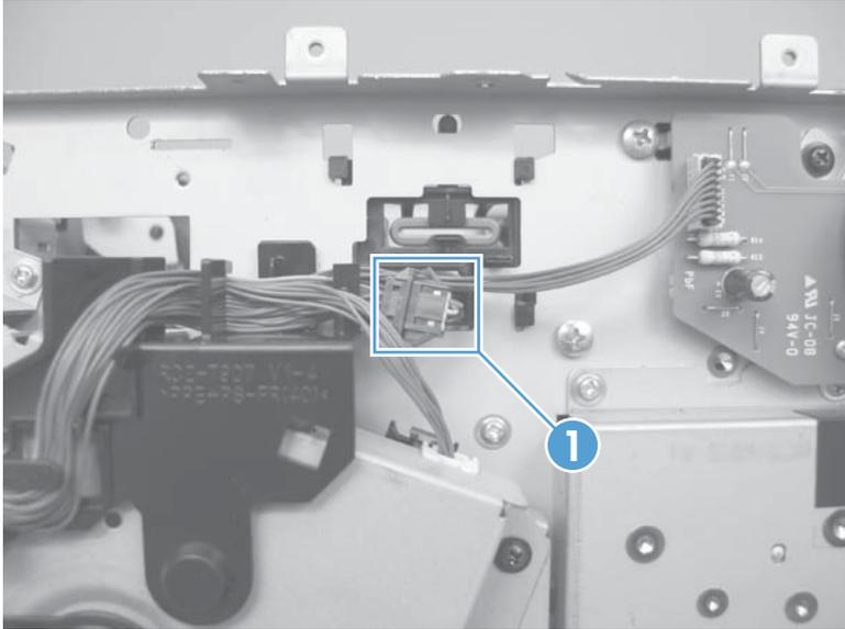
3. Release the wire harness from the retainers (callout 1), and then feed the wire harness through the opening in the chassis (callout 2).
