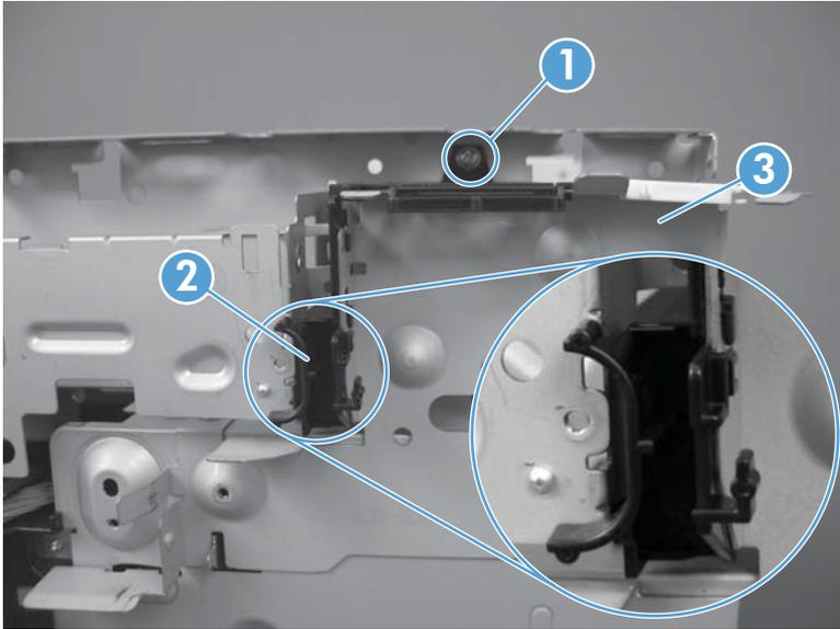
4. Remove two screws and the plastic retainer.
