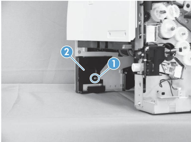
6. Remove one screw (callout 1), release one tab (callout 2) and then slide the guide toward the front of the product to release it. Remove the guide.
