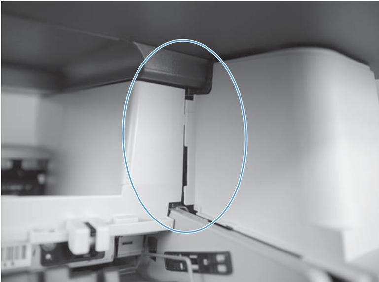
2. Make sure the two tabs are securely inserted.
