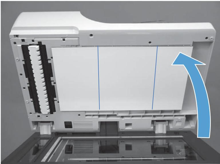
6. Press firmly on the foam reflector to ensure it is securely attached.
