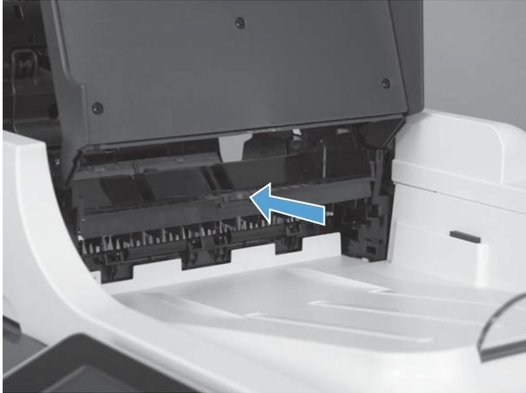
4. Lower the ADF tray, and then lift the separation pad.
