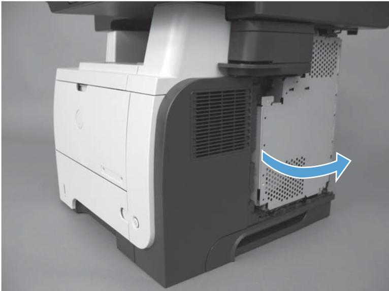
3. Lift and remove the sheet-metal door.
