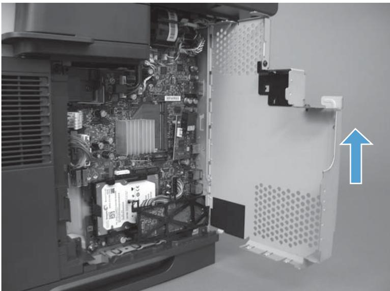
4. Turn the locking tab to release it, and then remove the tab.
