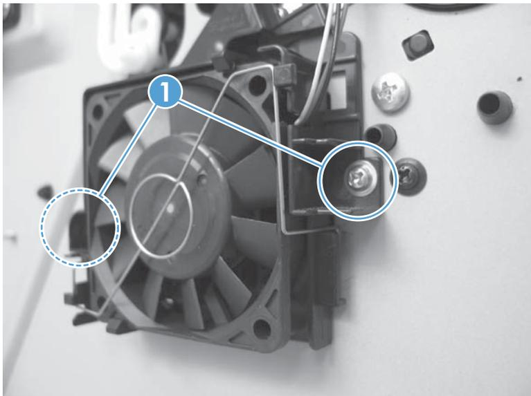
6. **To remove the fan only:** Release the metal static clip, release two tabs (callout 1), and then remove the sub fan.
