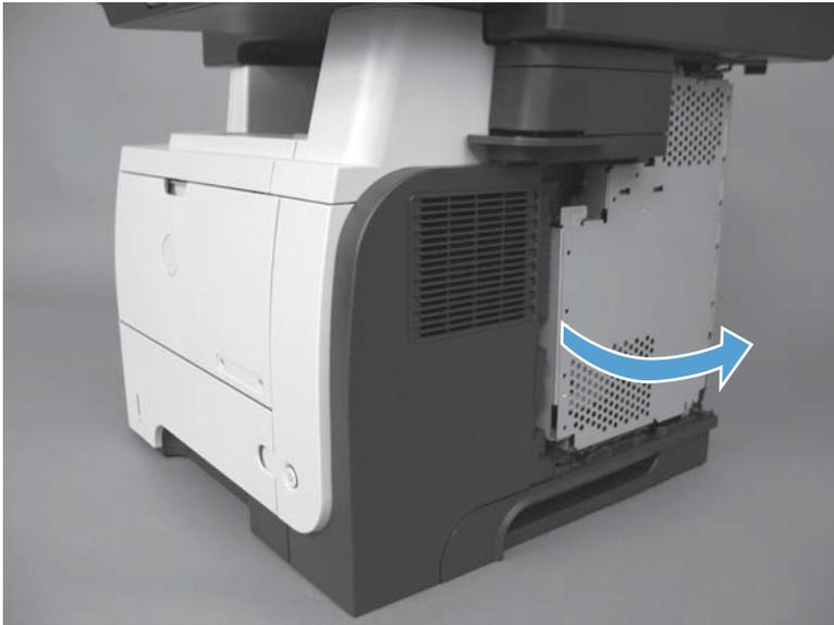
3. Remove one screw (callout 1), release one tab (callout 2) and remove the cover.
