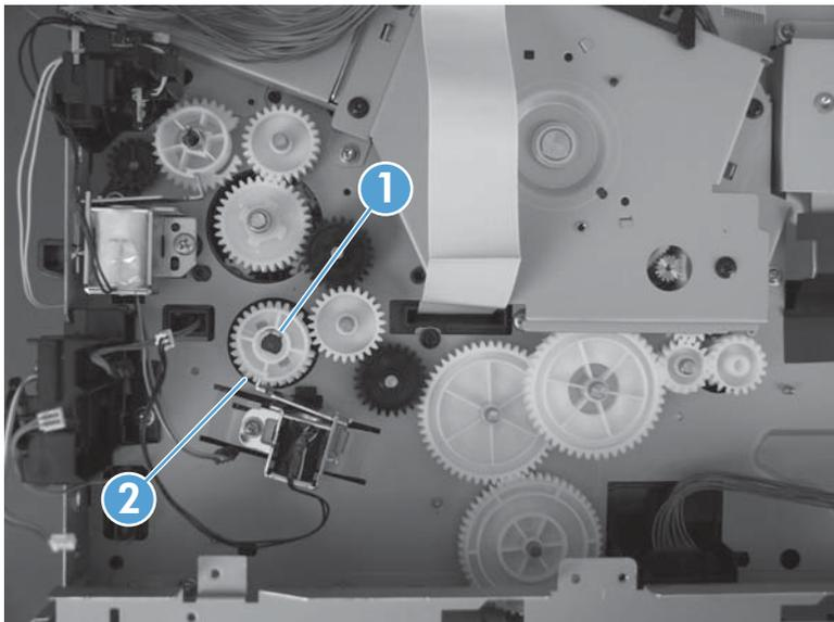
10. Remove two screws (callout 1) and the idler roller assembly (callout 2).
