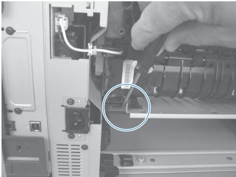
5. Slide the assembly away from the other hinge pin to release it.
