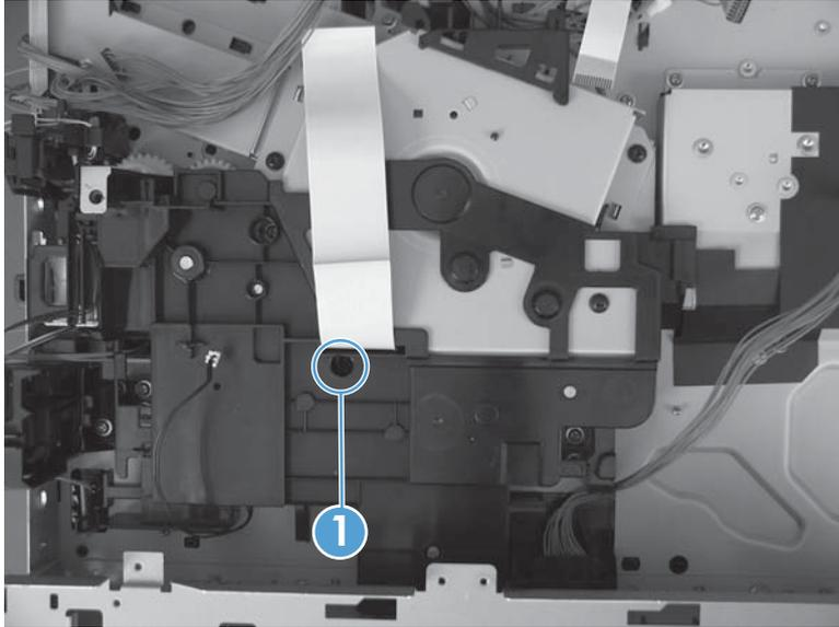
11. Place the product face-side up. Remove two screws (callout 1), and then remove the positioning guide (callout 2).
