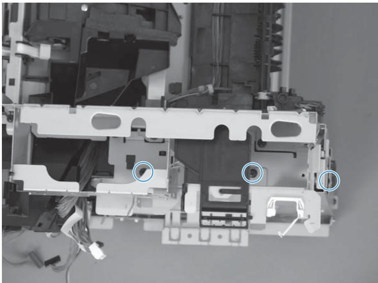
3. Remove one screw (callout 1), the wire harness holder (callout 2), and the sheet-metal bracket (callout 3).
