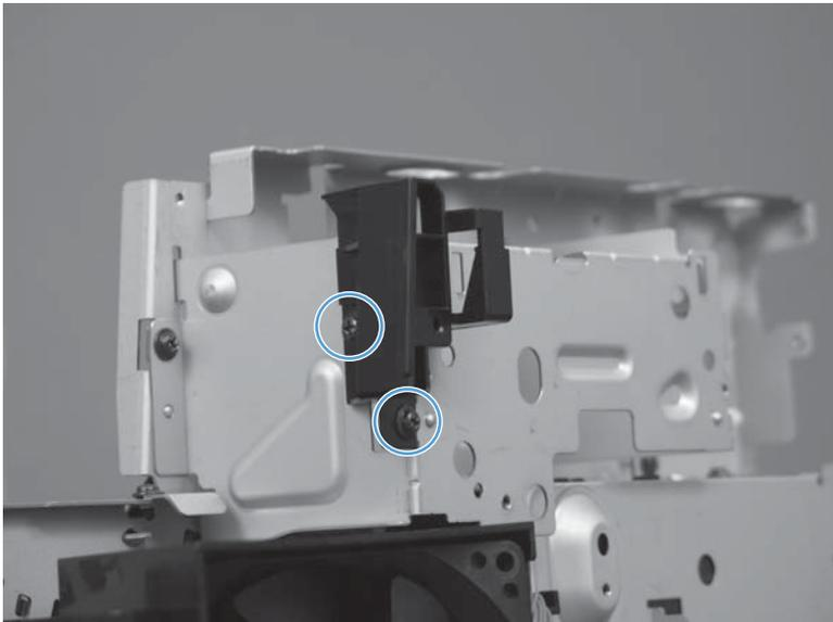
5. Remove two screws and the sheet metal bracket.
