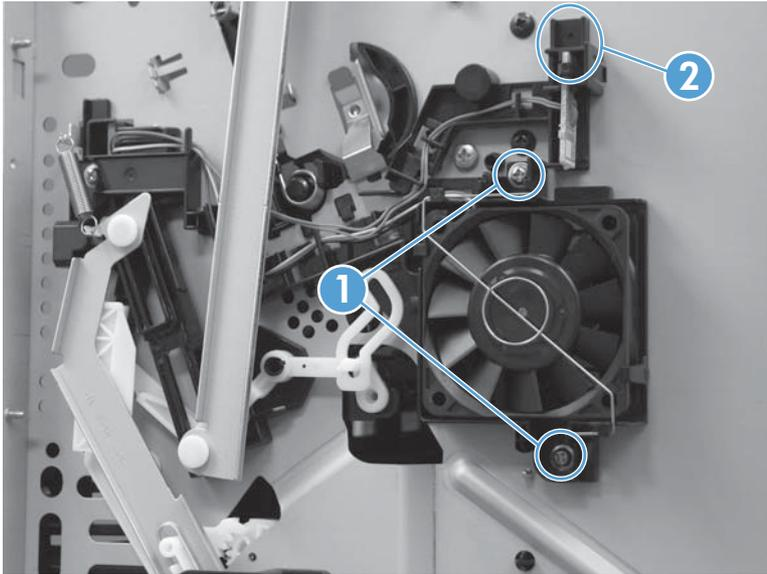
9. Remove two screws (callout 1), and then disconnect one connector (callout 2).
