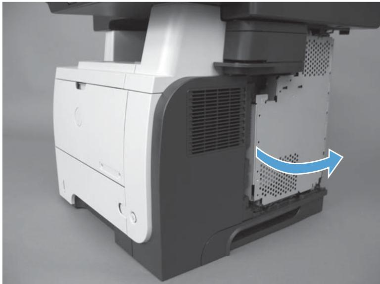
3. Lift and remove the sheet-metal door.
