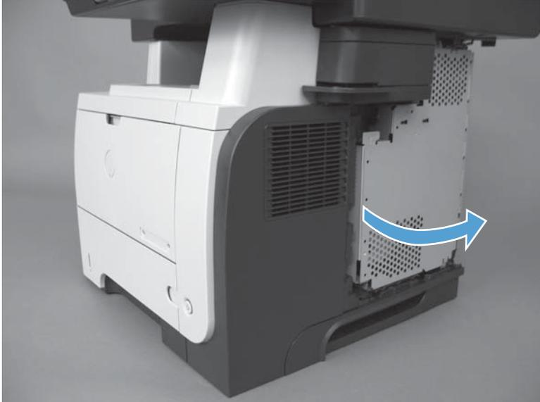
3. Lift and remove the sheet-metal door.
