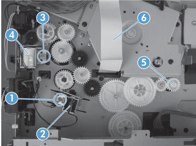
**TIP:** Thread the FFC (callout 6) through the gear cover when reinstalling and make sure to reinstall the gear (callout 5) if it becomes dislodged.
