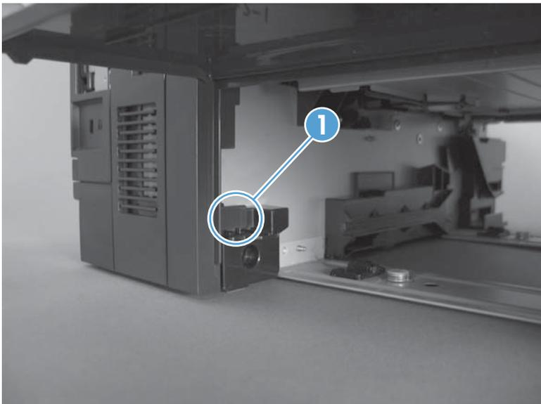
7. Rotate the bottom of the rear cover assembly away from the product.
