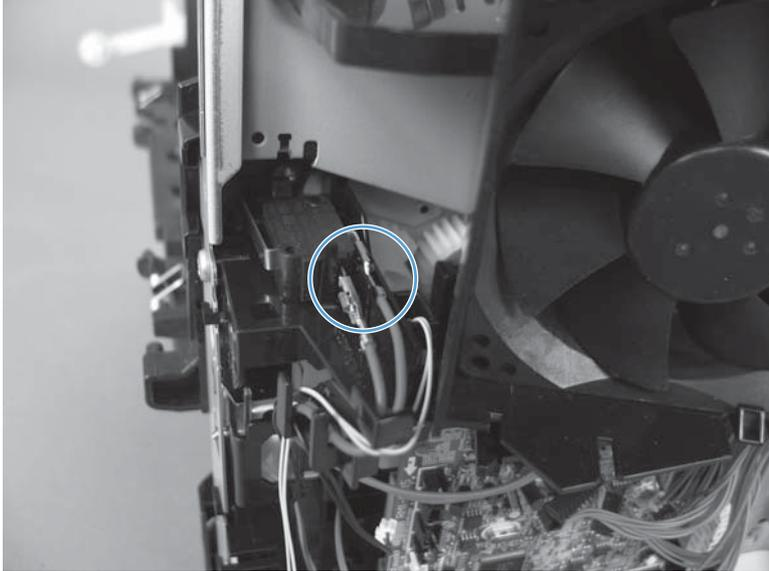
**Figure 1-192** Remove the DC controller (3 of 6)
