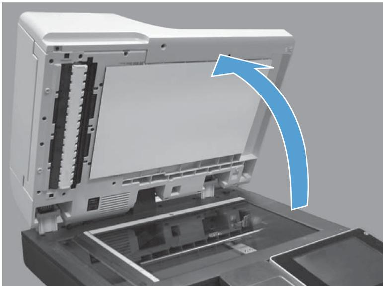
2. Carefully peel the foam reflector from the ADF.
