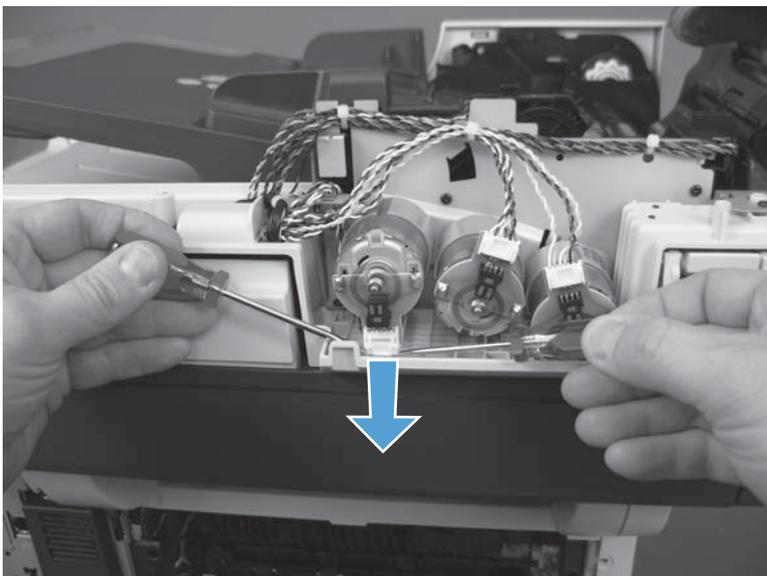
5. Remove two screws (callout 1) and then release the ADF cable from its retainers (callout 2).
