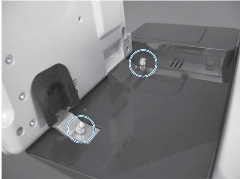
4. Slowly slide the control-panel assembly away from the product to release it. Lift the control-panel assembly to reveal the connectors.
