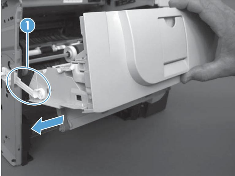
4. After releasing from the hinge pins, move the cartridge door to the right to release the pressure on the link arm. Rotate the assembly down, and then separate the link arm (callout 1) from the assembly. Remove the cartridge-door assembly.
