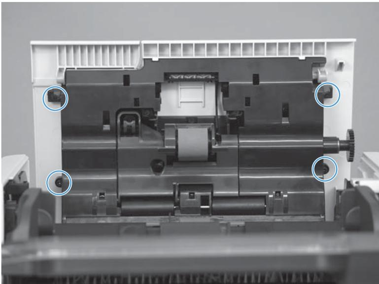
3. Before removing the cover, note the location of the tabs.
