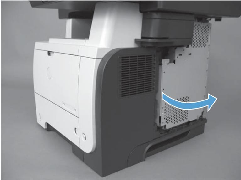
3. Lift and remove the sheet-metal door.
