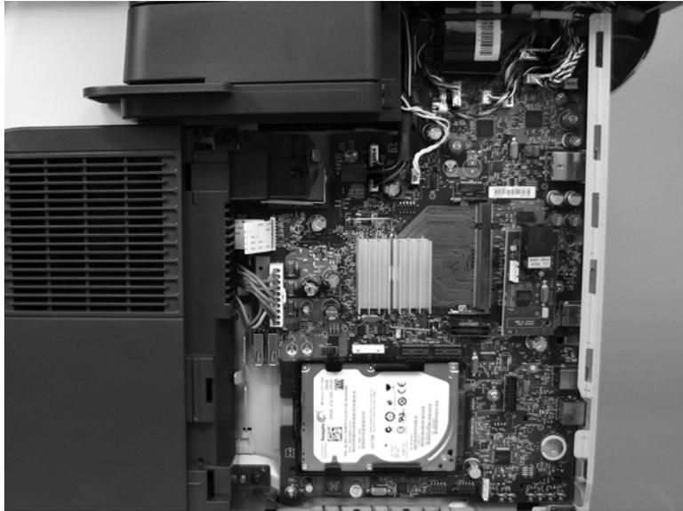
5. Remove five screws and then carefully remove the formatter PCA.
