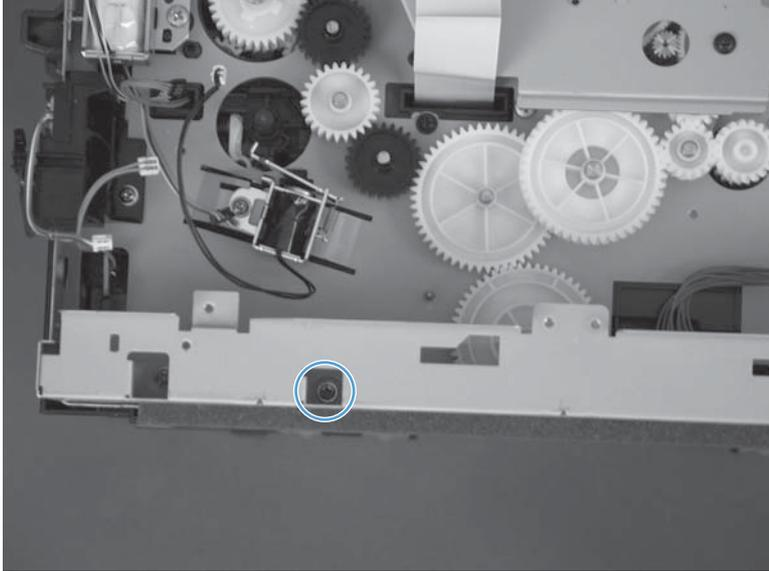
3. Remove one screw (callout 1), and then remove the base plate (callout 2).
