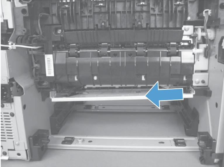
6. Pull the duplex media-feed assembly out of the back of the product.
