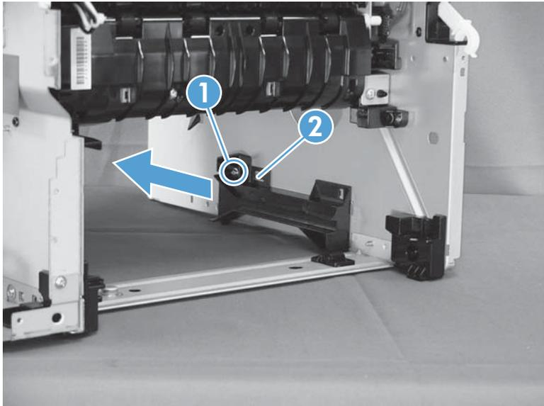
8. Remove two screws (callout 1) and release one tab (callout 2). Let the sub fan and environmental sensor hang from their wire harnesses.
