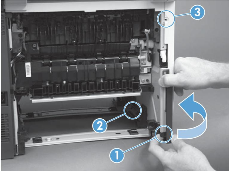
4. Rotate the rear of the cover slightly away from the product, and then slide the cover toward the front of the product to remove it.
