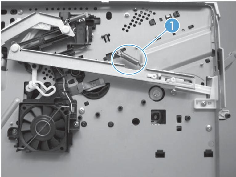
3. Open the cartridge door slightly and then slide the assembly toward the left side of the product to release it from the hinge pins.
