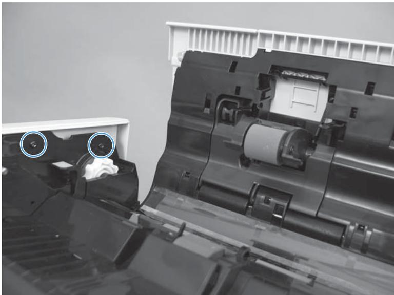
3. Open the ADF, and then remove four screws.
