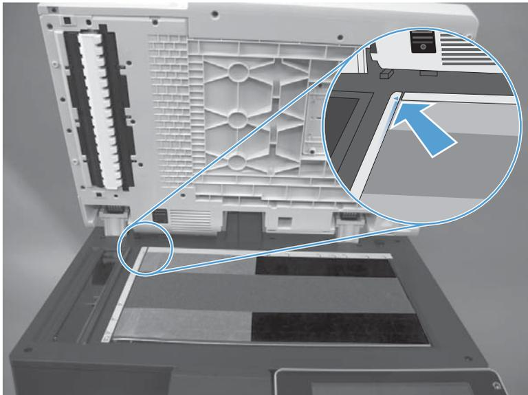
4. Close the ADF lid to attach the foam reflector.
