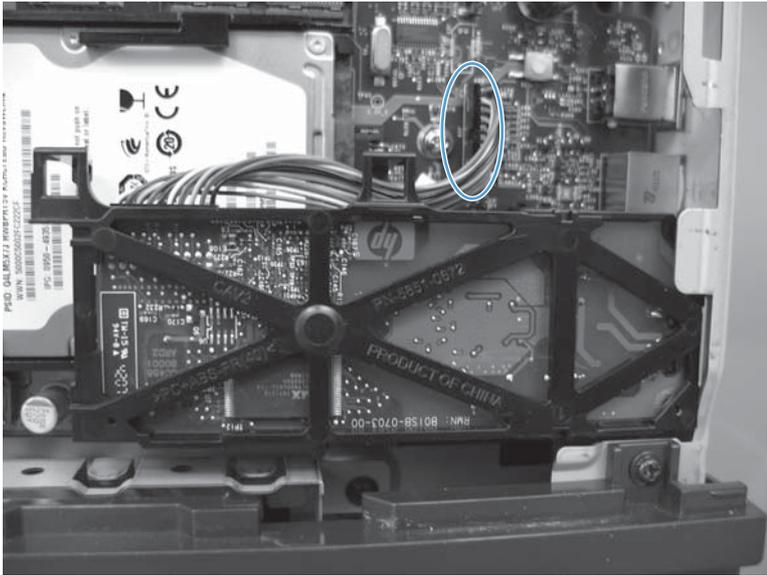
5. Press three tabs to release the fax card, and then remove the fax card from the product.
