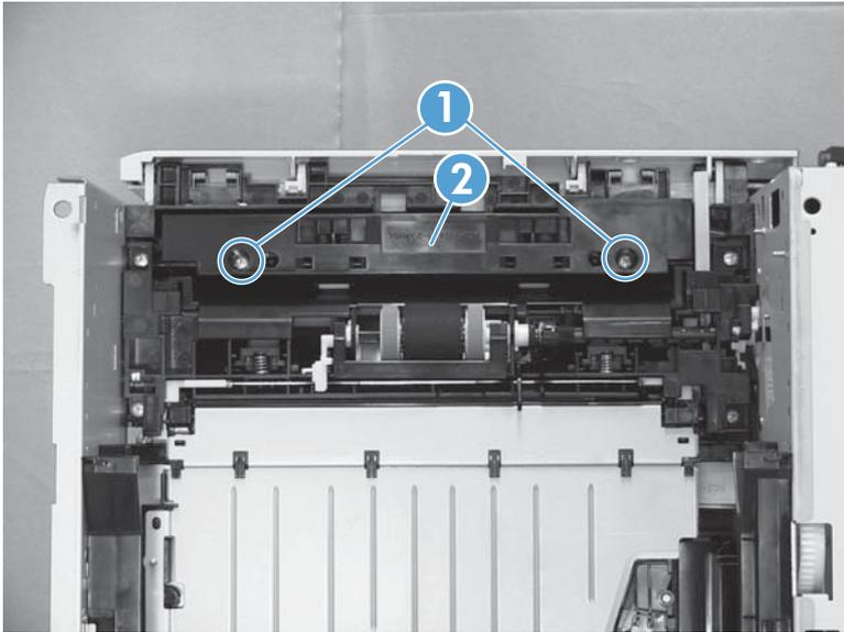
11. Remove four screws and the Tray 2 paper pickup assembly. Rotate the left side of the assembly away from the product first and then remove the right.
