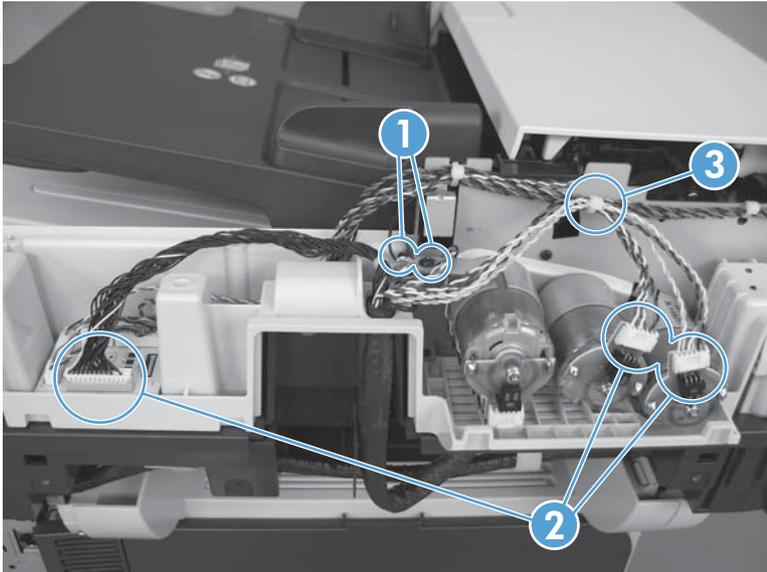
4. Carefully disconnect one connector. Use needle nose pliers or two small screwdrivers to disconnect.
