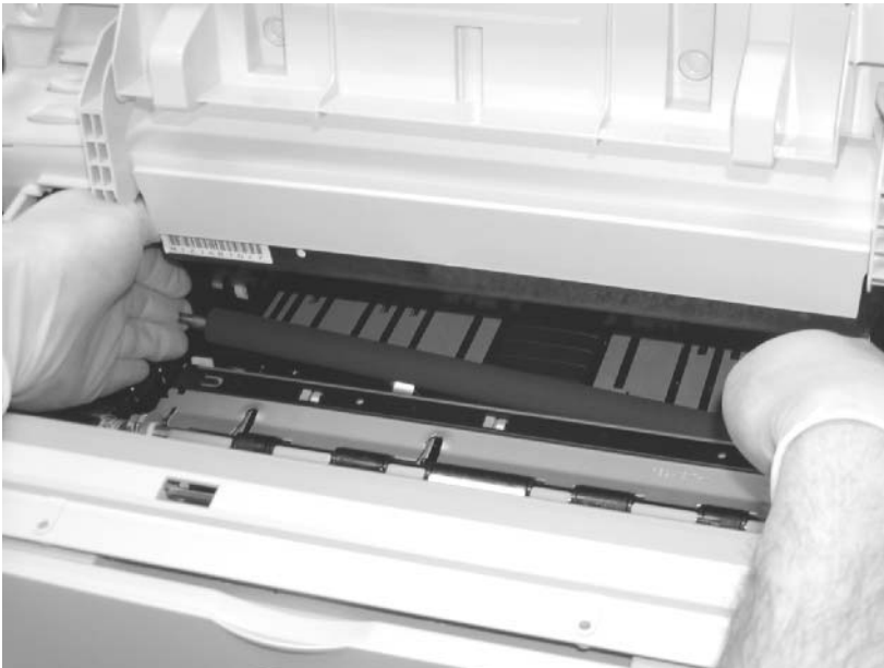
Transfer-roller assembly removal (3 of 3)
