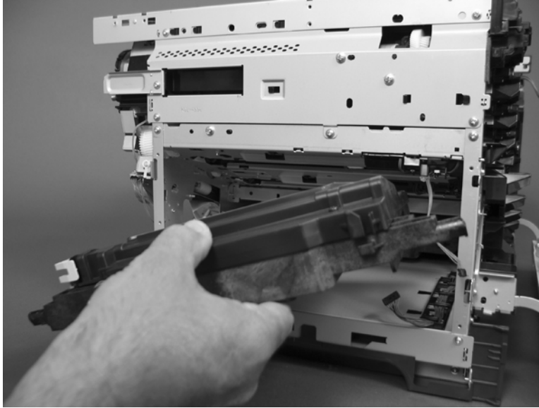
Figure 6-242 Remove the laser/scanner assembly (Y/M) (12 of 12)
