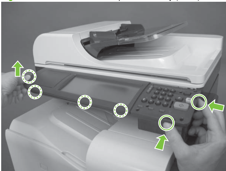
Figure 6-58 Remove the control-panel assembly (1 of 3)
