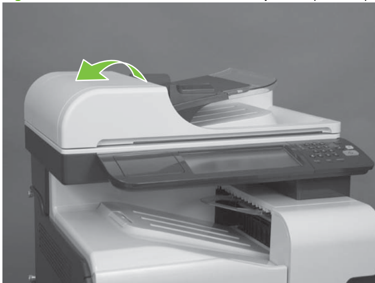
Figure 6-50 Remove the ADF roller assembly and separation pad (1 of 5)
