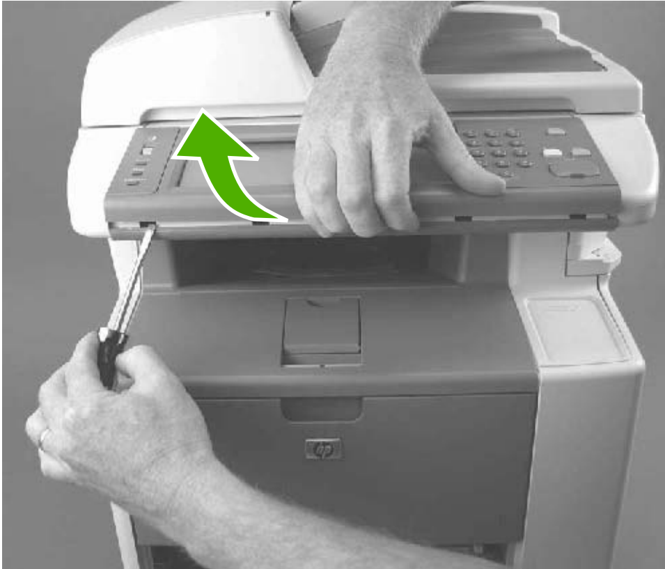
Figure 5-6 Removing the control panel (1 of 2)
