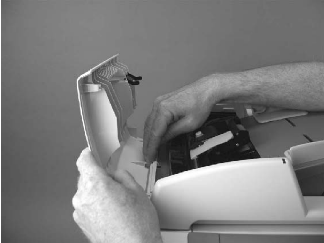
Figure 5-3 Reinstalling the ADF cover
