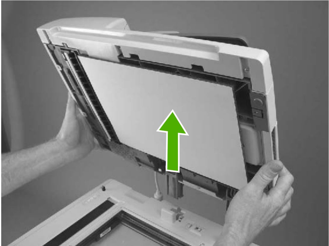
Figure 5-11 Removing the ADF (3 of 3)
