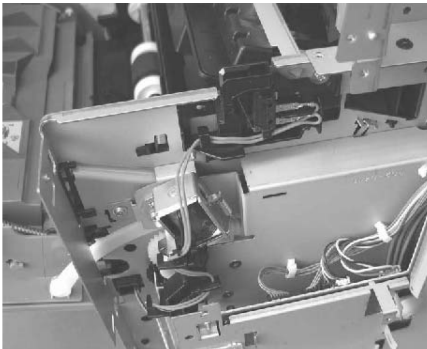
Figure 5-57 Reinstalling the front-door microswitch cable
