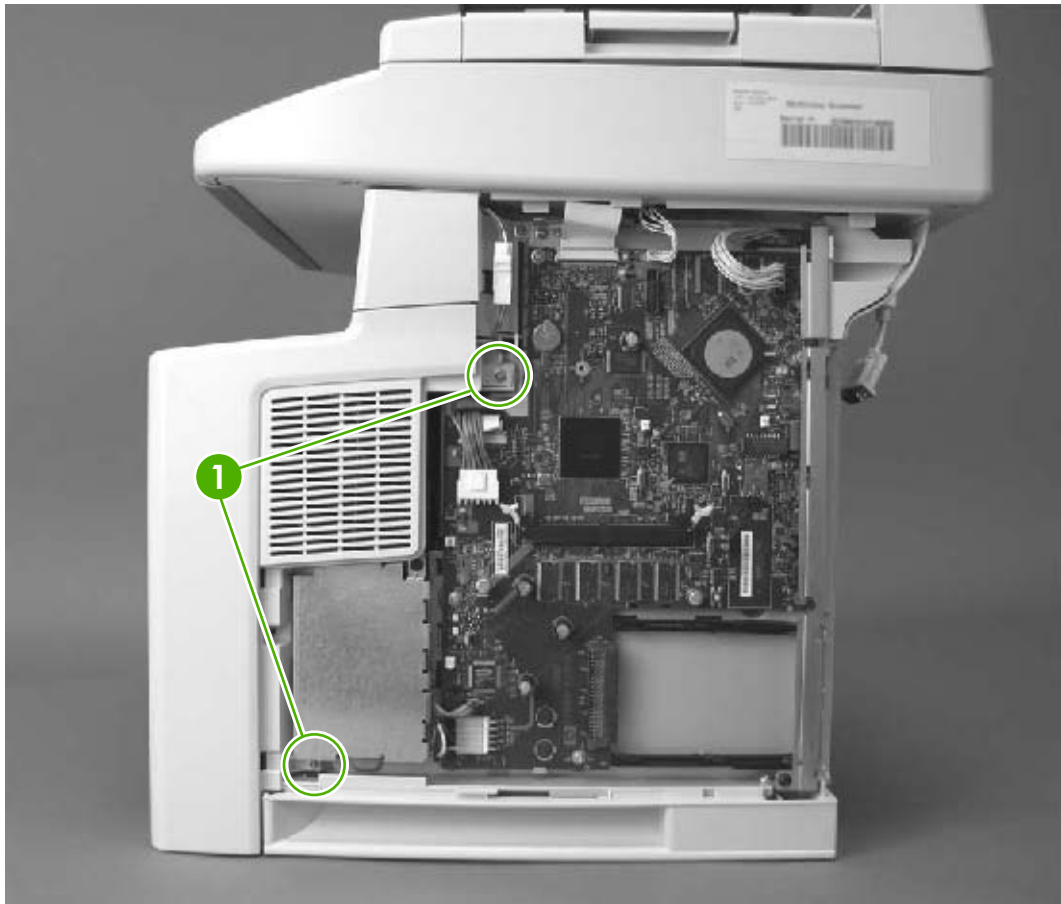
Figure 5-30 Removing the front, right cover (1 of 2)
