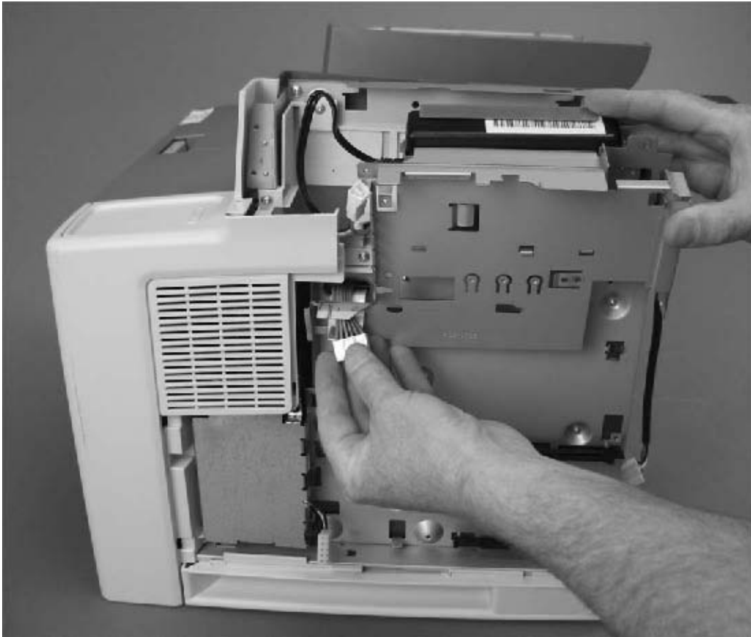
Figure 5-47 Removing the stapler power supply (4 of 5)
