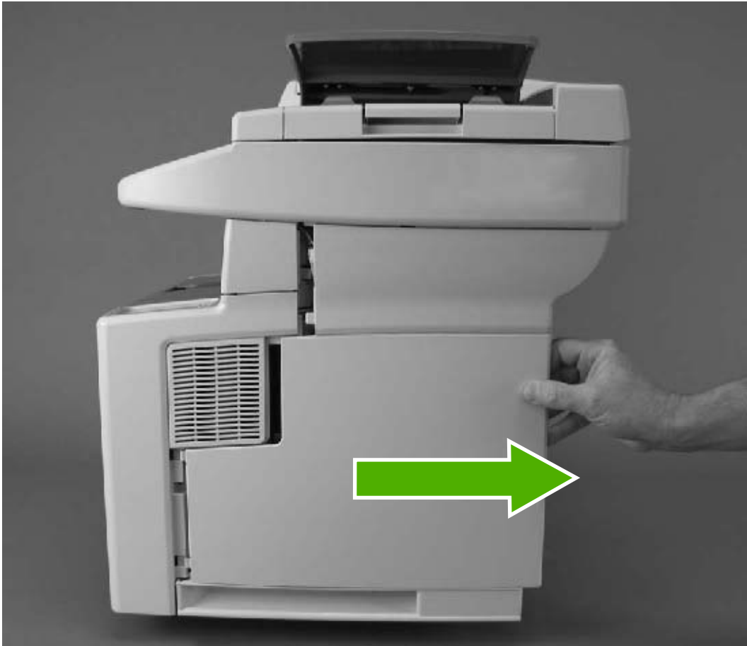
Figure 5-16 Removing the right-side cover
