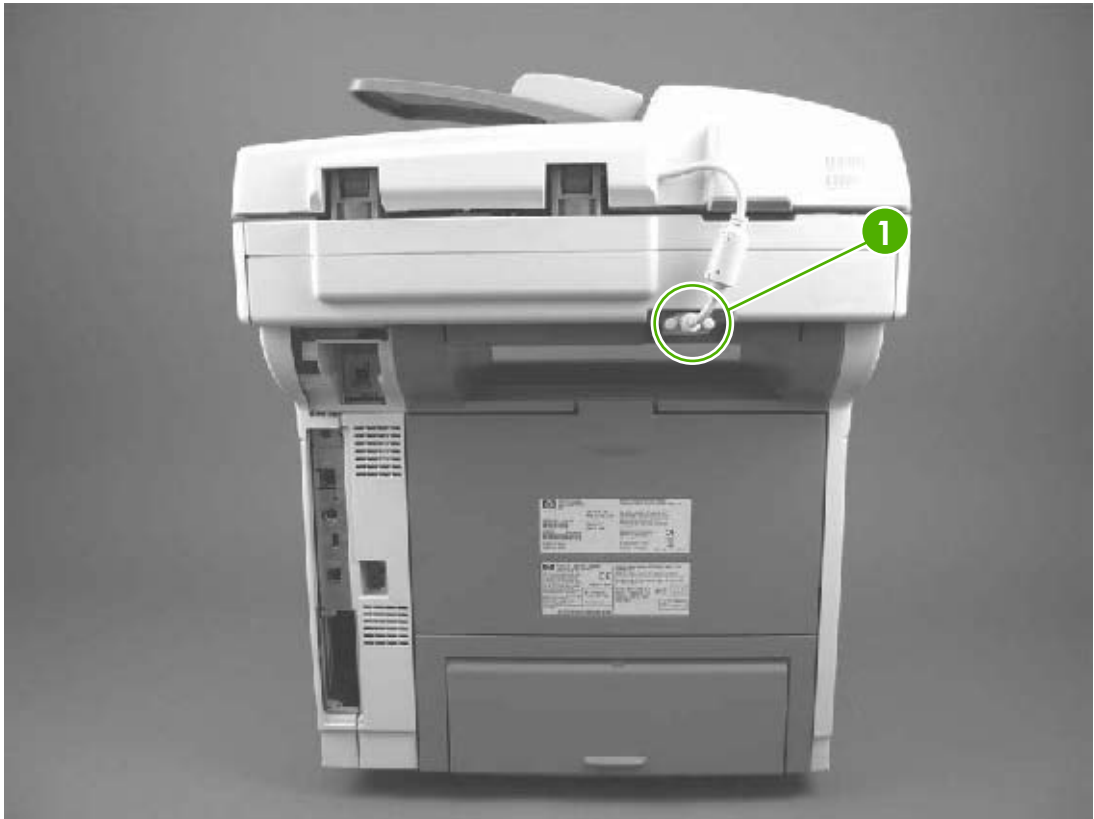
Figure 5-9 Removing the ADF (1 of 3)
