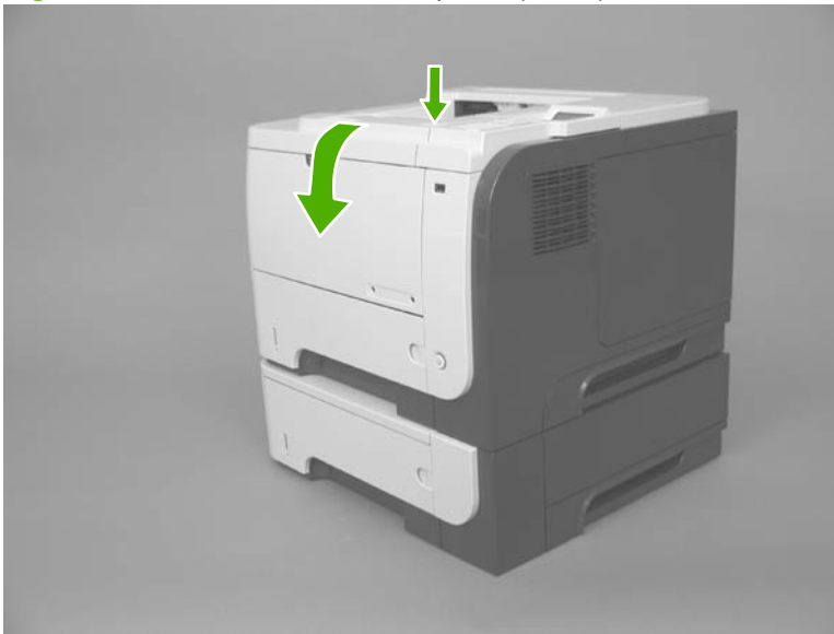
Figure 2-42 Remove the control panel (1 of 4)
