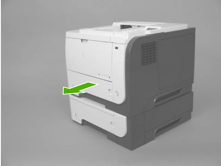
Figure 2-6 Remove the tray cassette (1 of 2)
