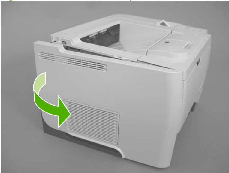
Figure 2-31 Remove the left cover (4 of 4)
