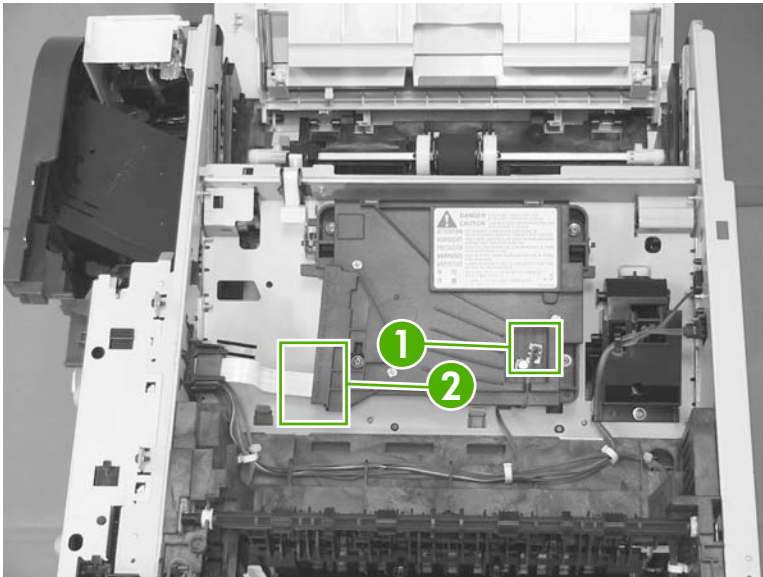
Figure 2-95 Remove the laser/scanner (3 of 5)
