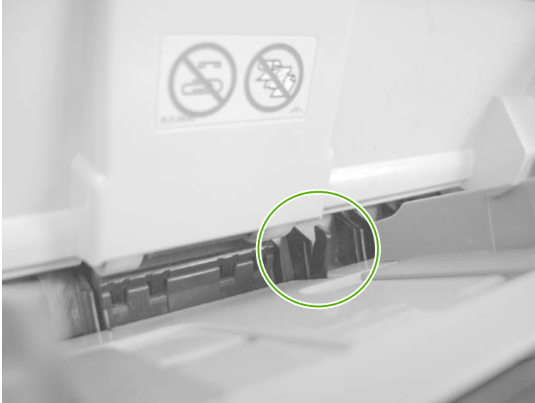
Figure 3-14 Test the Tray 1 (multipurpose tray) media-presence sensor
