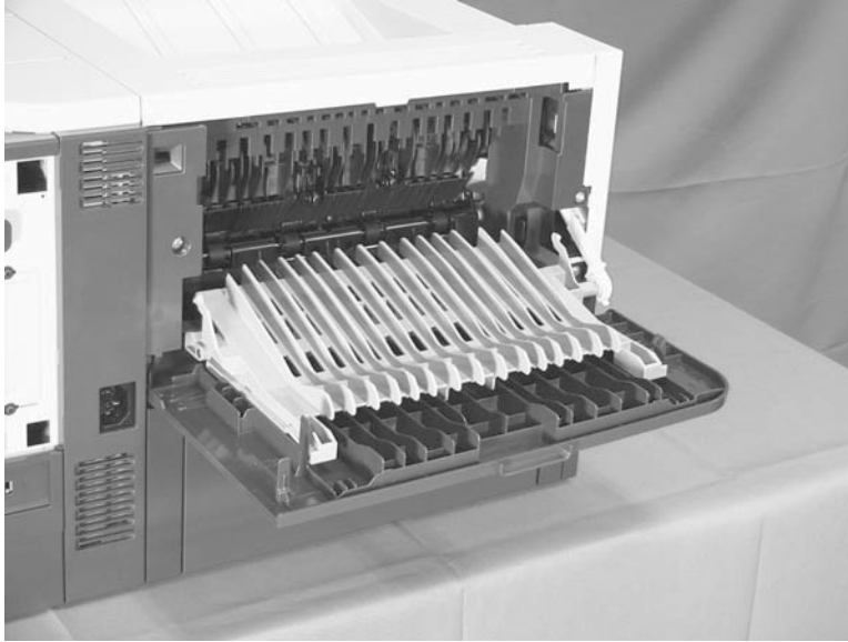
Figure 3-13 Test the face-up detect sensor (2 of 2)
