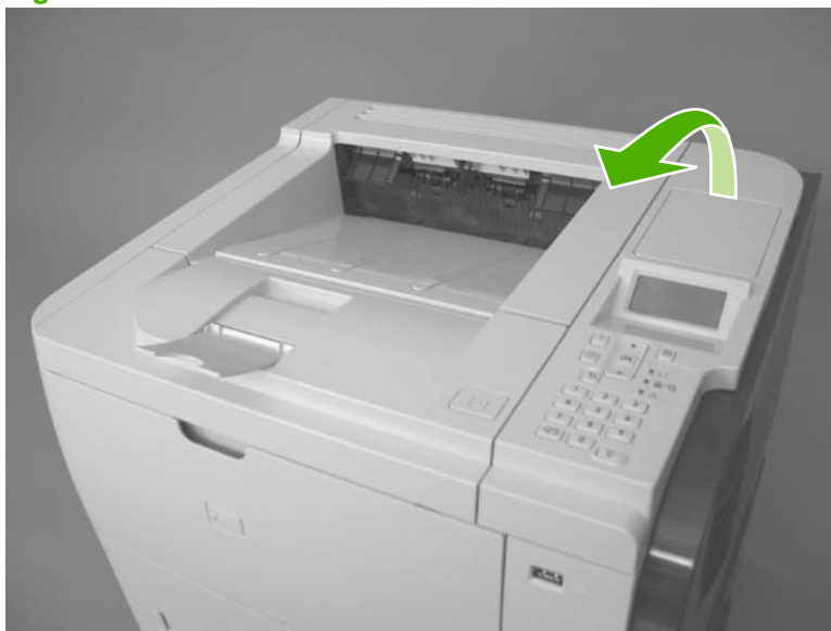
Figure 2-8 Remove the sub cover
