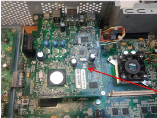
4. Remove the two screws shown.
