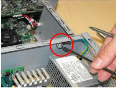
6. Remove the power supply unit.
