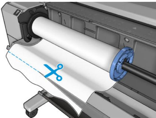
8. Remove the paper left in the printer.
