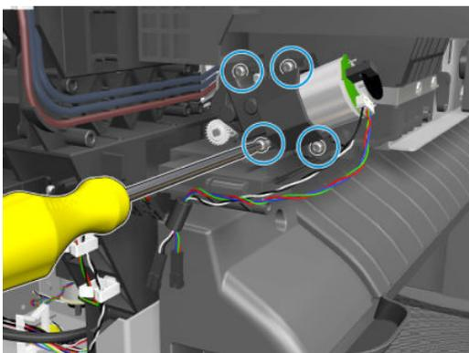
4. Remove the ramps motor.
