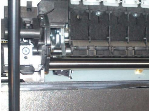
4. Remove the circlip.
