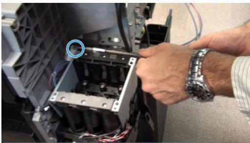
7. Remove the service station. See [Service Station with Drop Detector on page 309](#).
