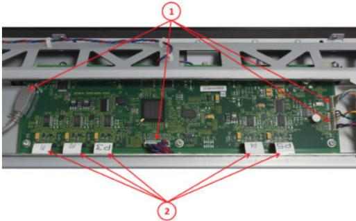
4. Remove the Screws (Torx 10), and remove the Scanner Controller Board.
