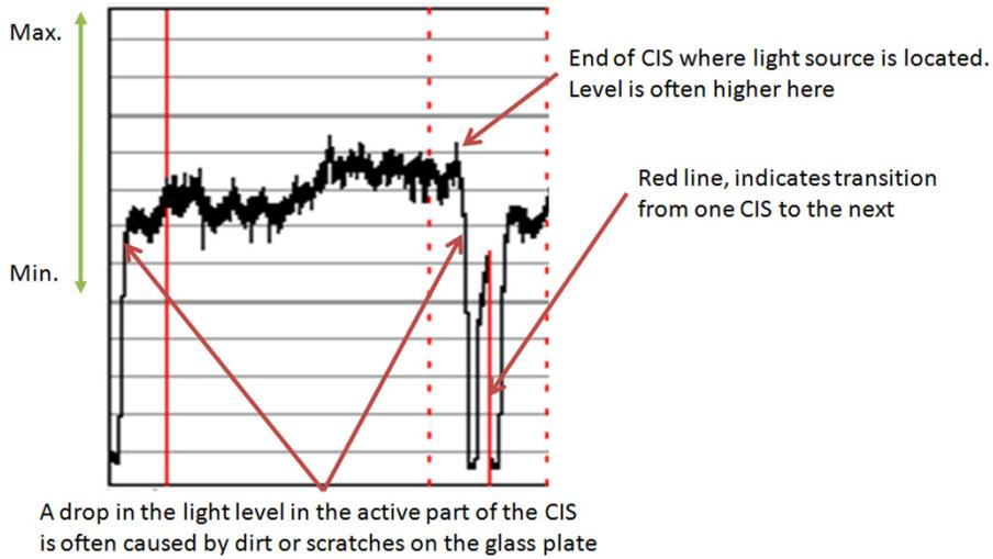
A white patch is located at each end of the CIS element. The one at the start of the CIS is a bit smaller than the one at the end, it makes a black point, unlike the end which makes a Black and a White point.
