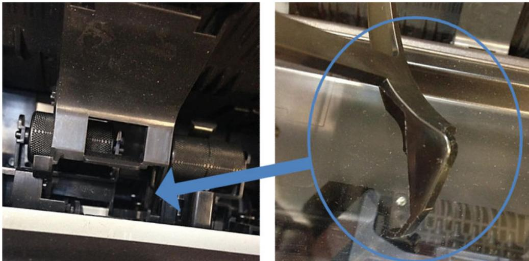
The right pin of the stacker wheel lifter for MFP must slide into the groove shown by the blue arrow.
