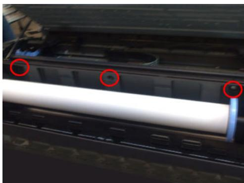
5. Unhook the 2 hooks, and remove the bumper.
