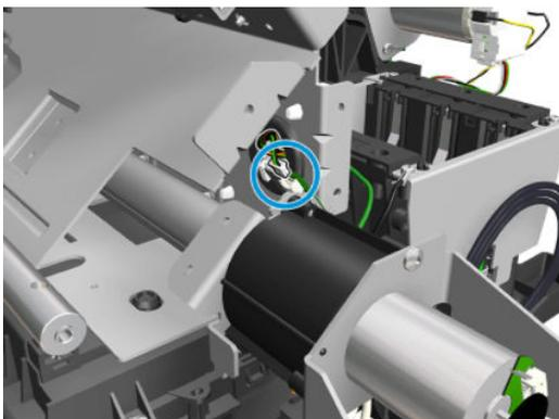
11. Rotate, unlock, and remove the auto pinch lifter.
