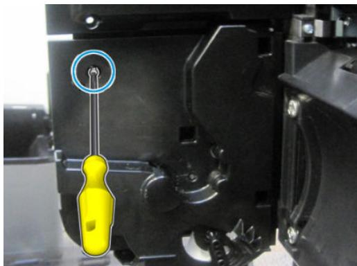
6. Remove 3 T-15 screws and the rewriter.
