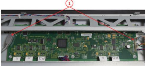
4. Unclip the USB Cable and pull it gently out of the CIS bridge (1). Remove the screws and unclip the cable (2).
