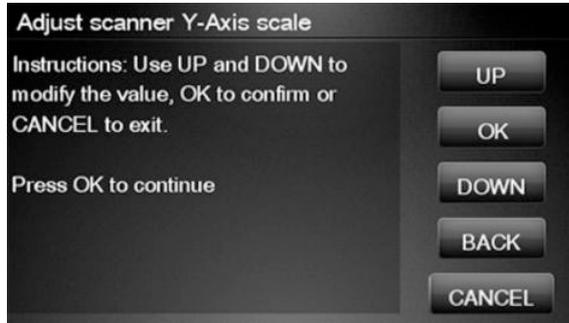
13. Press **UP** and **DOWN** to pre-set the new value of Y-Axis adjustment scale and press **OK**.
