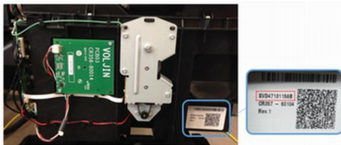
5. Disconnect and take out from route location the encoder cable and motor cable.
