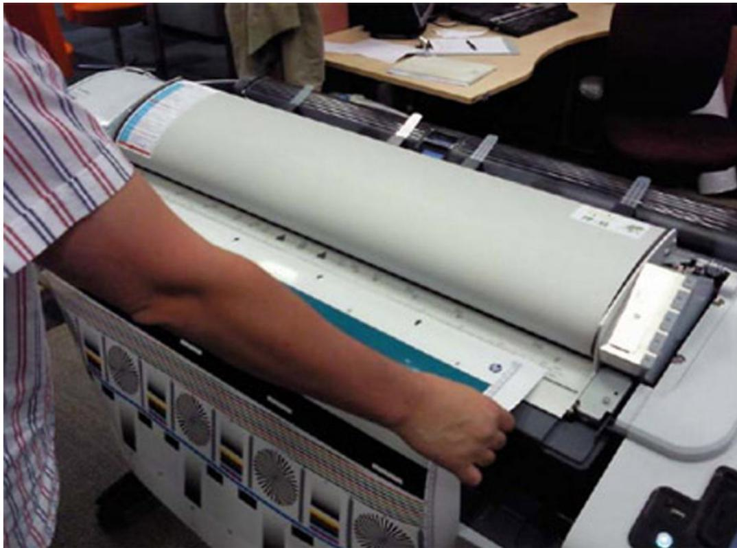
9. Follow the next steps to calculate the Y-Axis adjustment scale: Measure the total length of the two vertical rules at both sides of the copied plot (we call it M1 and M2).
