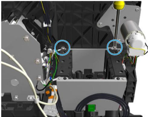
4. Remove the bracket and side plate.
