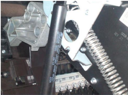
5. Remove the lift assembly. See [Lift assembly on page 422](#).
