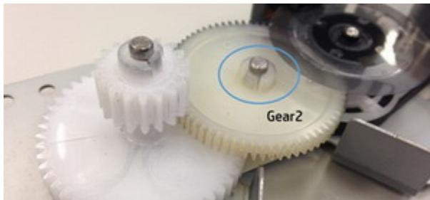
10. Place the tip of the needle in the slot and inject grease until it covers the slot. Repeat this step in both slots.
