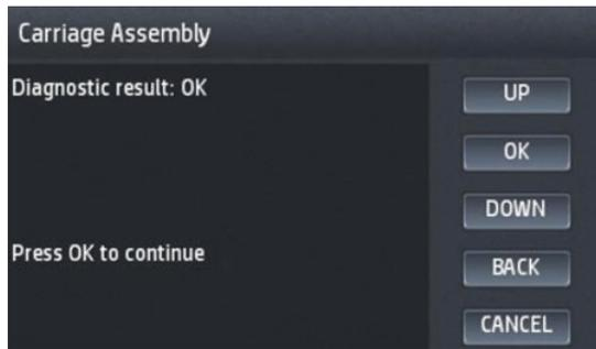
If an error has been found in any of the steps of this diagnostic (parameter values are out of the allowed range; printhead improperly detected or not detected, sensor errors, etc.) the diagnostic test will automatically detect it and stop the test (checks will stop), and the error description will be shown in the front panel. The error description will contain the System Error code (for determining the recovery action) and the specific error cause, if known.
