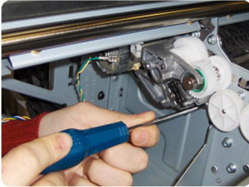
3. Loosen the encoder sensor adjustment screw.
