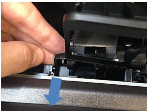
4. Check that the stacker wheel lifter can rotate freely.
