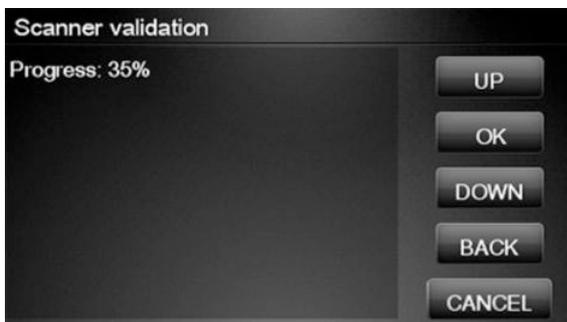
7. Wait until the scanner validation test has completed. The Touch Control Panel will then show the test results. Press OK to continue
