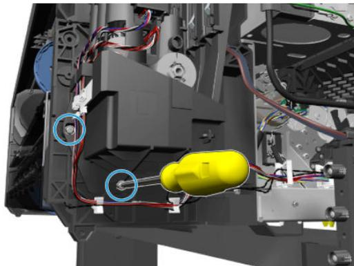
**8. Remove the ISS Front Panel Side.**
