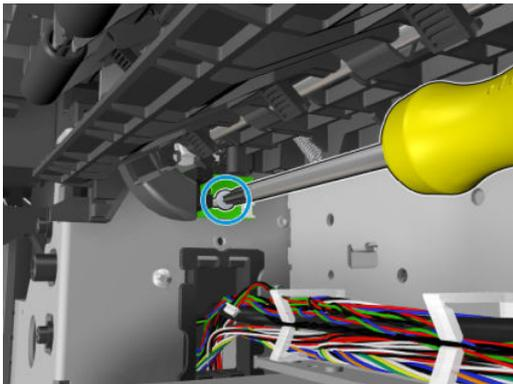
5. Remove the sensor valves.
