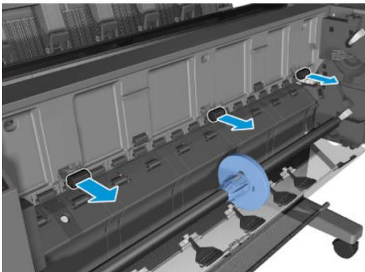
5. Remove the 3 T-15 screws underneath.
