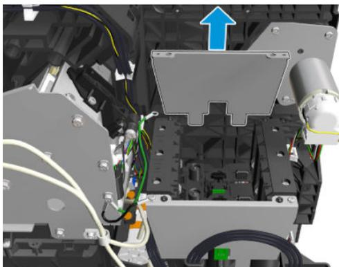
5. Remove 2 screws and the side plate.
