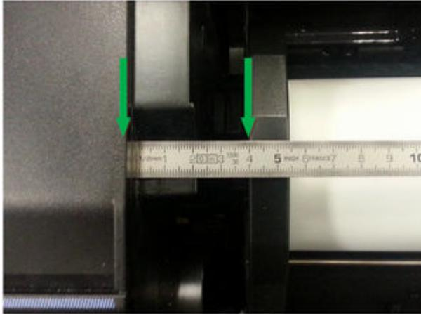
3. If customer is using 36 inch paper roll width, measure distance on the blue hub on the right (as shown in picture below). This distance should be **greater than 4.5 cm** otherwise, the blue hub is probably not completely inserted into the roll core.
