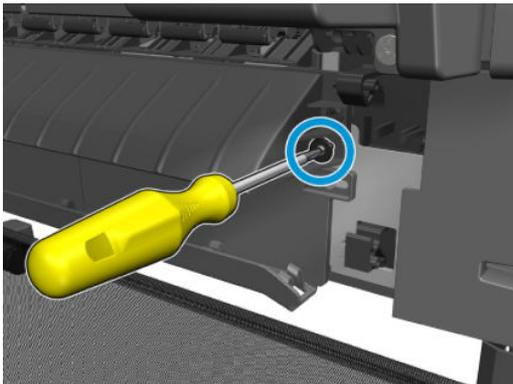
3. Remove the output platen.
