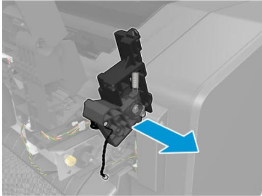
6. Remove the screw and microswitch (sensor).
