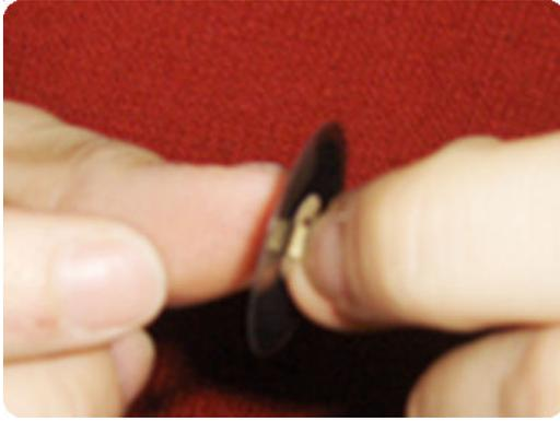
2. Pre-assemble the encoder on the roller without using pressure.
