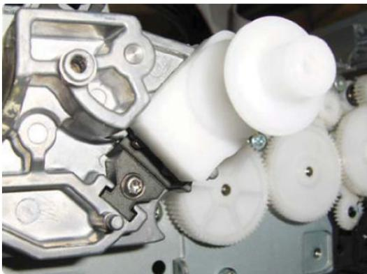
5. Position the Media Advance Drive Adjustment Tool on the end Media Advance Roller shaft, push it firmly onto the shaft and maintain a constant pressure to ensure it is flush to the Media Advance Drive.
