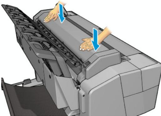
6. Clean the area immediately in front of the scanner, where the scanned sheet rests before scanning.
