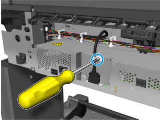
5. Disconnect and unclip the front panel cable.
