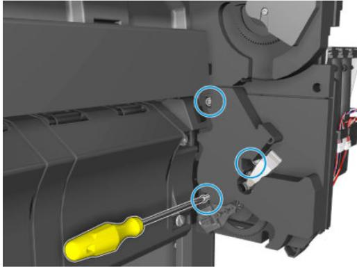
7. Remove the bottom tip support.
