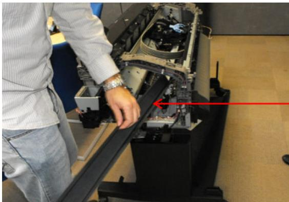
11. Remove 6 screws and the printheads.
