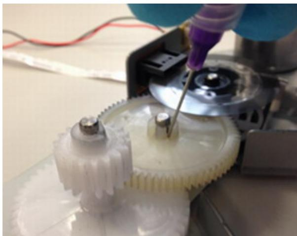
11. Clean the remaining grease with the lint free cotton. After cleaning it should look like in the image below.
