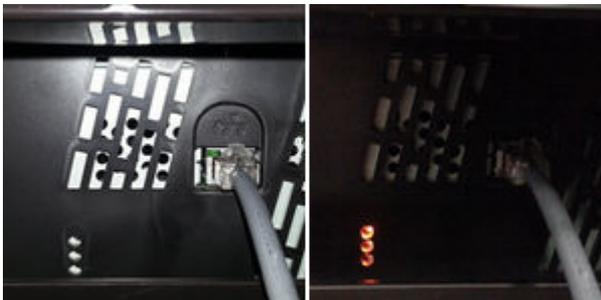
3. Use the following table to interpret the LEDs and find the source of the problem. Remember that you should read these LEDs when you press the power button. Some combinations may require the replacement of more than one component. In this case, always replace one component at a time. Check the LEDs again to see whether the problem has disappeared. If the same LED sequence appears, replace the next component indicated in the table.
