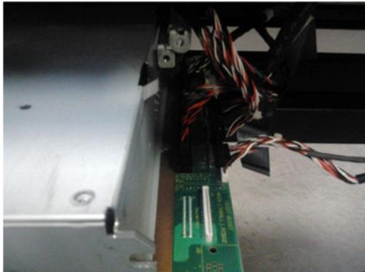
6. Remove the E-Box from the printer.
