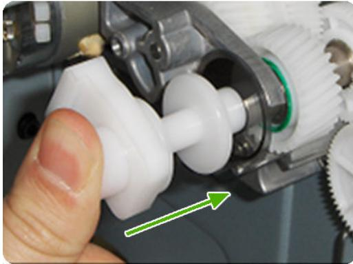
6. While maintaining pressure on the Media Advance Drive Adjustment Tool, fully tighten the three T-15 attachment screws in the order shown.
