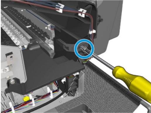
3. Remove the bump cutter actuator.
