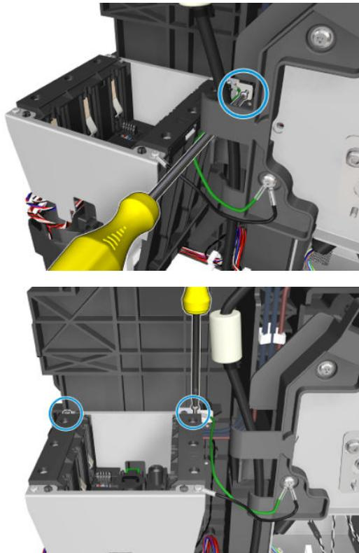
4. Remove the bracket and side plate.
