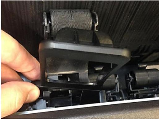
2. Push the stacker wheel lifter's left leg to align the left pin with the left groove.
