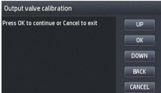
3. The screen will show the 'calibrating status' during some minutes, while the output valve is performing some movements.
