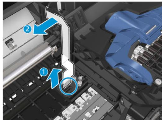
3. Unclip the mylar, and disconnect trailing cable.
