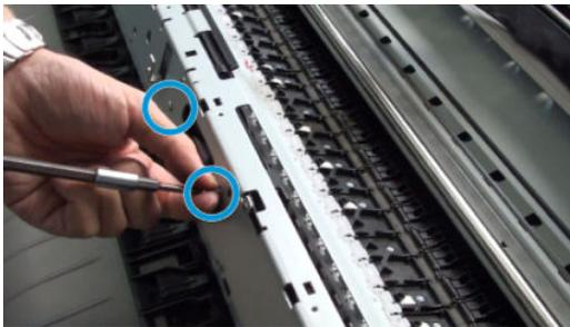
6. Remove the ISSWALL (removing 2 T-10 screws).
