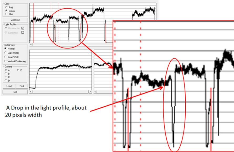
A light profile with an about 20 pixel drop can be a contaminated lens in the CIS module.
