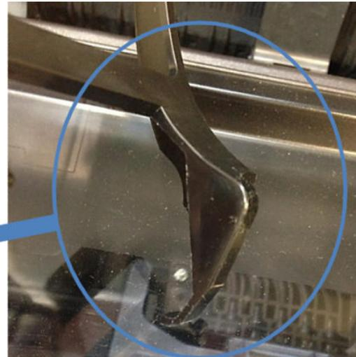
The right pin of the stacker wheel lifter for MFP must slide into the groove shown by the blue arrow.
