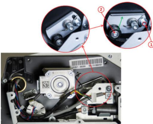
7. Remove the motor screws.
