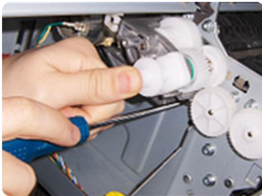
7. While maintaining pressure on the Media Advance Drive Adjustment Tool, fully tighten the encoder sensor adjustment screw.
