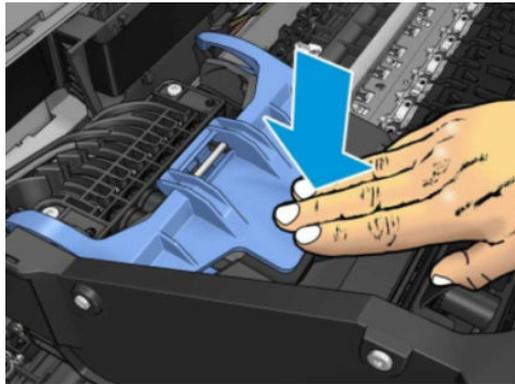
If these two conditions are not met, printhead installation may fail and/or some tubes may not be filled with ink.
