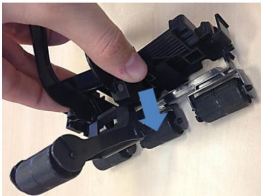
The stacker wheel lifter is now removed from the Hand-off assembly.
