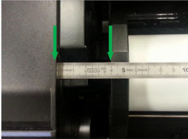
4. If customer is using 36 inch paper roll width, measure distance on the blue hub on the right (as shown in picture below). This distance should be **greater than 4.5 cm** otherwise, the blue hub is probably not completely inserted into the roll core.
