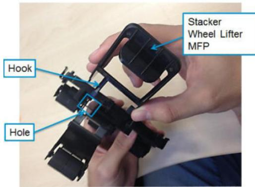
2. Rotate the second wheel holder in order to insert the right and left pin.
