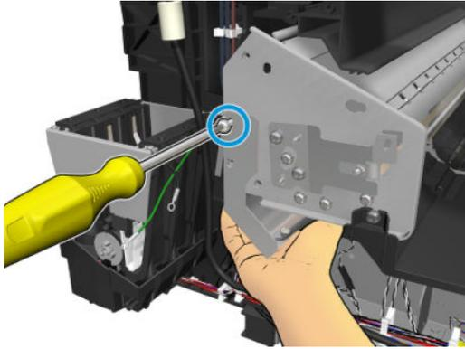
8. Remove the Scan Axis Motor.
