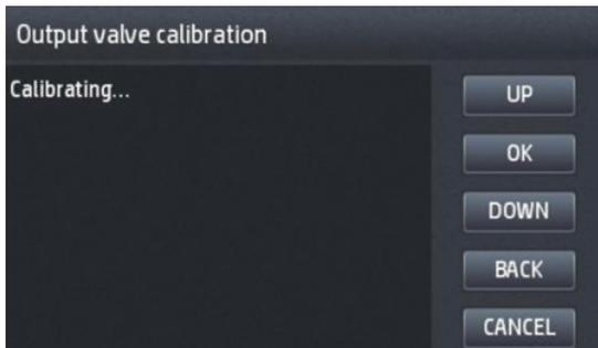
4. At the end of the process, you will have the result of the calibration. The screen will show also a recommendation to verify the calibration (print a plot to stacker). Typical values for the calibration range from 1015 to 1225.
