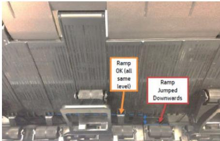
If ramps are not aligned, replace the stacker.
