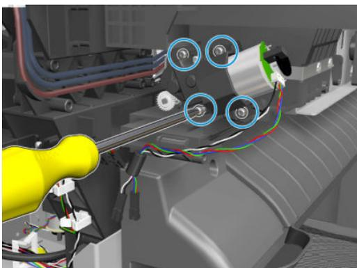
4. Remove the ramps motor.
