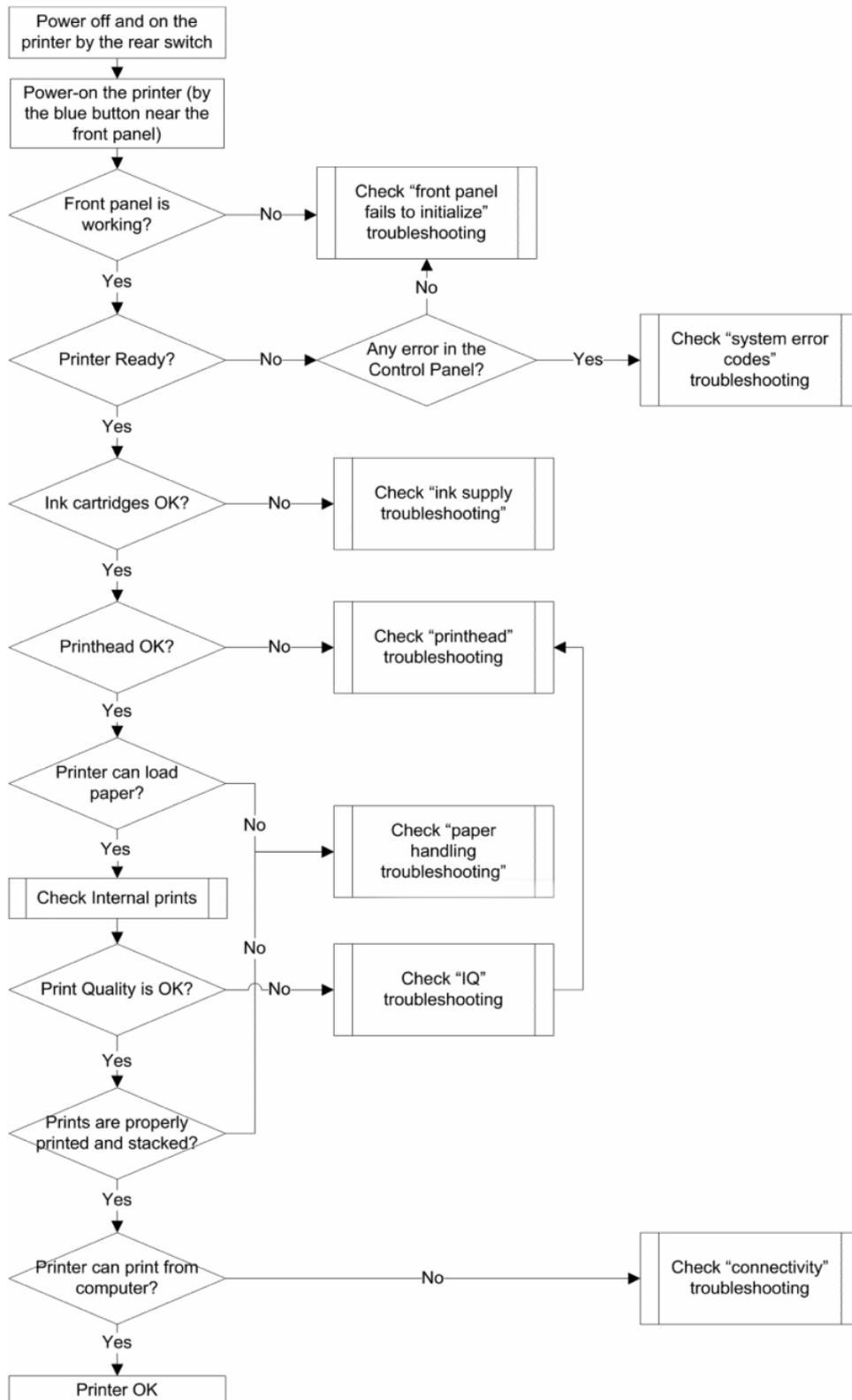
**NOTE:** Once an issue is confirmed, check that printer has latest firmware installed.
