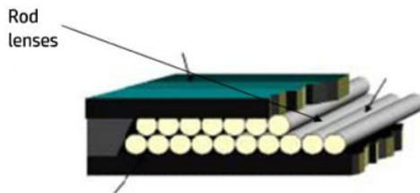
Due to the very short focal length, the focus depth is limited. The original has to be in contact with the surface of the glass plate in order to be in focus.
