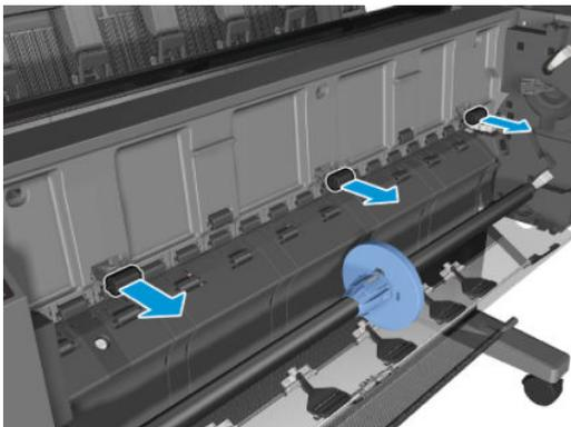
5. Remove the 3 T-15 screws underneath.
