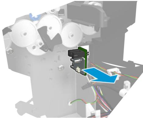
5. Remove the 3 gears.
