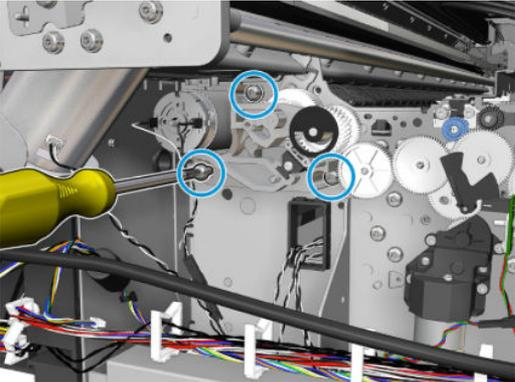
7. Remove the paper axis motor.
