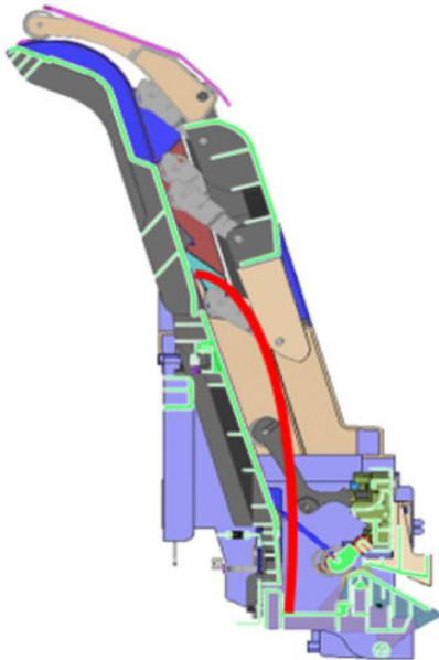
Stacker capacity is defined as up to 50 pages (T920/T1500/T2500), and 100 pages (T3500), A1/D size line drawing plots in landscape on bond media, but stacker capacity depends on media thickness and page size. If you are printing plots shorter than A1 and you experience a reduction in the stacker capacity because they collapse and the curling fills the available stacking space:
