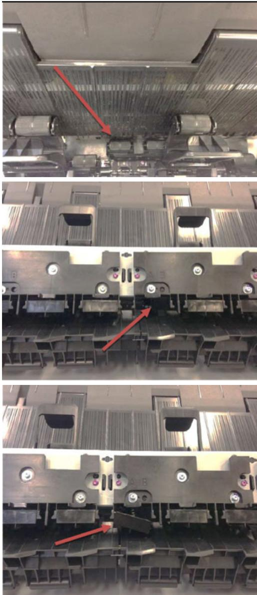
8. Check that Ramps are broken are not broken and are aligned.
