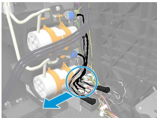
3. Remove the T-20 screw, the T-10 screw, the tubes, and the plastic pieces.
