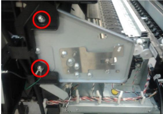
8. Remove the Scan Axis Motor. See [Scan Axis Motor on page 305](#).
