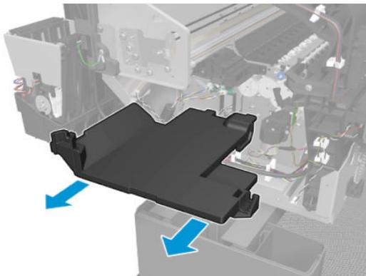
3. Remove the first starwheel rail. See [Customer Self Repair Flyers on page 442](#).
