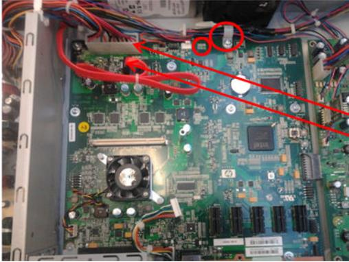
6. Remove four T-8 screws and the L-shaped metal sheet.
