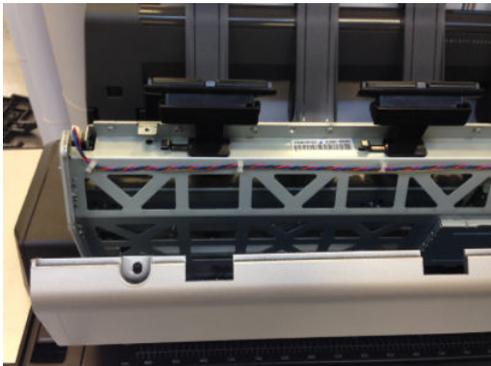
4. Replace the broken batch scanning piece.
