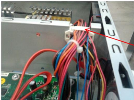
5. Remove grounding cable T-25 screw.
