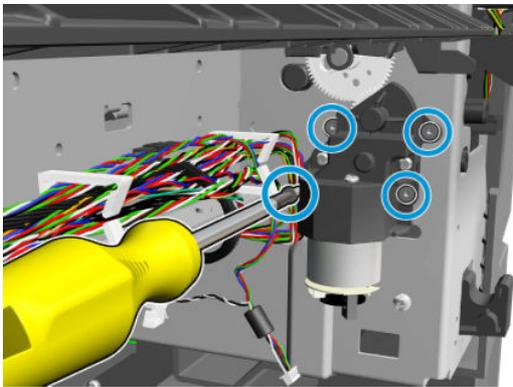
4. Remove the valves motor.
