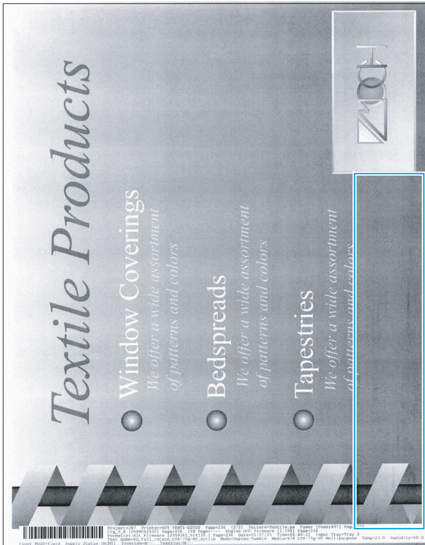
Figure 2-98 Dark streaks (early in toner cartridge life)
